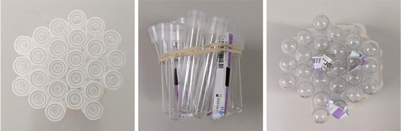
**Figure 4-1:** The figure demonstrated tube arrangement for irradiation with the suggested placement of Radsure stickers.
