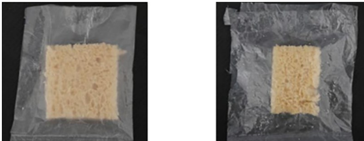
Figure 2.2: Bread packaged in a PHB films.
