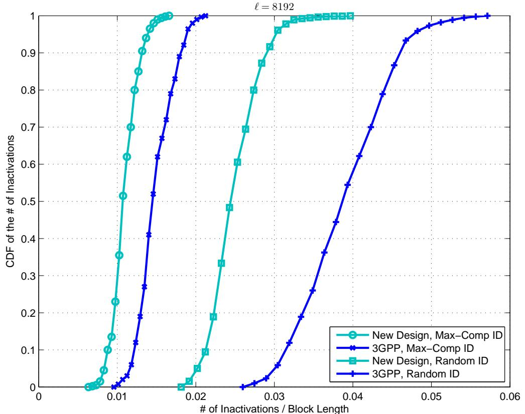
Figure 4.4: CDF of the normalized number of inactivations required for successful decoding,  $\ell = 8192$ . Simulations are performed based for  $10^4$  iterations. In each iteration a complete block of information is transmitted and its overhead is calculated.
