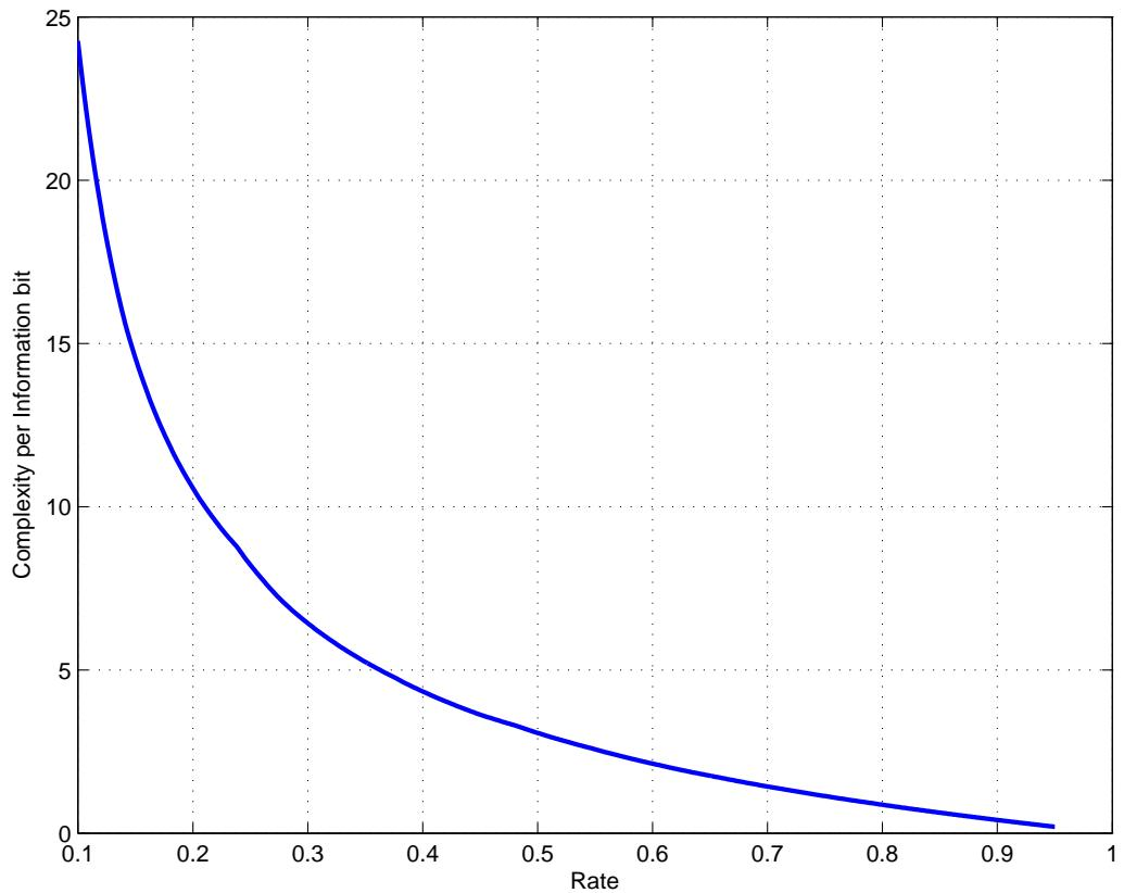
Figure 3.1: Complexity per information bit vs. rate for capacity approaching sequences of LDPC codes designed for the BEC.
