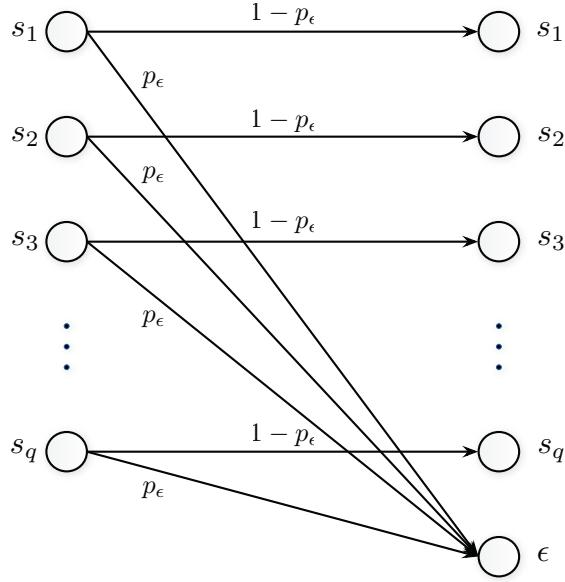
Figure 2.1: A  $q$ -ary erasure channel with an input alphabet of size  $q$ , and an output alphabet of size  $q + 1$ .
