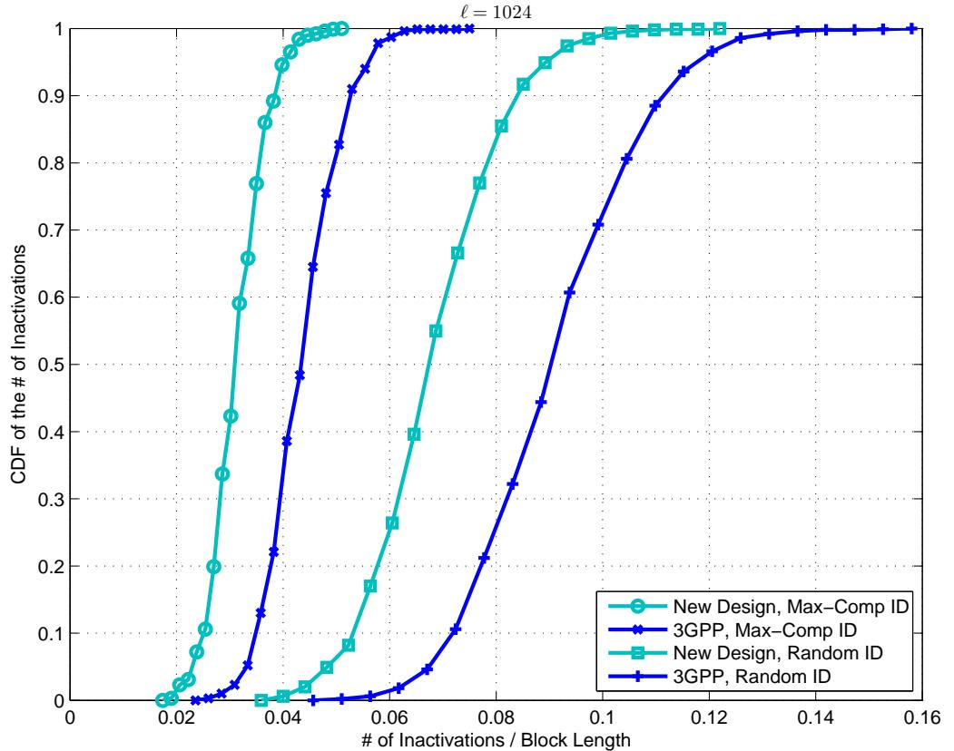
Figure 4.3: CDF of the normalized number of inactivations required for successful decoding,  $\ell = 1024$ . Simulations are performed based for  $10^4$  iterations. In each iteration a complete block of information is transmitted and its overhead is calculated.
