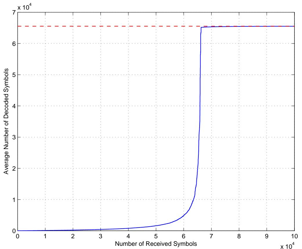
Figure 2.3: Average decoding progress in terms of the number of decoded symbols with respect to the number of received symbols for LT codes for  $k = 65536$ . The dashed red line shows the total number of input symbols.
