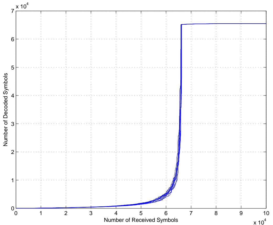
Figure 2.2: Samples of decoding progress in terms of the number of decoded symbols with respect to the number of received symbols for LT codes for  $k = 65536$
