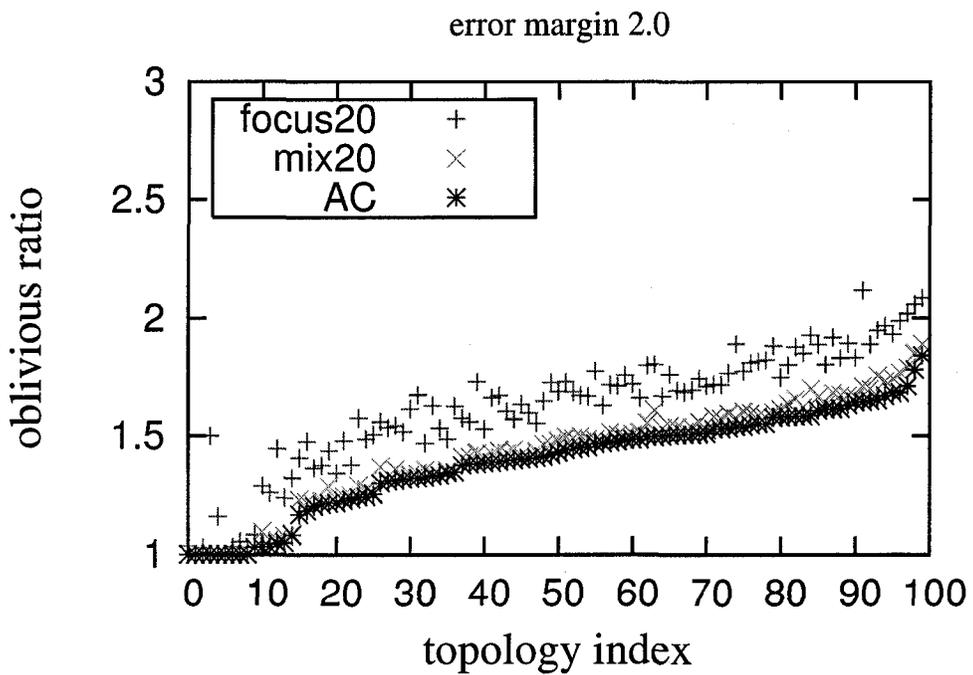
Figure 4.4: Performance of path selection methods on 100 random topologies, comparing with AC.
