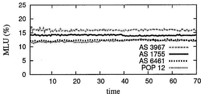
Figure 4.9: Robustness of MORE over failures. At each 10's second, a random link failure occurs, and MORE uses the augmentation strategy for failure restoration over the same set of paths. The TM does not change.
