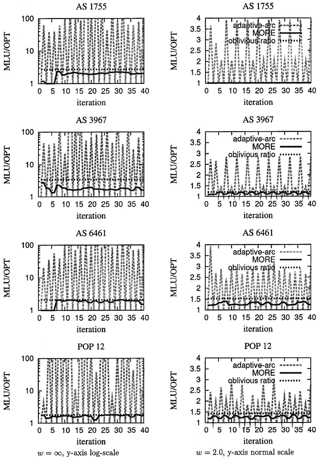
Figure 4.6: Comparing MORE with adaptive-arc under adversary attack. Legend: in figures on right column.
