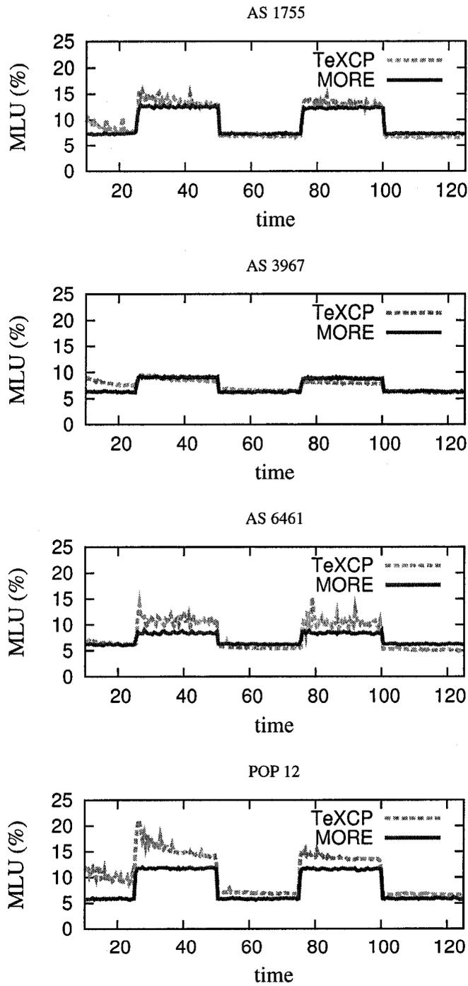
Figure 4.8: TeXCP vs. MORE. During time interval [25,50] and [75,100], extra random traffic is generated.
