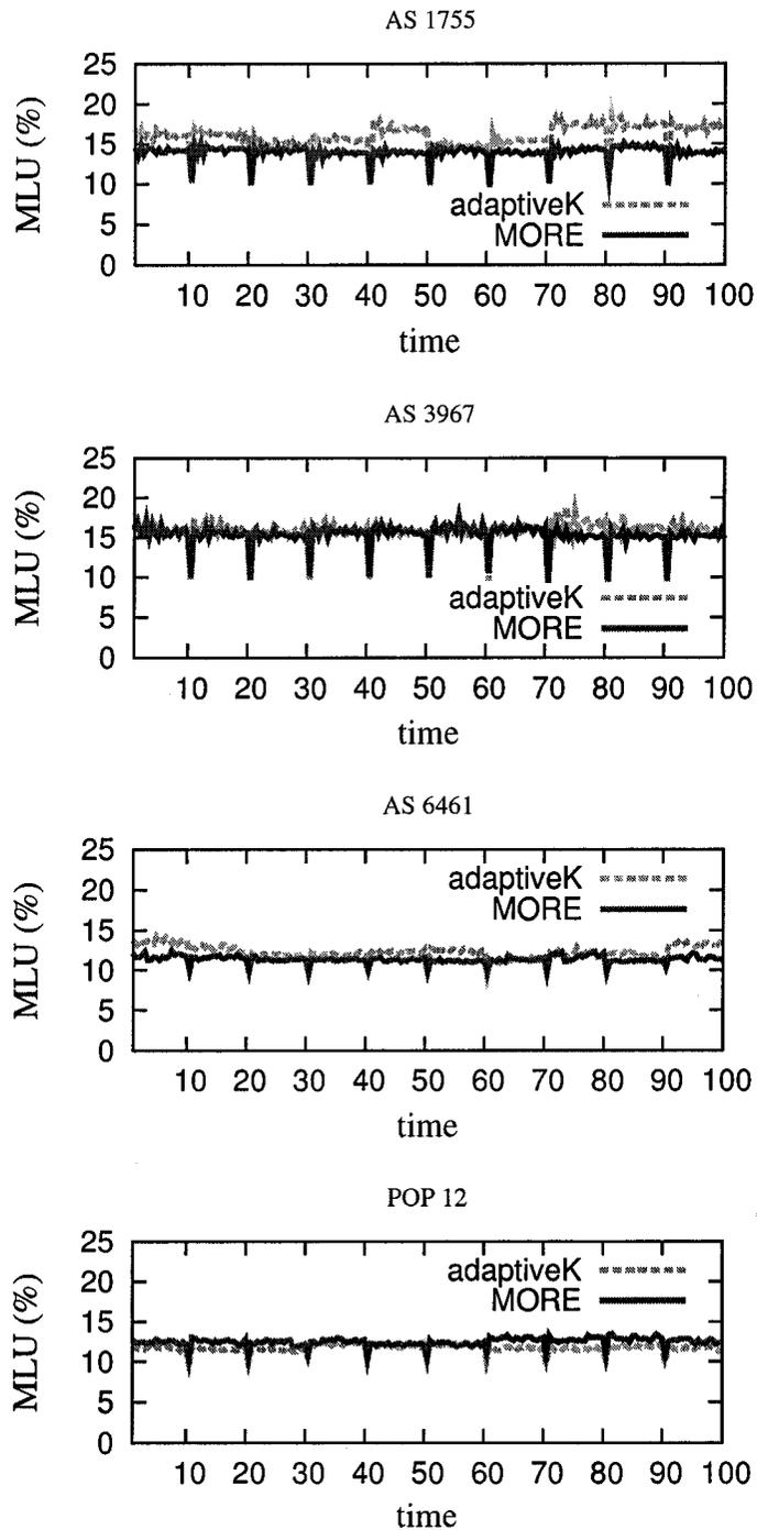
Figure 4.7: Excellent performance of MORE over varying TMs and routings. For each 10 seconds, a random TM is generated, and MORE responds with an optimal multipath oblivious routing over the same set of paths. For adaptiveK, it computes, for each TM, an optimal routing on  $K$ -shortest paths ( $K = 20$ ).
