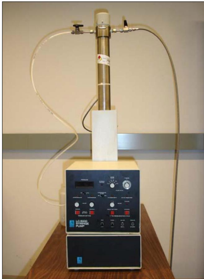
**Fig. 4.3 – Constant Rate Syringe Pump**
