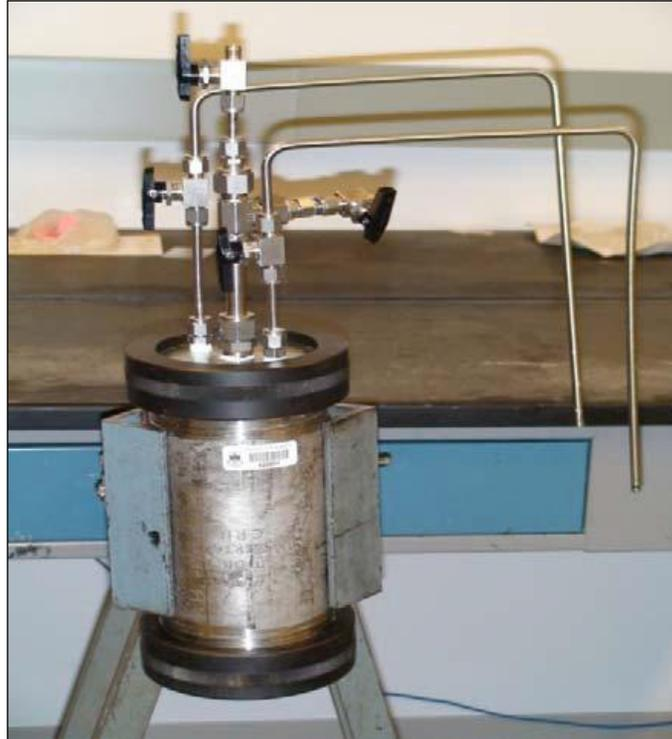
**Fig. 4.2 – Radial Core Holder**
