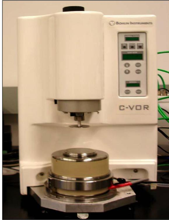
**Fig. 3.3 – Bohlin Rheometer**
