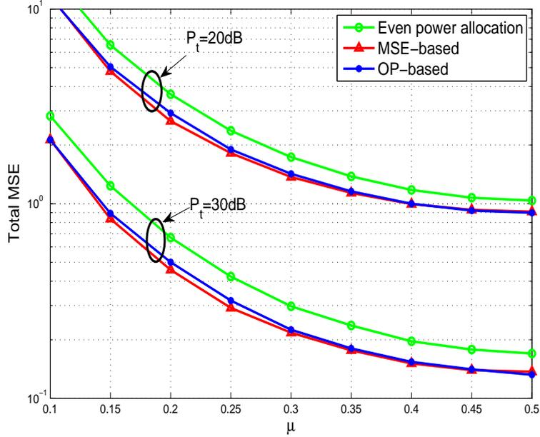
Fig. 4.2: Total MSE for different training power values for two-way single-relay network.
