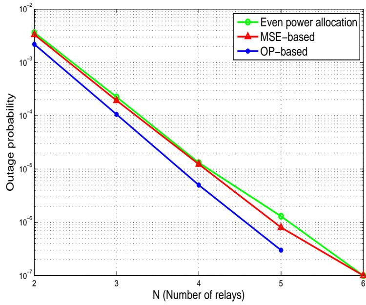
Fig. 3.8: Outage probability for different relay numbers where  $P = 10\text{dB}$  and  $\mu = 0.9$ .
