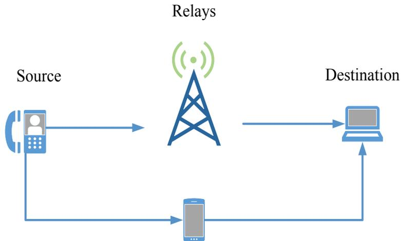
Fig. 1.1: One-way two-relay network.
