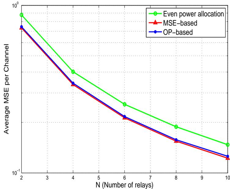
Fig. 3.5: Average MSE per channel for different relay numbers where  $P = 15\text{dB}$  and  $\mu = 0.2$ .
