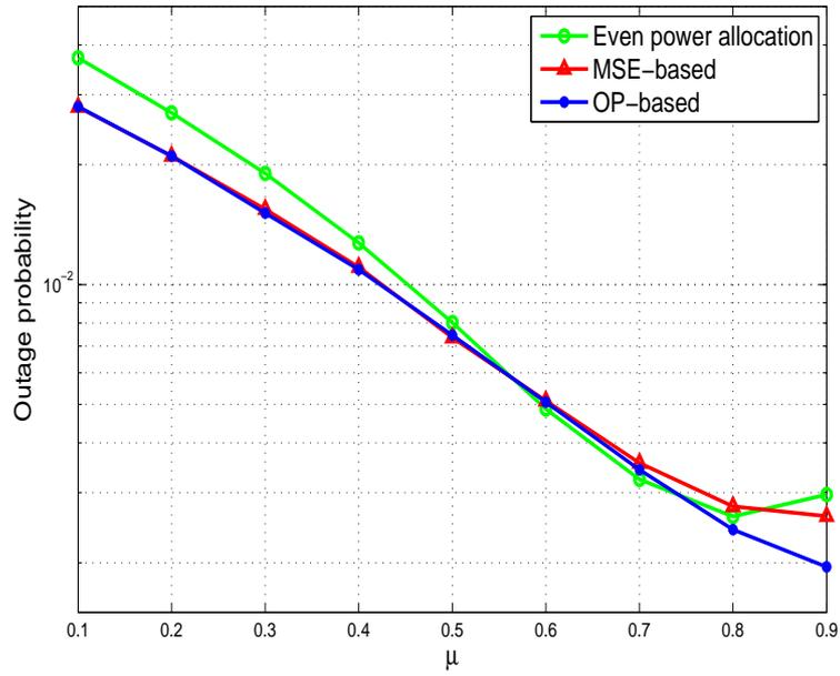
Fig. 2.3: Outage probability for different relay locations for one-way single-relay network where  $P_t = 20\text{dB}$ .
