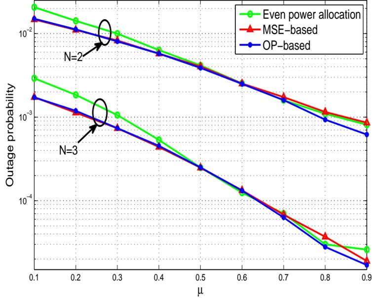
Fig. 3.7: Outage probability for different relay locations for one-way networks with 2 and 3 relays where  $P = 15\text{dB}$ .
