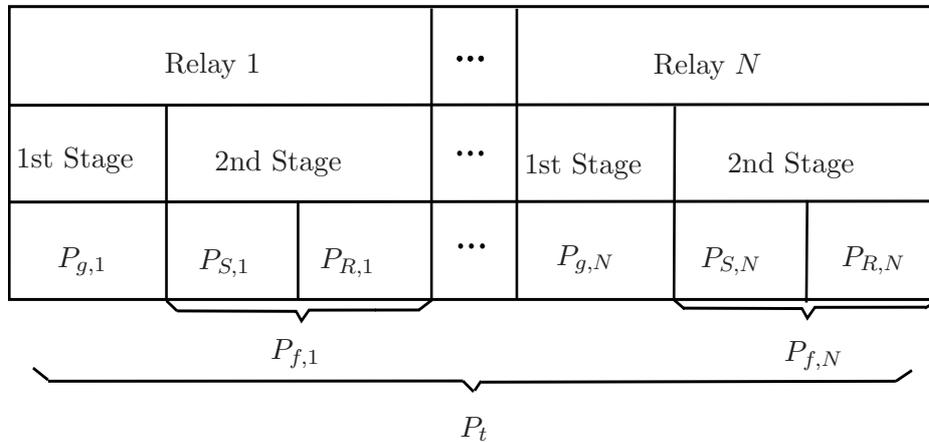
Fig. 3.2: Training scheme and power for one-way multi-relay network.
