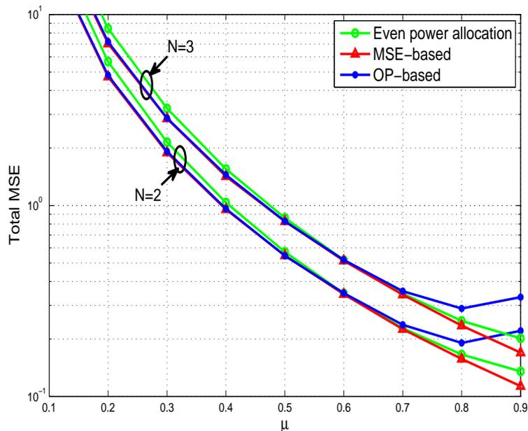
Fig. 3.4: Total MSE for different relay locations for one-way networks with 2 and 3 relays where  $P = 15\text{dB}$ .
