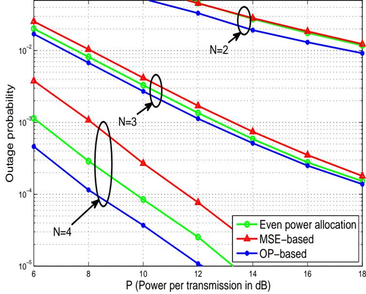
Fig. 3.6: Outage probability for different training power values for one-way networks with 2, 3, and 4 relays.
