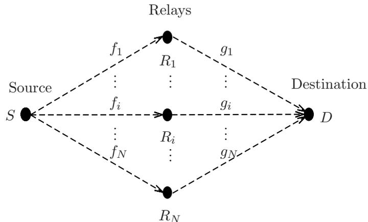
Fig. 3.1: One-way multi-relay network model.
