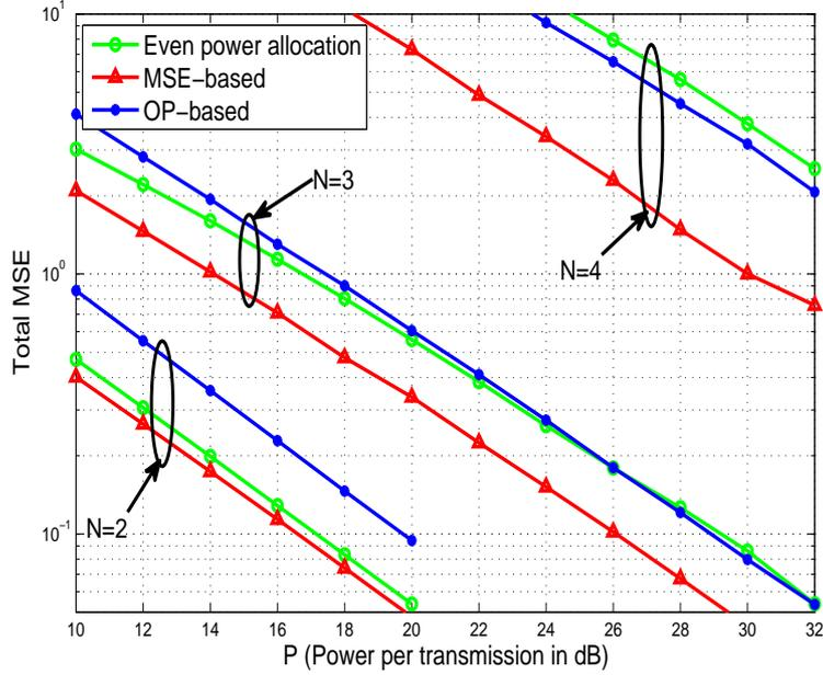
Fig. 3.3: Total MSE for different training power values for one-way networks with 2, 3, and 4 relays.
