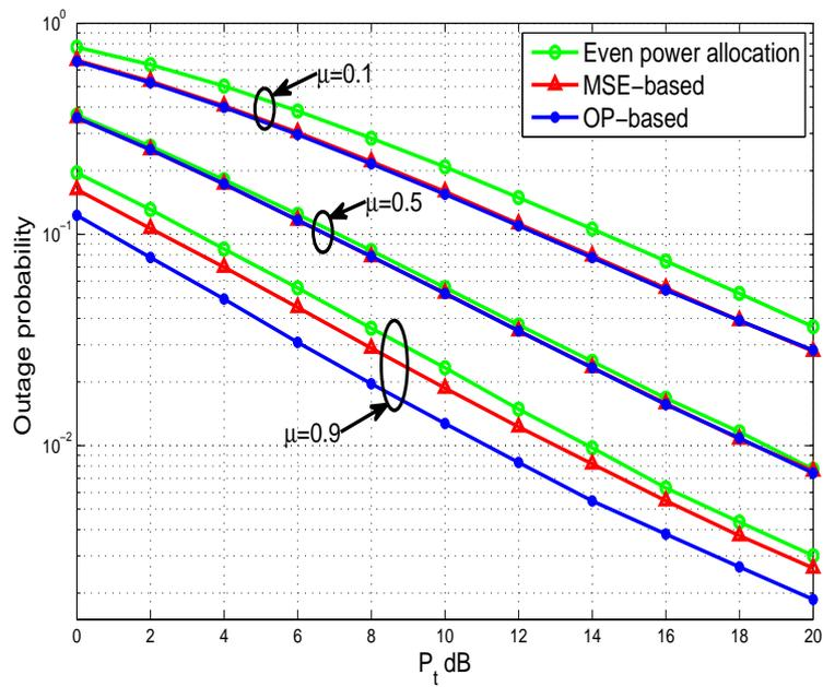
Fig. 2.4: Outage probability for different training power values for one-way single-relay network.
