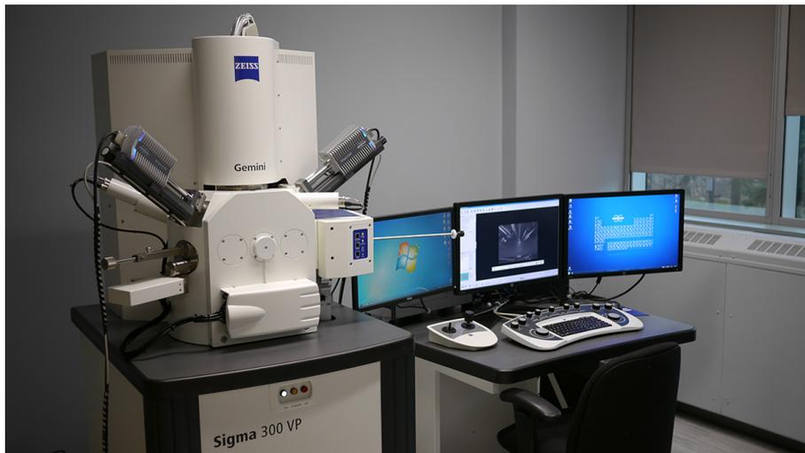
(b) Scanning electron microscope
