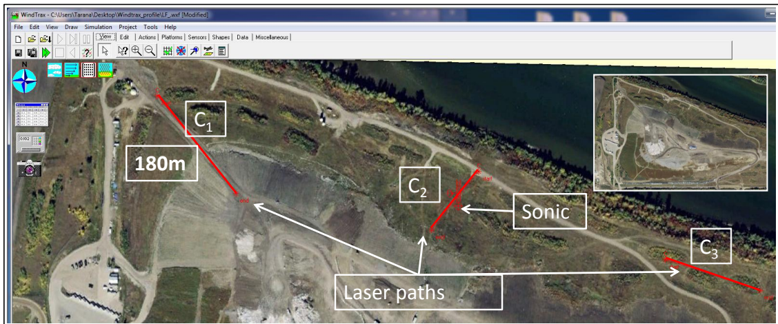
Figure 5.10: Sensor locations in experimental setup for source L_F .
