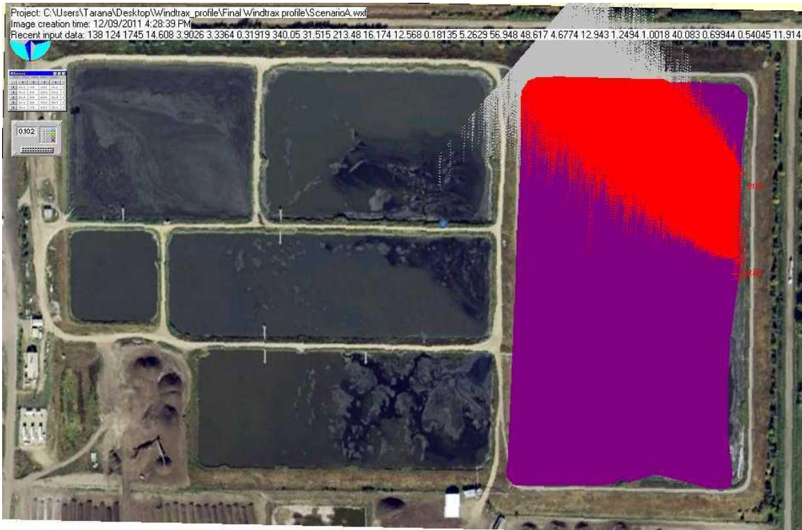
Figure 4.5: Example of WindTrax analysis using configuration A. A single plume of touchdown points is visible, emanating from the downwind laser, and plotted in red when touching down on the source or in grey over land (or over the inactive sources, i.e. other ponds). Background concentration is equated to the concentration signal from the upwind laser, not visible here because obscured by touchdowns.
