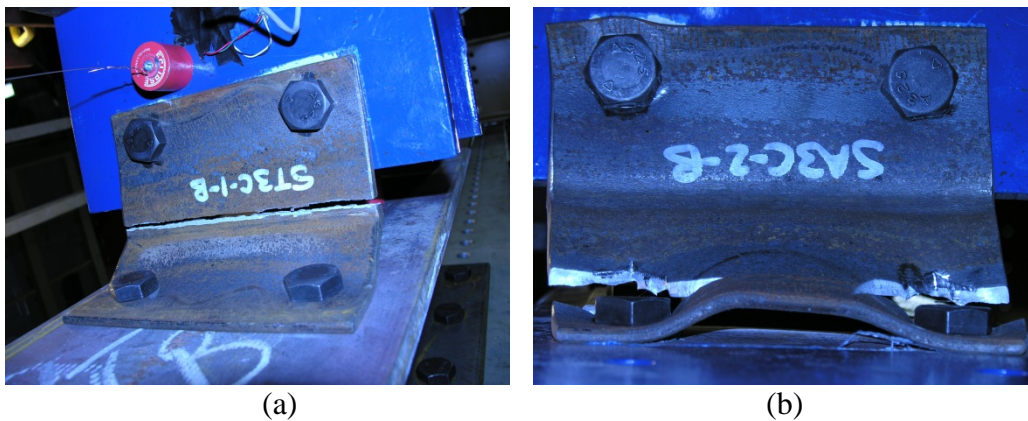
Figure 4.17. Seat angle failure modes (viewed from below): (a) tearing along plastic hinge near angle heel, and (b) tearing along plastic hinges near column bolt line.
