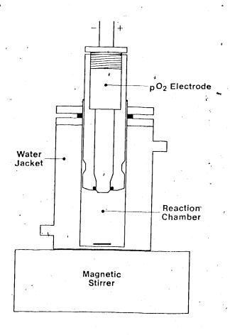
Figure 1.1. Oxygen consumption apparatus. A Clark-type pQ2 electrode is placed inside a plexiglass jacket which fits snugly into a glass reaction chamber. Mitochondria and other additions are introduced to the reaction with a Hamilton syringe. A groove along the length of the electrode jacket permits additions to the medium without allowing the entry of air bubbles. The reaction chamber is surrounded by a water jacket which can regulate the temperature to ±0.1° C.
