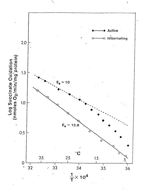
Figure 1.4. Experiment 1.2. Arrhenius plot of Ca2+-stimulated succinate oxidation in liver mitochondria from active and hibernating Columbian ground squirrels. Ea's are the mean of six individuals.
