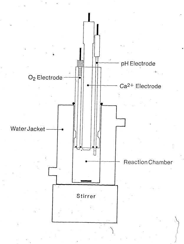
Figure 2.1. Electrode assembly for the simultaneous measurement of H- efflux,  $Ca^{2+}$  uptake and oxygen consumption.
