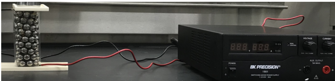
Figure 5.1: Experimental setup of the electrically heated steel particles packed in a glass cylinder: a - schematic representation of the experiment; b - photo of experimental setup.
