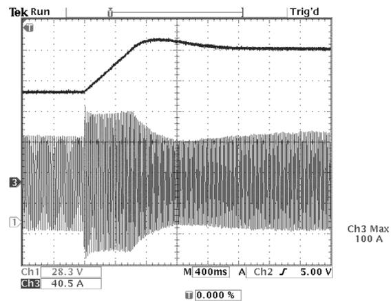
Fig. 14. Traces of the transient response: machine speed and line current.
