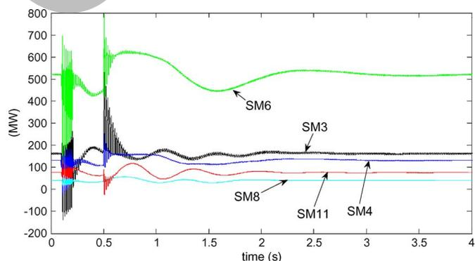
Fig. 8. Synchronous machines, 3-phase powers.
