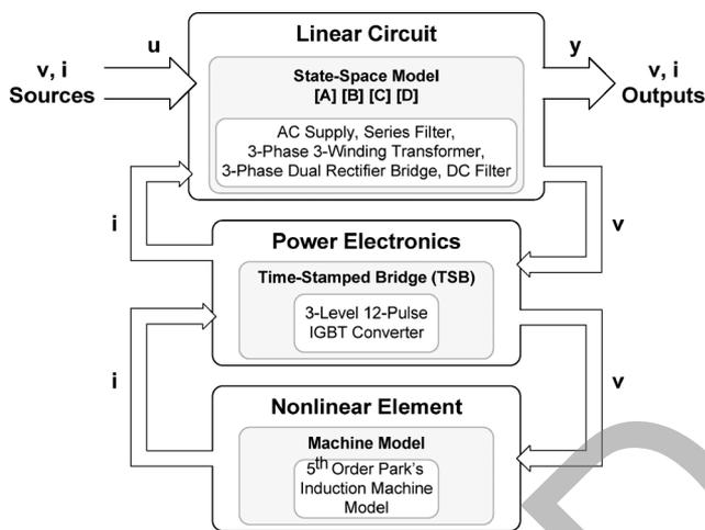
Fig. 11. System model separation for real-time simulation.
