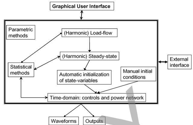
Fig. 1. Ultimate building blocks of an EMT-type simulation tool.
