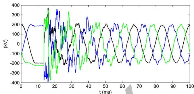
Fig. 6. Transmission line overvoltages at receiving end phases.
