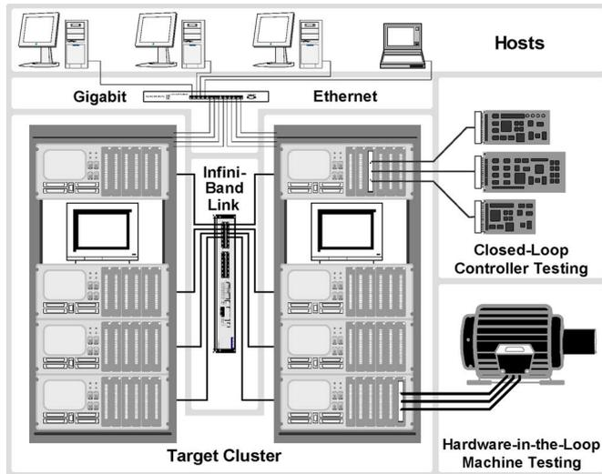
Fig. 9. PC-cluster based real-time digital simulator.
