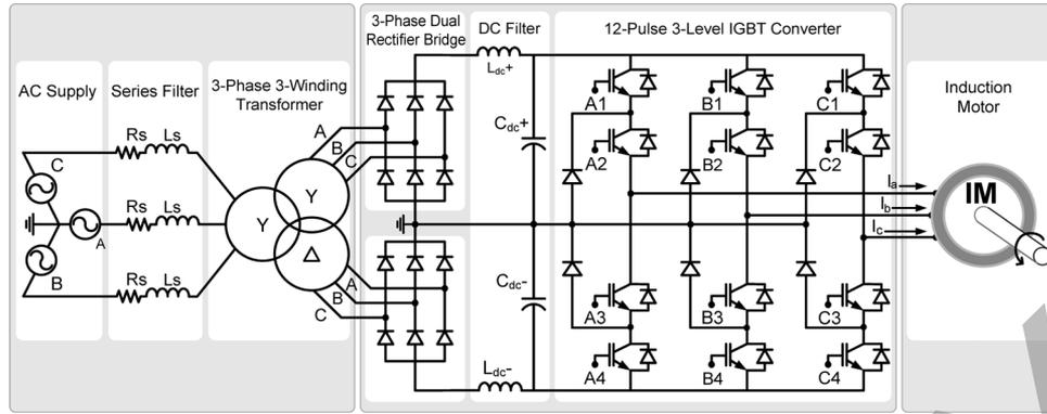
Fig. 10. Vector-controlled variable-speed ac drive.
