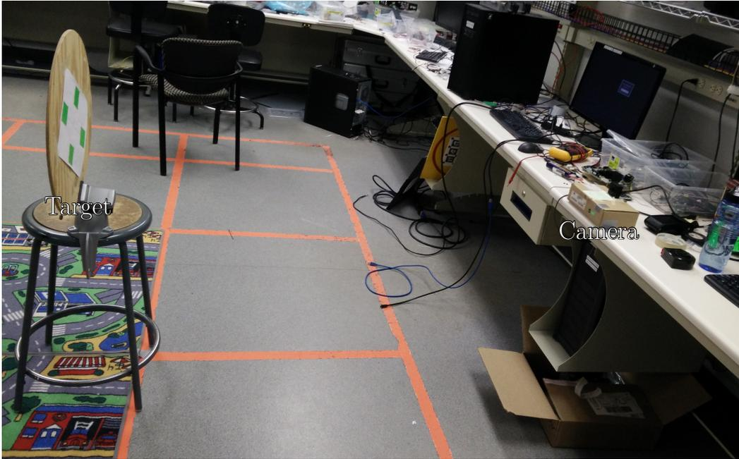
Figure 3.4: Image moment reference setup with relocatable target in front of the fixed camera
