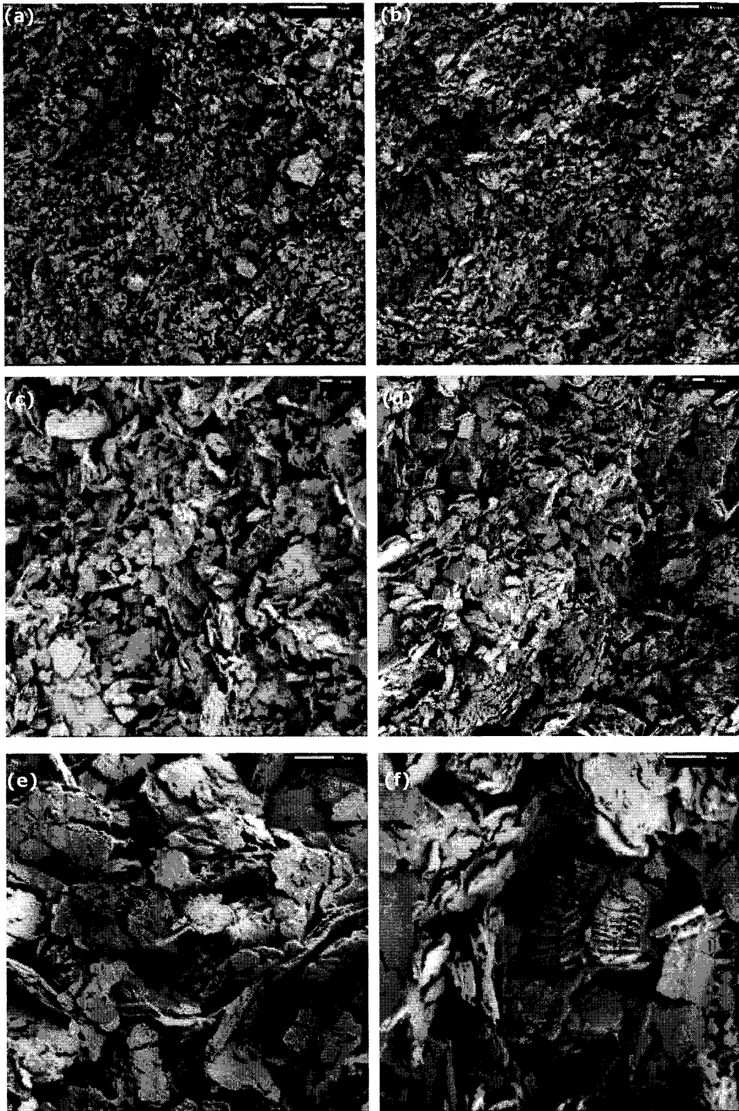
Figure E.12. Photomicrographs of oven-dried kaolin-cement at w=100\% , A_c=5\% and T_c = 112 days. (a) & (b) M \approx 750X ; (c) & (d) M \approx 2250X ; (e) & (f) M \approx 7500X .
