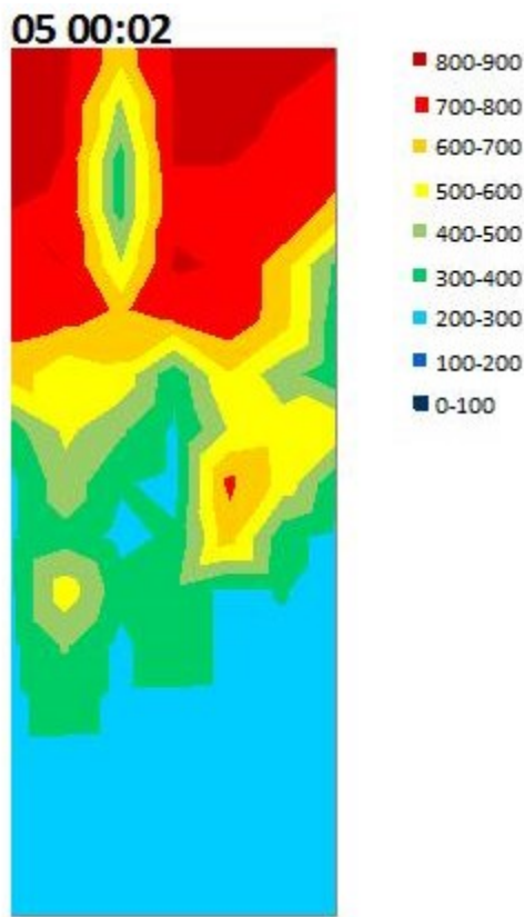
Figure 2.6 Coke Drum Shell Temperatures in [ °F ]
