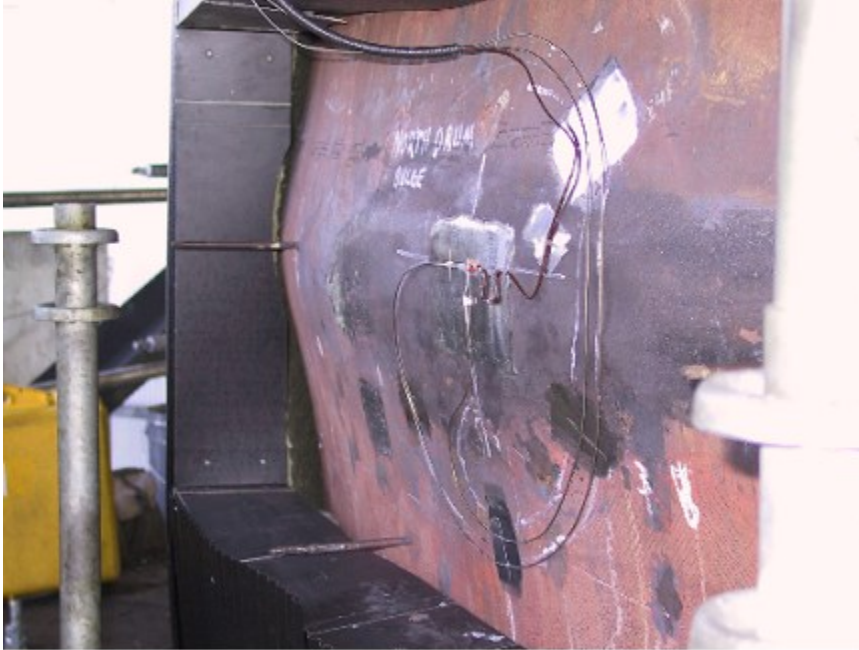
Figure 6.13 Photograph of a Drum Bulge
