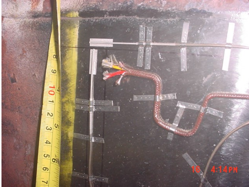
Figure 3.6 Strain Gauges with Independent Thermocouple
