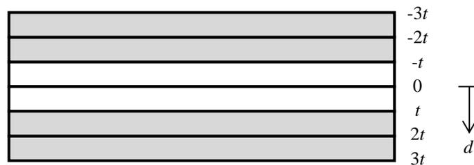
**Fig. (5).** Schematic of three braids, each consisting of two layers.
