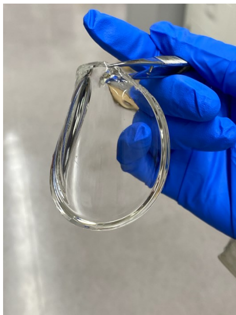
Figure S.1. Photograph of as-prepared H-0.5-0.5 hydrogel showing high transparency
