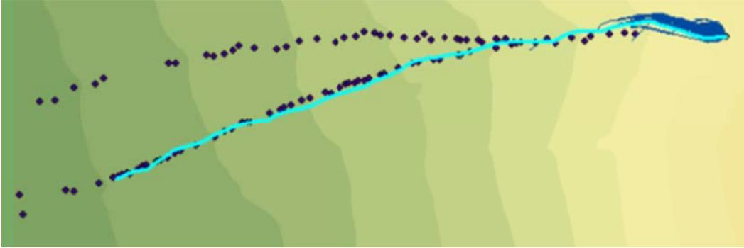
Figure C.78: Rockfall Simulation:  $R_n = 0.15$   $R_t = 0.8$ ; Slope Angle  $55^\circ$ ; Drop Height 50m
