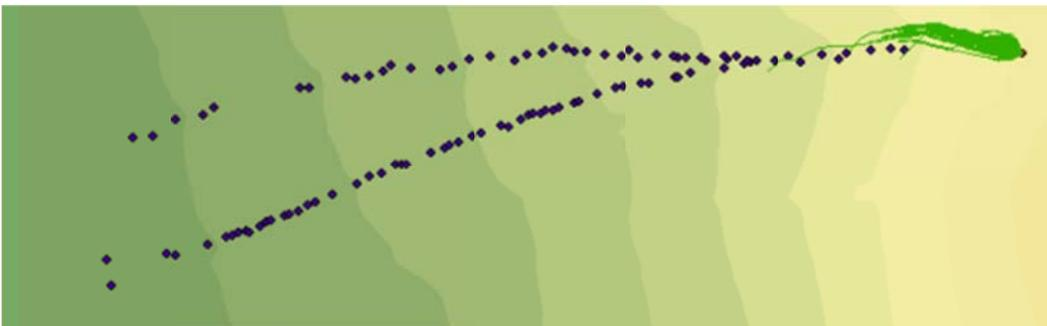
Figure C.42: Rockfall Simulation:  $R_n = 0.27$   $R_t = 0.77$ ; Slope Angle  $55^\circ$ ; Drop Height 50m
