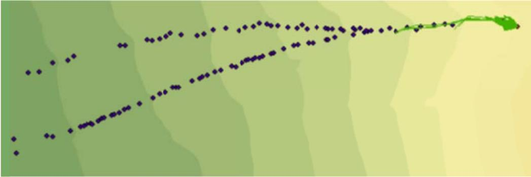
Figure C.90: Rockfall Simulation:  $R_n = 0.3$   $R_t = 0.5$ ; Slope Angle  $65^\circ$ ; Drop Height 50m
