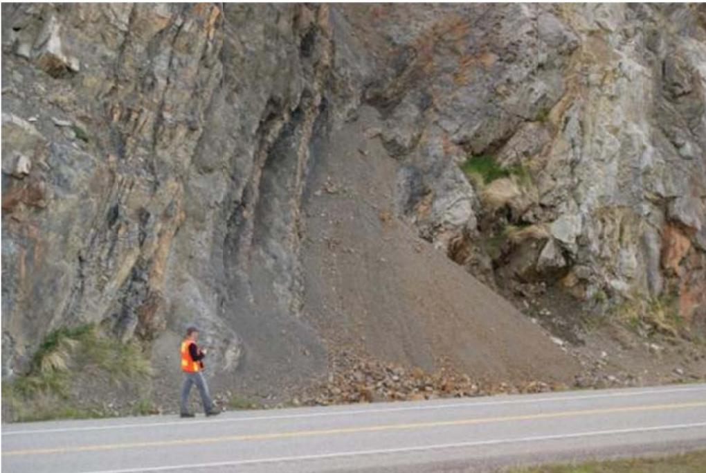
**Figure 3.14: Talus Cone Formed Under Erosion Gully at Fir Creek Site (photo by James Russell)**
