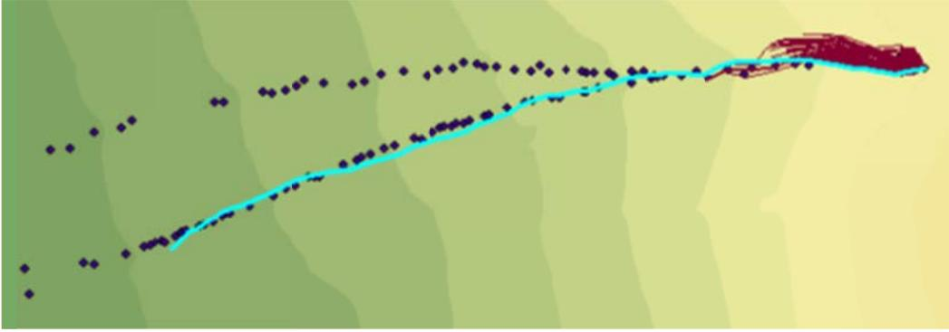
Figure C.89: Rockfall Simulation:  $R_n = 0.3$   $R_t = 0.5$ ; Slope Angle  $55^\circ$ ; Drop Height 70m
