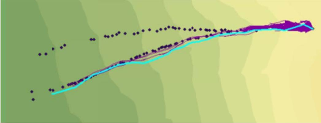
Figure C.6: Rockfall Simulation:  $R_n = 0.33$   $R_t = 0.87$ ; Slope Angle  $45^\circ$ ; Drop Height 50m
