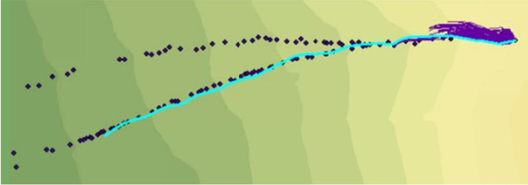
Figure C.71: Rockfall Simulation:  $R_n = 0.15$   $R_t = 0.5$ ; Slope Angle  $55^\circ$ ; Drop Height 70m
