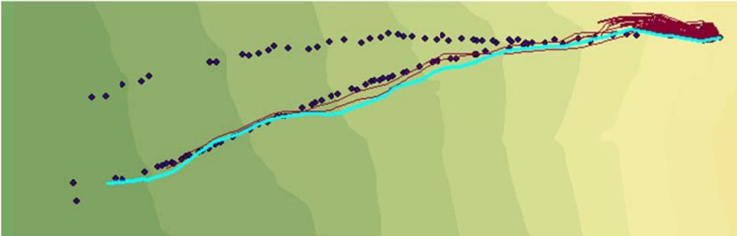
**Figure 5.25: Typical COR Value Simulation ( $55^\circ$  Slope Angle and 70m Drop Height)**
