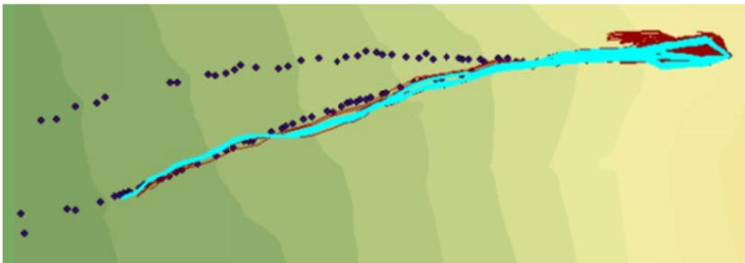
**Figure C.77: Rockfall Simulation:  $R_n = 0.15$   $R_t = 0.8$ ; Slope Angle  $45^\circ$ ; Drop Height 70m**
