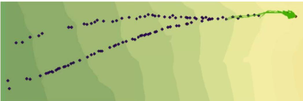
Figure C.63: Rockfall Simulation:  $R_n = 0.3$   $R_t = 0.77$ ; Slope Angle  $65^\circ$ ; Drop Height 50m
