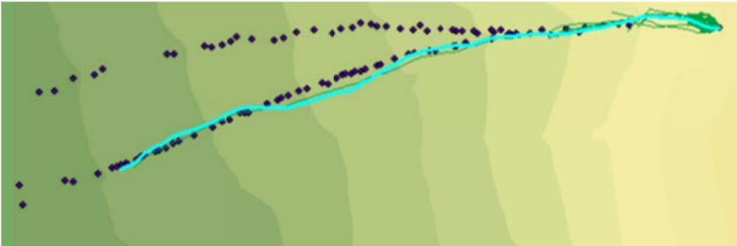
Figure C.55: Rockfall Simulation:  $R_n = 0.27$   $R_t = 0.8$ ; Slope Angle  $65^\circ$ ; Drop Height 60m
