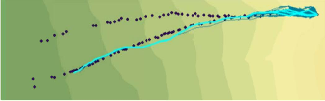
Figure C.39: Rockfall Simulation:  $R_n = 0.27$   $R_t = 0.77$ ; Slope Angle  $45^\circ$ ; Drop Height 50m
