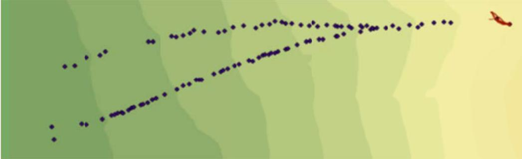
Figure C.23: Rockfall Simulation:  $R_n = 0.33$   $R_t = 0.87$ ; Slope Angle  $75^\circ$ ; Drop Height 10m
