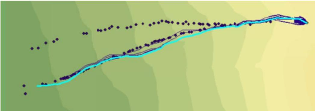
Figure C.38: Rockfall Simulation:  $R_n = 0.3$   $R_t = 0.8$ ; Slope Angle  $65^\circ$ ; Drop Height 70m
