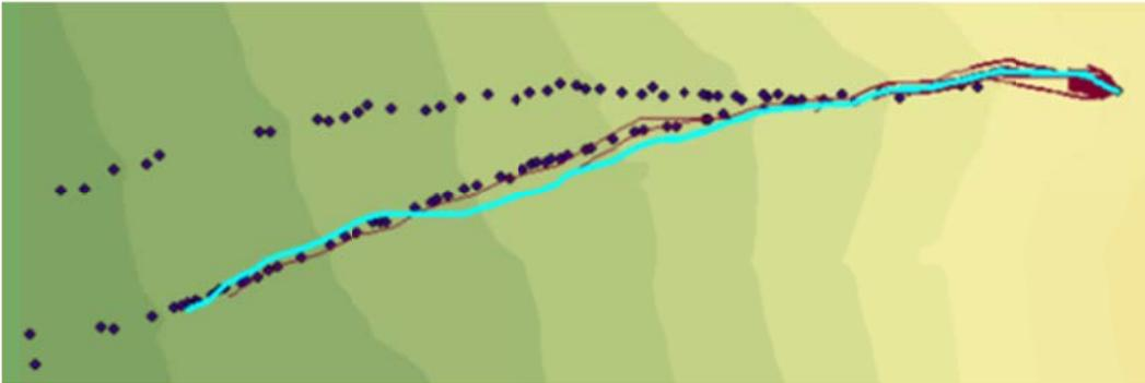
**Figure C.83: Rockfall Simulation:  $R_n = 0.15$   $R_t = 0.8$ ; Slope Angle  $65^\circ$ ; Drop Height 70m**
