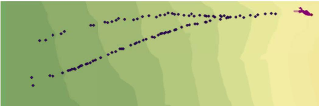
Figure C.25: Rockfall Simulation:  $R_n = 0.33$   $R_t = 0.87$ ; Slope Angle  $75^\circ$ ; Drop Height 30m
