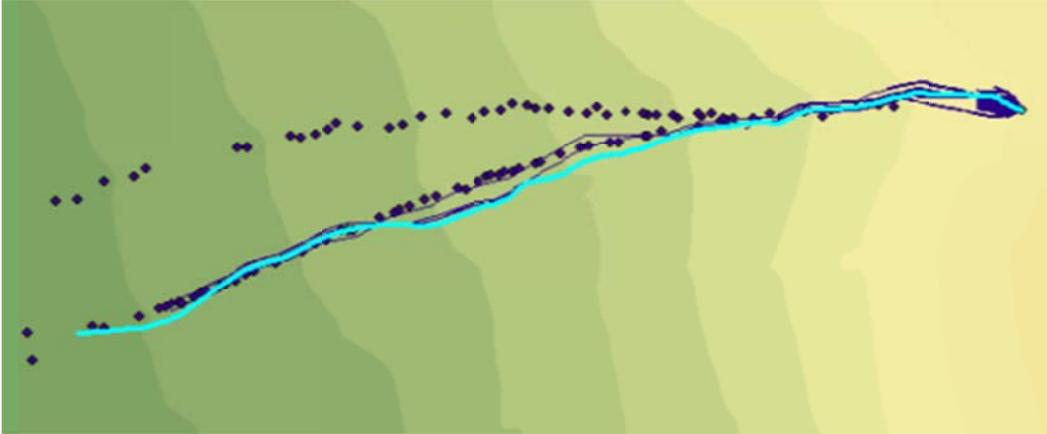
**Figure C.47: Rockfall Simulation:  $R_n = 0.27$   $R_t = 0.77$ ; Slope Angle  $65^\circ$ ; Drop Height 70m**
