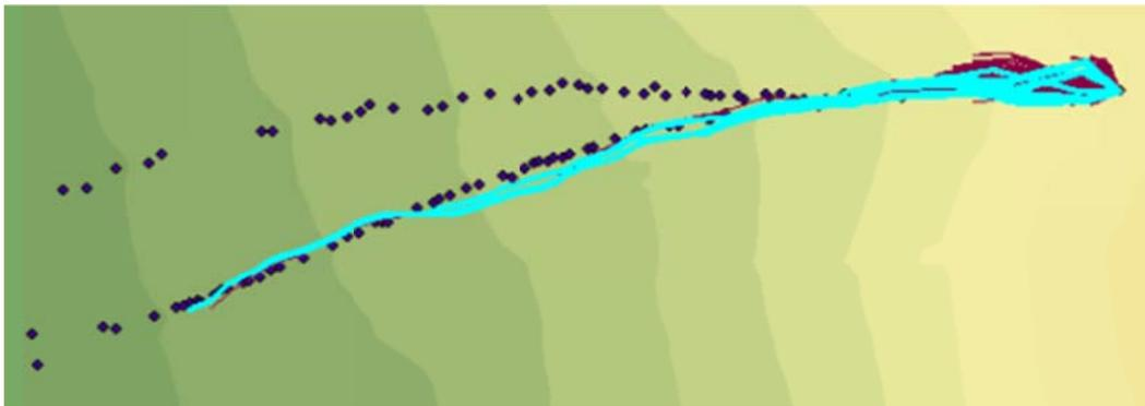
**Figure C.76: Rockfall Simulation:  $R_n = 0.15$   $R_t = 0.8$ ; Slope Angle  $45^\circ$ ; Drop Height 60m**
