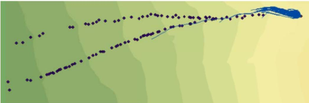
Figure C.69: Rockfall Simulation:  $R_n = 0.15$   $R_t = 0.5$ ; Slope Angle  $55^\circ$ ; Drop Height 50m
