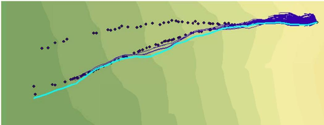
**Figure 5.22: Rockfall Energy Calibration Simulation: Angle 45° Drop Height 60m**
