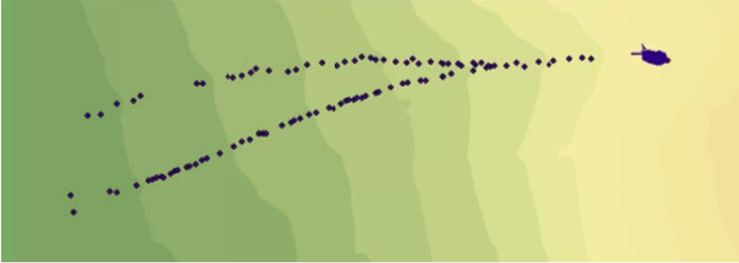
Figure C.2: Rockfall Simulation:  $R_n = 0.33$   $R_t = 0.87$ ; Slope Angle  $45^\circ$ ; Drop Height 10m
