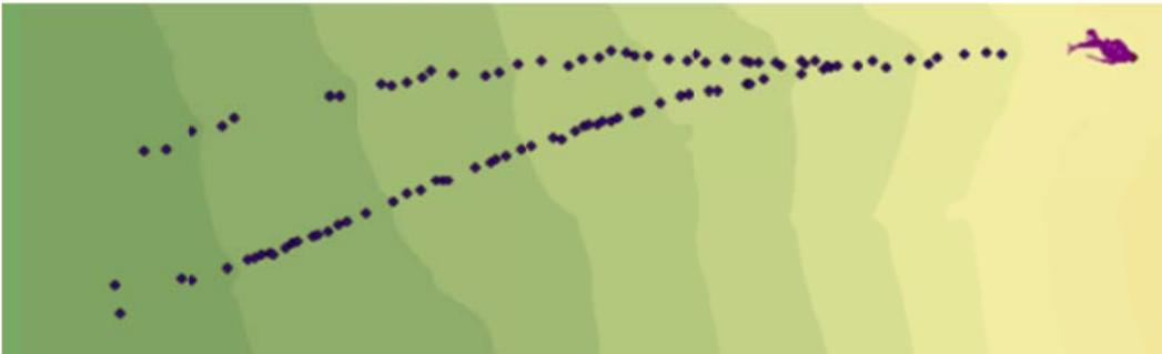
Figure C.17: Rockfall Simulation:  $R_n = 0.33$   $R_t = 0.87$ ; Slope Angle  $65^\circ$ ; Drop Height 20m
