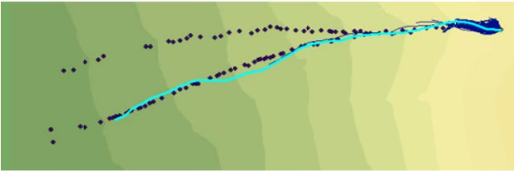
Figure C.4: Rockfall Simulation:  $R_n = 0.33$   $R_t = 0.87$ ; Slope Angle  $45^\circ$ ; Drop Height 30m
