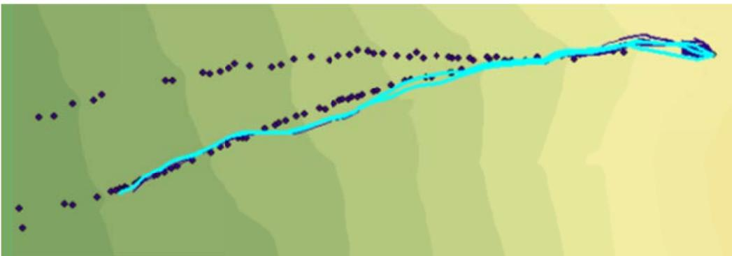
Figure C.92: Rockfall Simulation:  $R_n = 0.3$   $R_t = 0.5$ ; Slope Angle  $65^\circ$ ; Drop Height 70m
