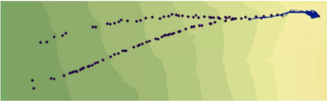
Figure C.20: Rockfall Simulation:  $R_n = 0.33$   $R_t = 0.87$ ; Slope Angle  $65^\circ$ ; Drop Height 50m
