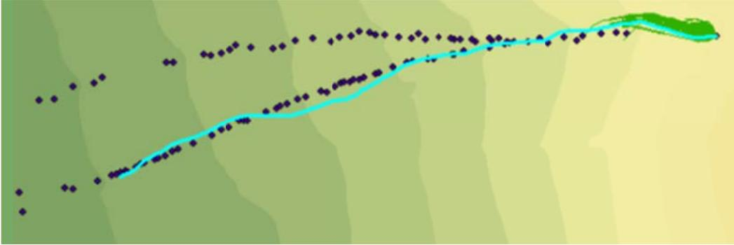
Figure C.60: Rockfall Simulation:  $R_n = 0.3$   $R_t = 0.77$ ; Slope Angle  $55^\circ$ ; Drop Height 50m
