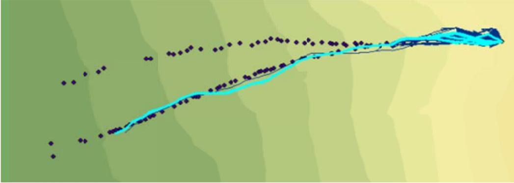
**Figure C.30: Rockfall Simulation:  $R_n = 0.3$   $R_t = 0.8$ ; Slope Angle  $45^\circ$ ; Drop Height 50m**
