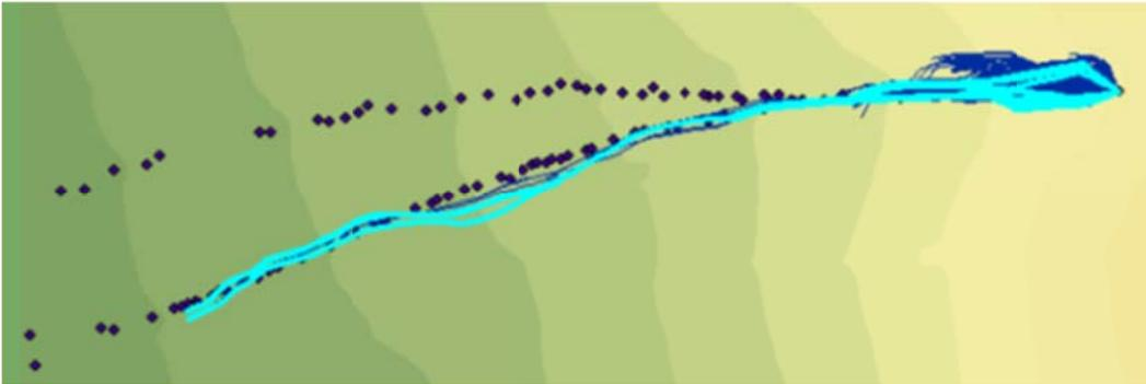
Figure C.86: Rockfall Simulation:  $R_n = 0.3$   $R_t = 0.5$ ; Slope Angle  $45^\circ$ ; Drop Height 70m
