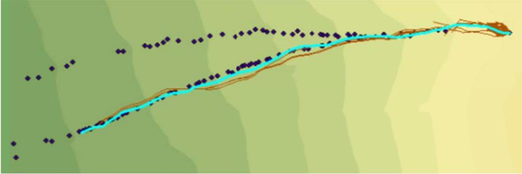
**Figure C.82: Rockfall Simulation:  $R_n = 0.15$   $R_t = 0.8$ ; Slope Angle  $65^\circ$ ; Drop Height 60m**
