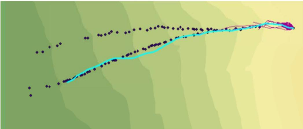
Figure C.21: Rockfall Simulation:  $R_n = 0.33$   $R_t = 0.87$ ; Slope Angle  $65^\circ$ ; Drop Height 60m
