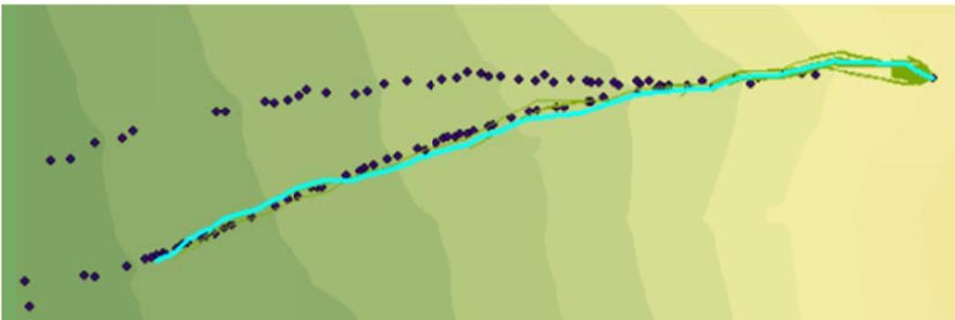
Figure C.74: Rockfall Simulation:  $R_n = 0.15$   $R_t = 0.5$ ; Slope Angle  $65^\circ$ ; Drop Height 70m
