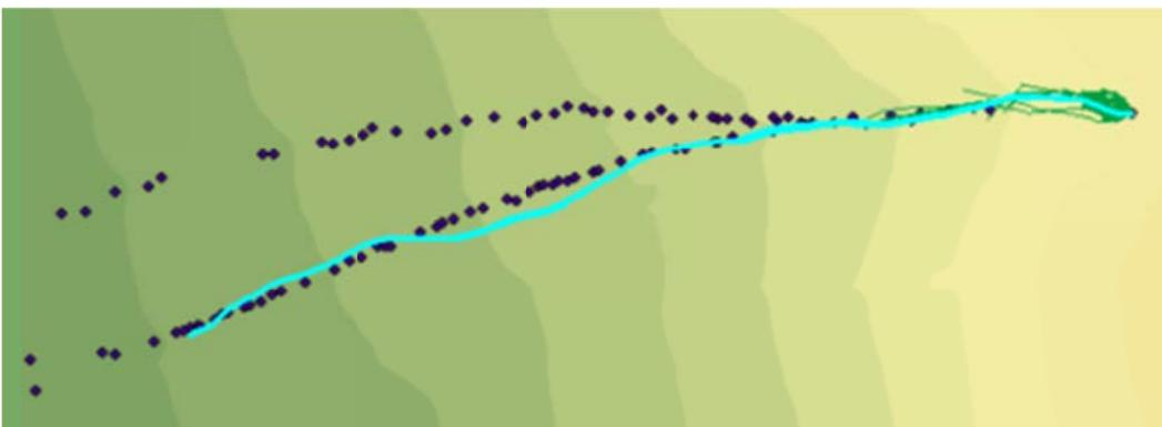
Figure C.46: Rockfall Simulation:  $R_n = 0.27$   $R_t = 0.77$ ; Slope Angle  $65^\circ$ ; Drop Height 60m
