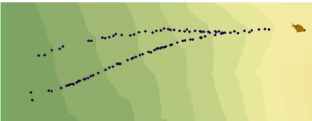
Figure C.19: Rockfall Simulation:  $R_n = 0.33$   $R_t = 0.87$ ; Slope Angle  $65^\circ$ ; Drop Height 40m
