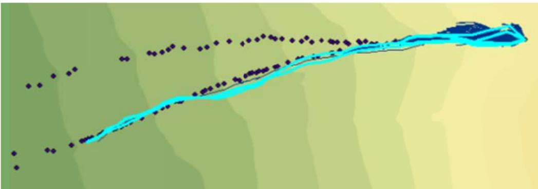
**Figure C.49: Rockfall Simulation:  $R_n = 0.27$   $R_t = 0.8$ ; Slope Angle  $45^\circ$ ; Drop Height 60m**
