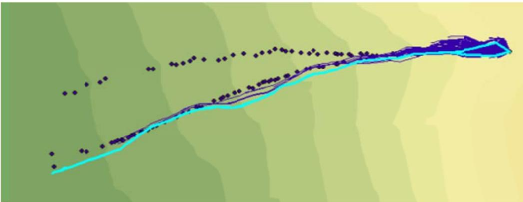
Figure C.7: Rockfall Simulation:  $R_n = 0.33$   $R_t = 0.87$ ; Slope Angle  $45^\circ$ ; Drop Height 60m
