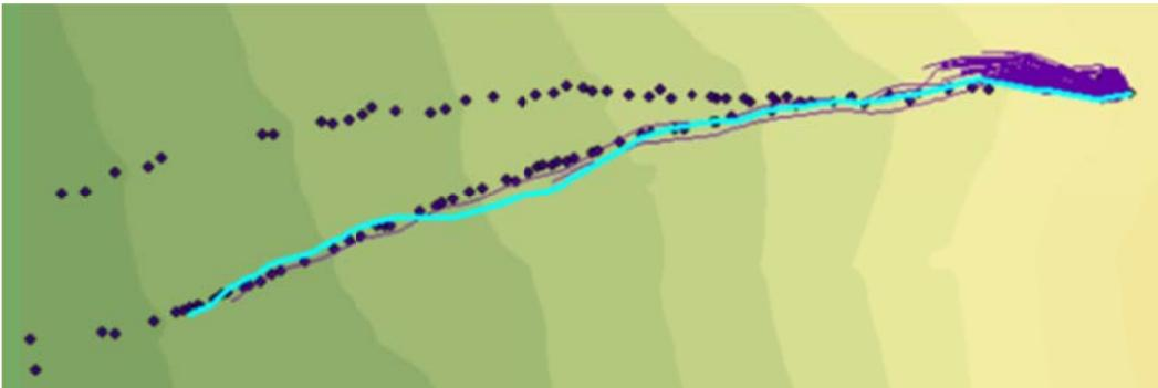
Figure C.80: Rockfall Simulation:  $R_n = 0.15$   $R_t = 0.8$ ; Slope Angle  $55^\circ$ ; Drop Height 70m
