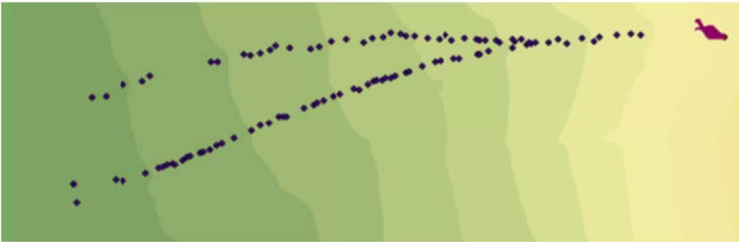
**Figure C.27: Rockfall Simulation:  $R_n = 0.33$   $R_t = 0.87$ ; Slope Angle  $75^\circ$ ; Drop Height 50m**
