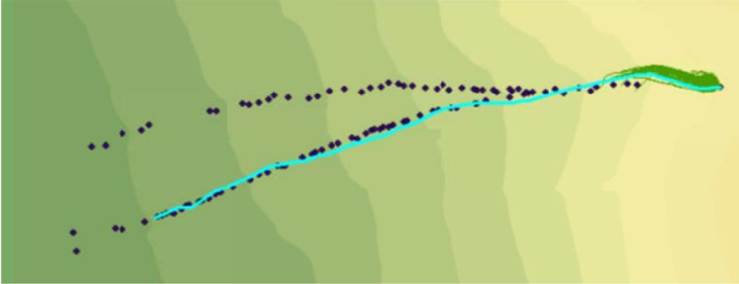
Figure C.13: Rockfall Simulation:  $R_n = 0.33$   $R_t = 0.87$ ; Slope Angle  $55^\circ$ ; Drop Height 50m
