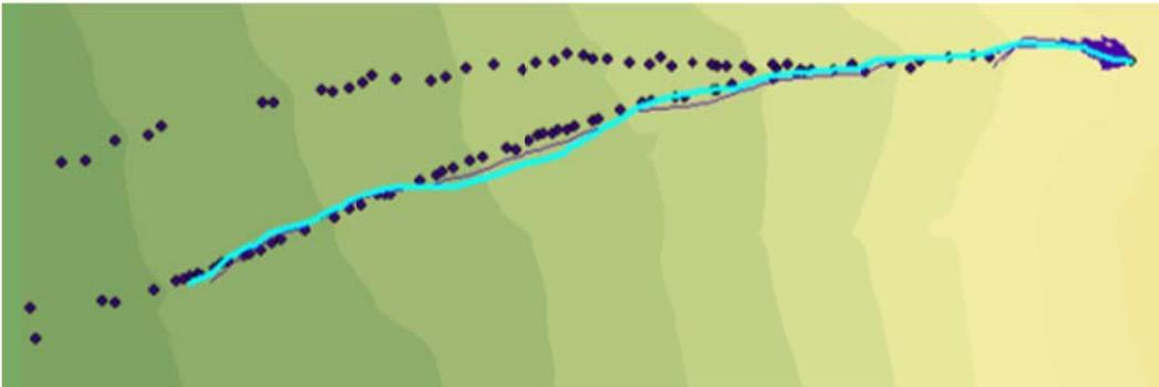
Figure C.72: Rockfall Simulation:  $R_n = 0.15$   $R_t = 0.5$ ; Slope Angle  $65^\circ$ ; Drop Height 50m
