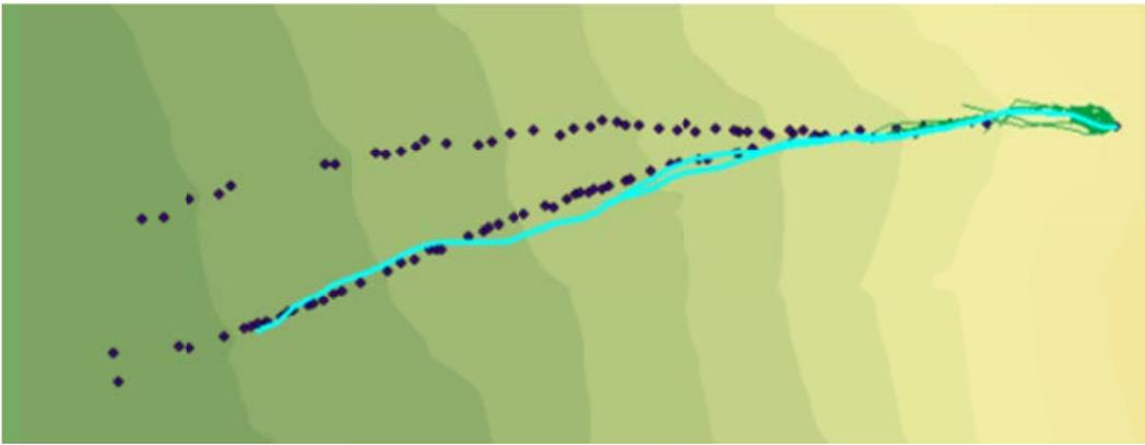
Figure C.37: Rockfall Simulation:  $R_n = 0.3$   $R_t = 0.8$ ; Slope Angle  $65^\circ$ ; Drop Height 60m
