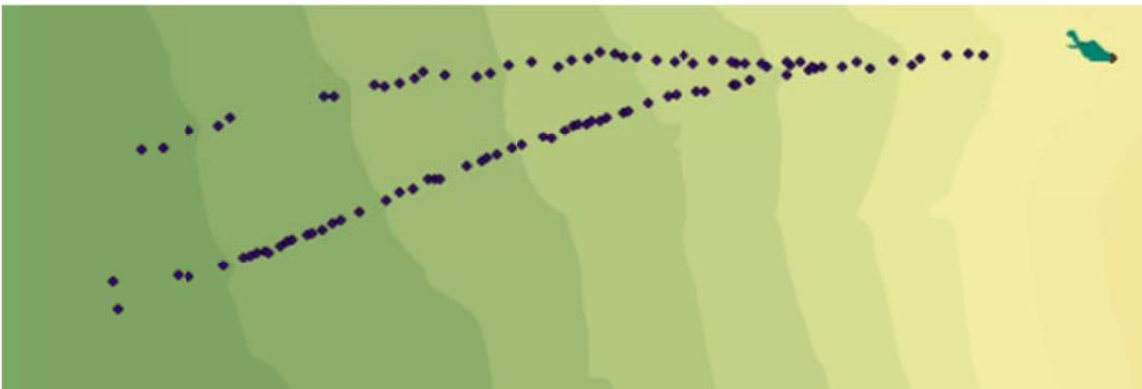
Figure C.26: Rockfall Simulation:  $R_n = 0.33$   $R_t = 0.87$ ; Slope Angle  $75^\circ$ ; Drop Height 40m
