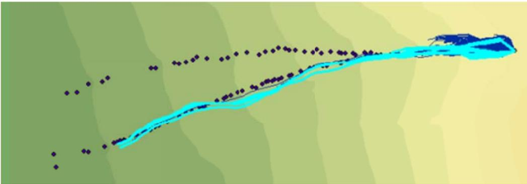
Figure C.41: Rockfall Simulation:  $R_n = 0.27$   $R_t = 0.77$ ; Slope Angle  $45^\circ$ ; Drop Height 70m
