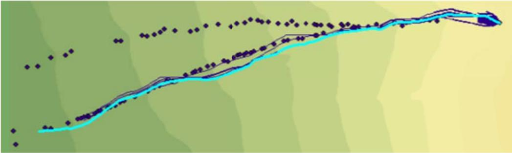
**Figure C.65: Rockfall Simulation:  $R_n = 0.3$   $R_t = 0.77$ ; Slope Angle  $65^\circ$ ; Drop Height 70m**
