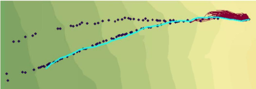
**Figure 5.39: Typical Normal Greatly Reduced Tangential COR Value Simulation (55° Slope Angle and 70m Drop Height)**
