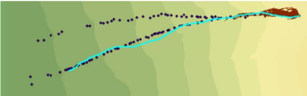
Figure C.5: Rockfall Simulation:  $R_n = 0.33$   $R_t = 0.87$ ; Slope Angle  $45^\circ$ ; Drop Height 40m
