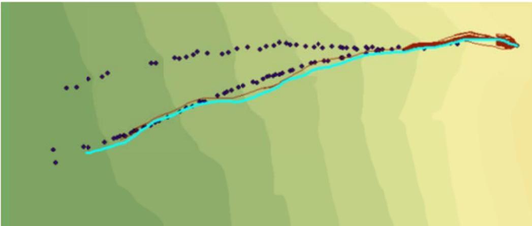
Figure C.22: Rockfall Simulation:  $R_n = 0.33$   $R_t = 0.87$ ; Slope Angle  $65^\circ$ ; Drop Height 70m
