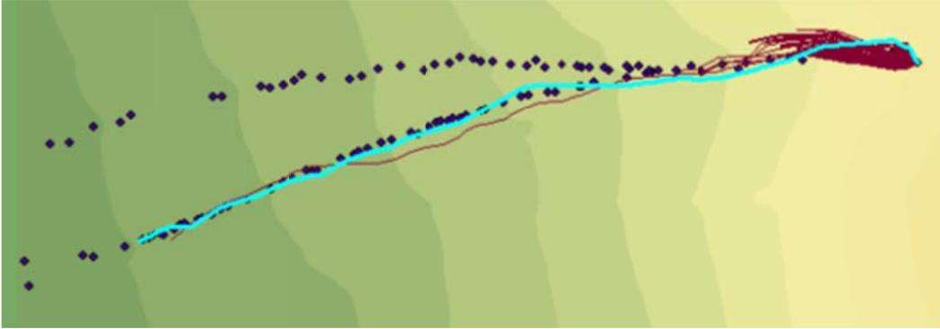
Figure 5.31: Reduced Normal Typical Tangential COR Value Simulation (55° Slope Angle and 70m Drop Height)
