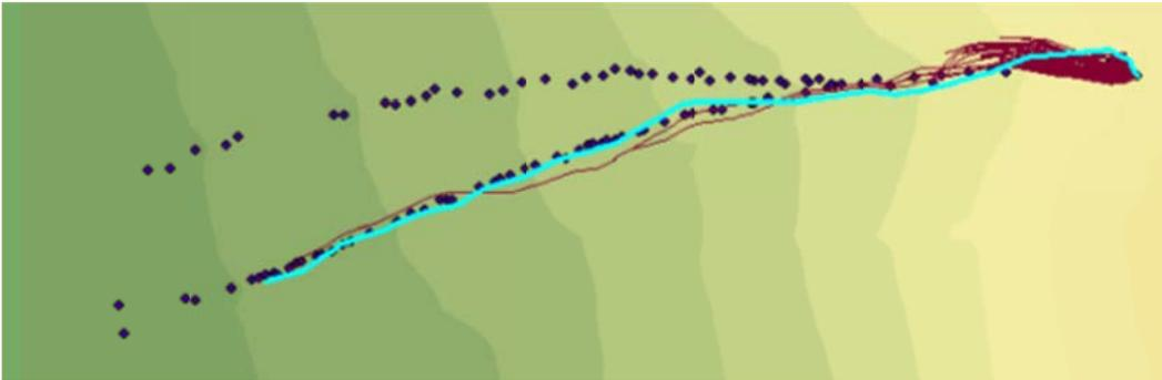
**Figure 5.29: Reduced COR Value Simulation (55° Slope Angle and 70m Drop Height)**
