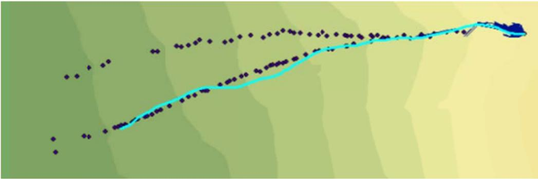
Figure C.3: Rockfall Simulation:  $R_n = 0.33$   $R_t = 0.87$ ; Slope Angle  $45^\circ$ ; Drop Height 20m
