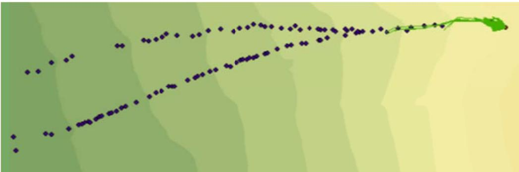
Figure C.45: Rockfall Simulation:  $R_n = 0.27$   $R_t = 0.77$ ; Slope Angle  $65^\circ$ ; Drop Height 50m
