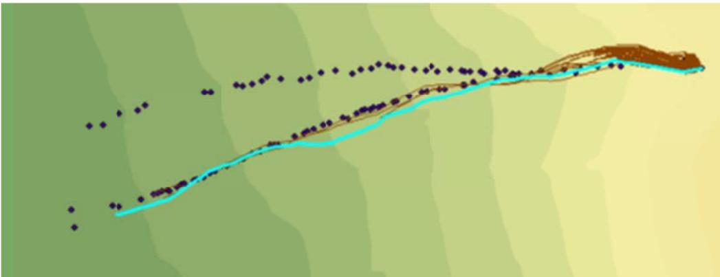
Figure C.15: Rockfall Simulation:  $R_n = 0.33$   $R_t = 0.87$ ; Slope Angle  $55^\circ$ ; Drop Height 70m
