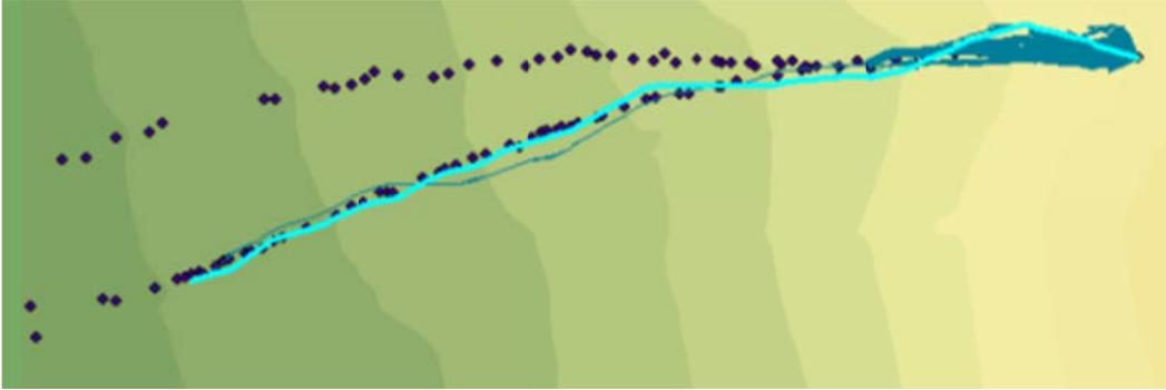
Figure C.57: Rockfall Simulation:  $R_n = 0.3$   $R_t = 0.77$ ; Slope Angle  $45^\circ$ ; Drop Height 50m
