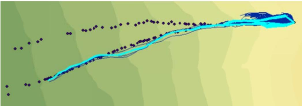
**Figure C.32: Rockfall Simulation:  $R_n = 0.3$   $R_t = 0.8$ ; Slope Angle  $45^\circ$ ; Drop Height 70m**
