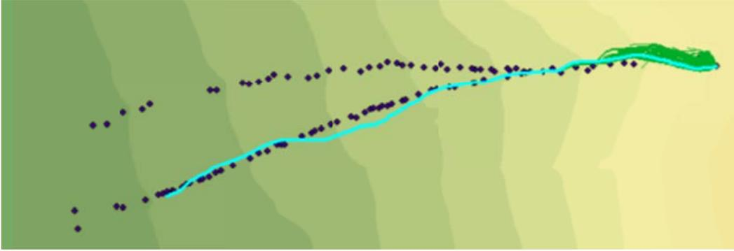
Figure C.43: Rockfall Simulation:  $R_n = 0.27$   $R_t = 0.77$ ; Slope Angle  $55^\circ$ ; Drop Height 60m
