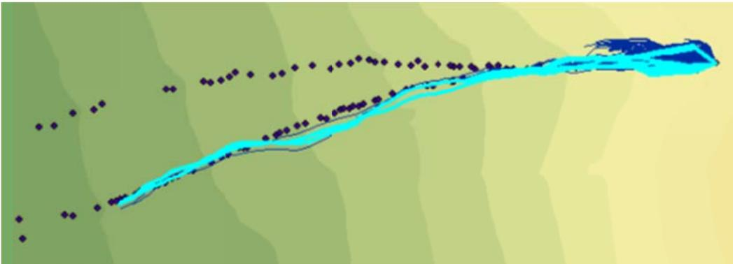
Figure C.59: Rockfall Simulation:  $R_n = 0.3$   $R_t = 0.77$ ; Slope Angle  $45^\circ$ ; Drop Height 70m
