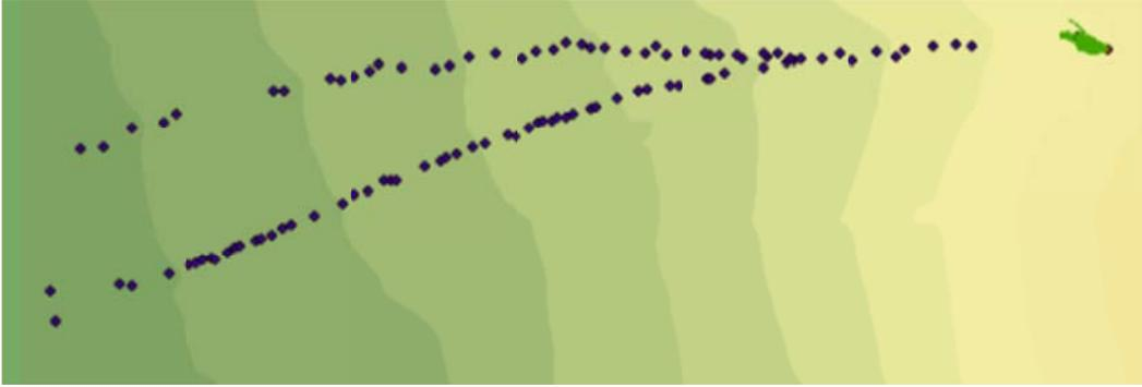
Figure C.16: Rockfall Simulation:  $R_n = 0.33$   $R_t = 0.87$ ; Slope Angle  $65^\circ$ ; Drop Height 10m
