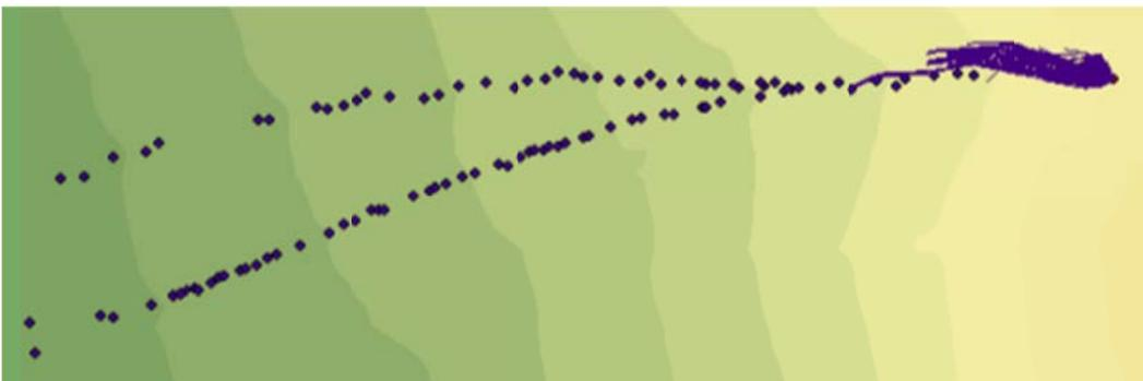
Figure C.70: Rockfall Simulation:  $R_n = 0.15$   $R_t = 0.5$ ; Slope Angle  $55^\circ$ ; Drop Height 60m
