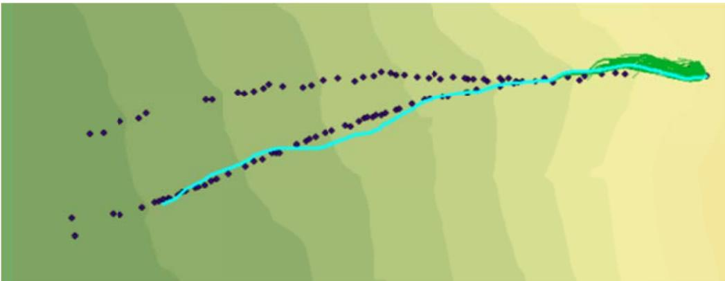
Figure C.34: Rockfall Simulation:  $R_n = 0.3$   $R_t = 0.8$ ; Slope Angle  $55^\circ$ ; Drop Height 60m
