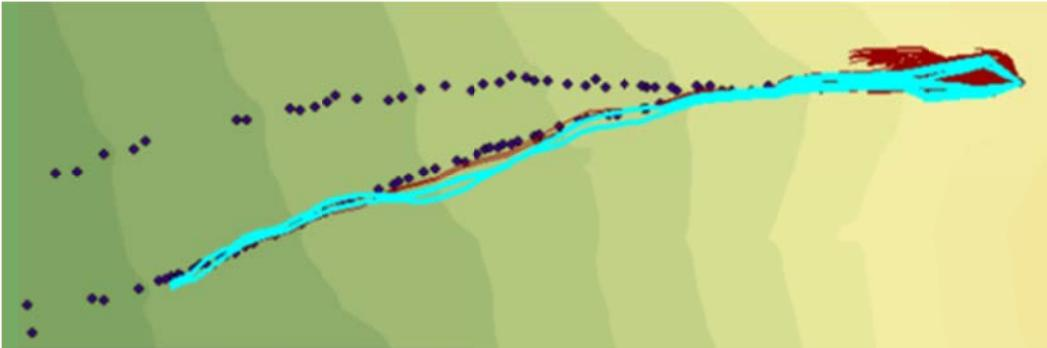
Figure C.68: Rockfall Simulation:  $R_n = 0.15$   $R_t = 0.5$ ; Slope Angle  $45^\circ$ ; Drop Height 70m
