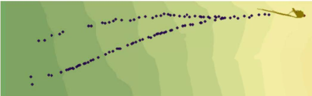
Figure C.11: Rockfall Simulation:  $R_n = 0.33$   $R_t = 0.87$ ; Slope Angle  $55^\circ$ ; Drop Height 30m
