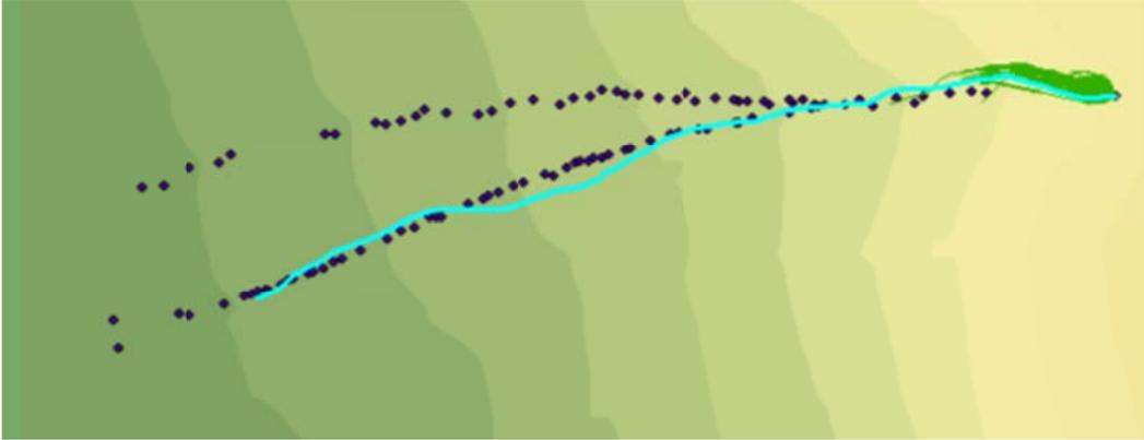
Figure C.33: Rockfall Simulation:  $R_n = 0.3$   $R_t = 0.8$ ; Slope Angle  $55^\circ$ ; Drop Height 50m
