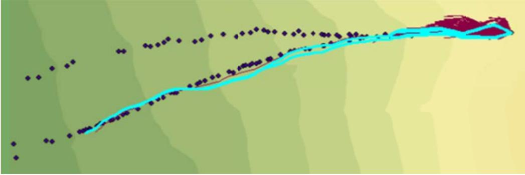
Figure C.67: Rockfall Simulation:  $R_n = 0.15$   $R_t = 0.5$ ; Slope Angle  $45^\circ$ ; Drop Height 60m
