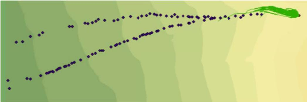
Figure C.51: Rockfall Simulation:  $R_n = 0.27$   $R_t = 0.8$ ; Slope Angle  $55^\circ$ ; Drop Height 50m
