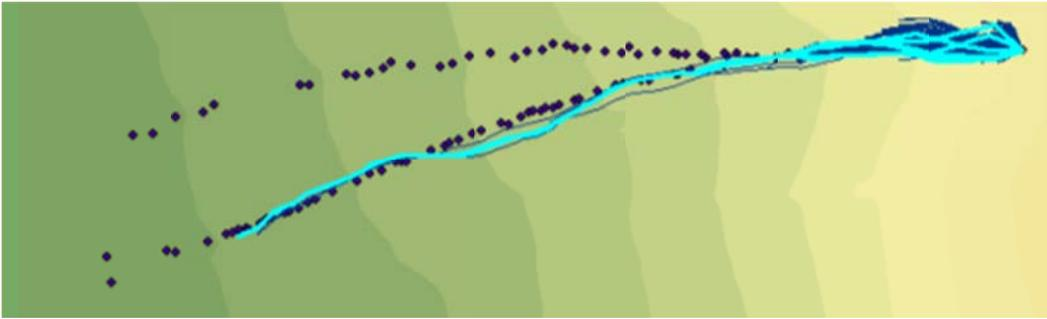
Figure C.40: Rockfall Simulation:  $R_n = 0.27$   $R_t = 0.77$ ; Slope Angle  $45^\circ$ ; Drop Height 60m
