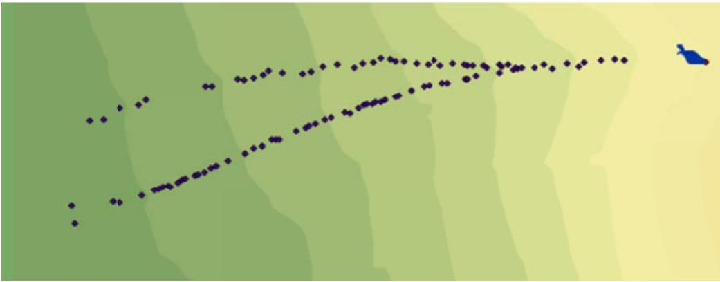
**Figure C.28: Rockfall Simulation:  $R_n = 0.33$   $R_t = 0.87$ ; Slope Angle  $75^\circ$ ; Drop Height 60m**
