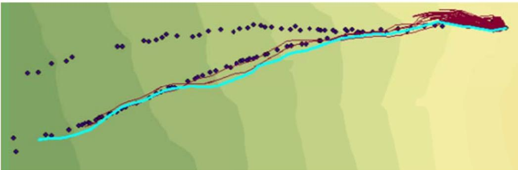
Figure C.62: Rockfall Simulation:  $R_n = 0.3$   $R_t = 0.77$ ; Slope Angle  $55^\circ$ ; Drop Height 70m
