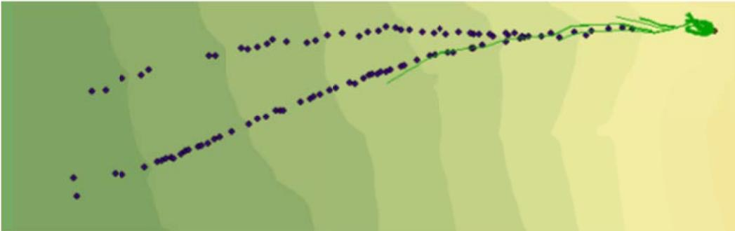
Figure C.10: Rockfall Simulation:  $R_n = 0.33$   $R_t = 0.87$ ; Slope Angle  $55^\circ$ ; Drop Height 20m
