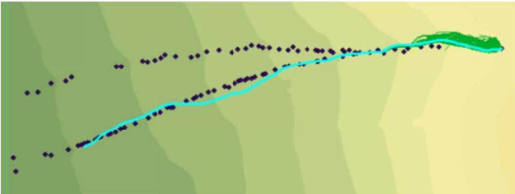
Figure C.52: Rockfall Simulation:  $R_n = 0.27$   $R_t = 0.8$ ; Slope Angle  $55^\circ$ ; Drop Height 60m
