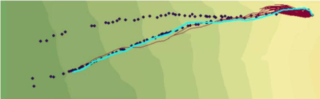
Figure C.44: Rockfall Simulation:  $R_n = 0.27$   $R_t = 0.77$ ; Slope Angle  $55^\circ$ ; Drop Height 70m
