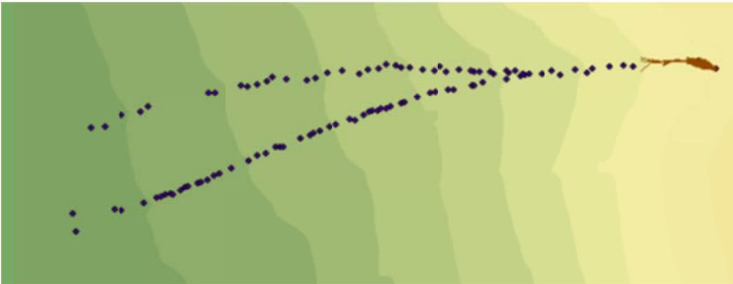
Figure C.24: Rockfall Simulation:  $R_n = 0.33$   $R_t = 0.87$ ; Slope Angle  $75^\circ$ ; Drop Height 20m
