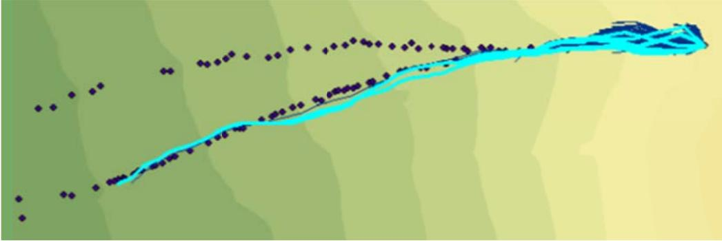
Figure C.85: Rockfall Simulation:  $R_n = 0.3$   $R_t = 0.5$ ; Slope Angle  $45^\circ$ ; Drop Height 60m
