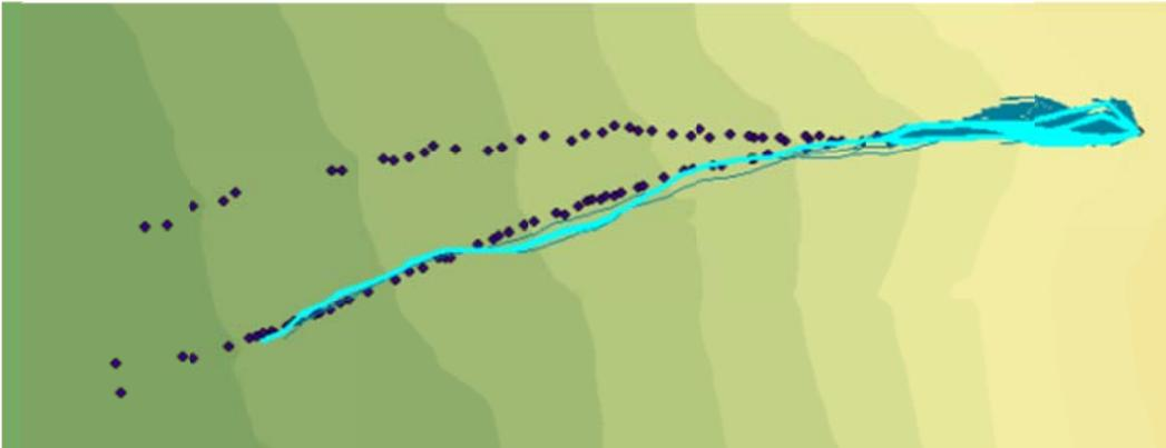
**Figure C.31: Rockfall Simulation:  $R_n = 0.3$   $R_t = 0.8$ ; Slope Angle  $45^\circ$ ; Drop Height 60m**
