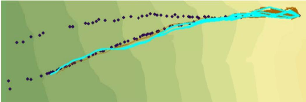
**Figure C.75: Rockfall Simulation:  $R_n = 0.15$   $R_t = 0.8$ ; Slope Angle  $45^\circ$ ; Drop Height 50m**
