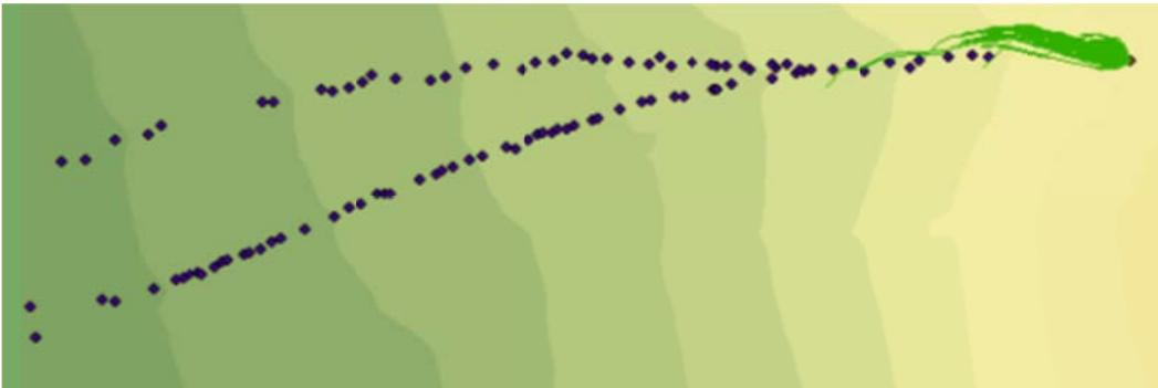
Figure C.87: Rockfall Simulation:  $R_n = 0.3$   $R_t = 0.5$ ; Slope Angle  $55^\circ$ ; Drop Height 50m
