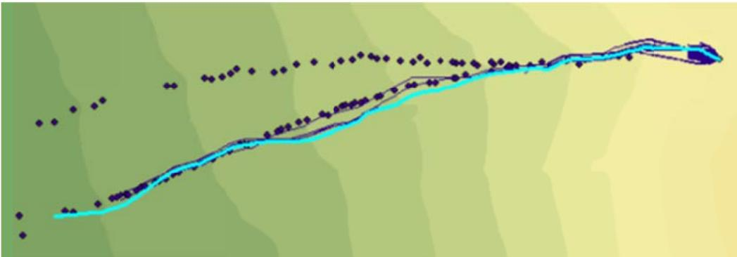
Figure C.56: Rockfall Simulation:  $R_n = 0.27$   $R_t = 0.8$ ; Slope Angle  $65^\circ$ ; Drop Height 70m
