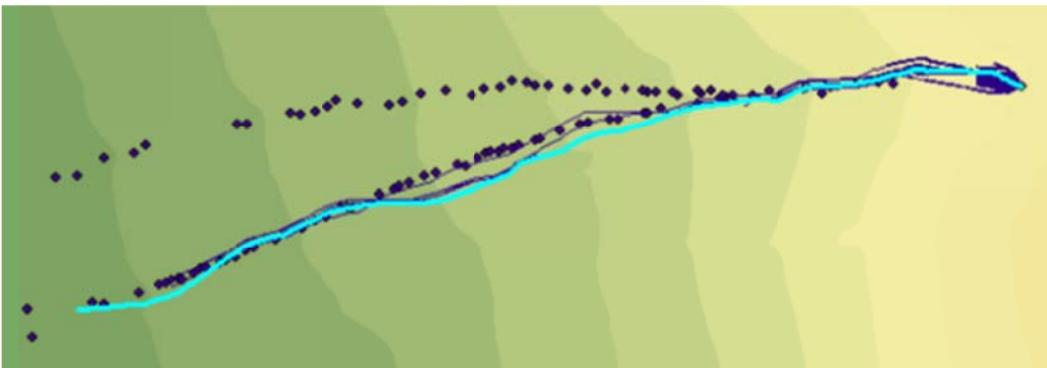
Figure 5.32: Reduced Normal Typical Tangential COR Value Simulation (65° Slope Angle and 70m Drop Height)
