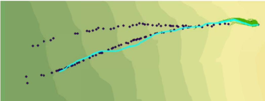
Figure C.12: Rockfall Simulation:  $R_n = 0.33$   $R_t = 0.87$ ; Slope Angle  $55^\circ$ ; Drop Height 40m
