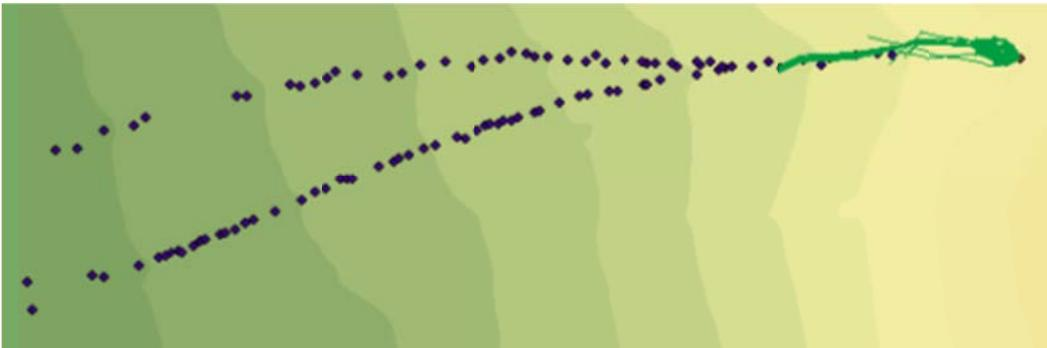
Figure C.91: Rockfall Simulation:  $R_n = 0.3$   $R_t = 0.5$ ; Slope Angle  $65^\circ$ ; Drop Height 60m
