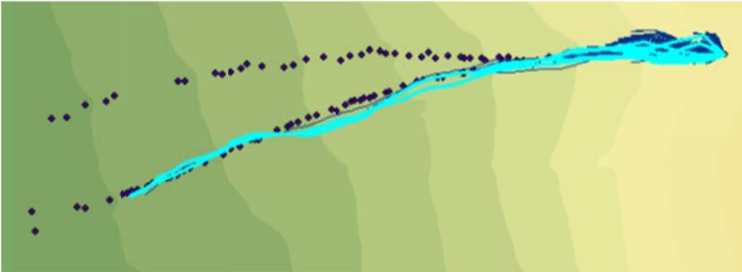
Figure C.58: Rockfall Simulation:  $R_n = 0.3$   $R_t = 0.77$ ; Slope Angle  $45^\circ$ ; Drop Height 60m
