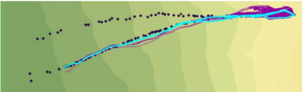
Figure C.8: Rockfall Simulation:  $R_n = 0.33$   $R_t = 0.87$ ; Slope Angle  $45^\circ$ ; Drop Height 70m
