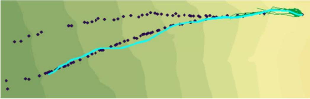
**Figure C.64: Rockfall Simulation:  $R_n = 0.3$   $R_t = 0.77$ ; Slope Angle  $65^\circ$ ; Drop Height 60m**
