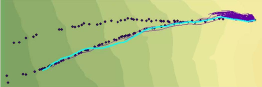
**Figure 5.37: Greatly Reduced Normal Typical Tangential COR Value Simulation (55° Slope Angle and 70m Drop Height)**
