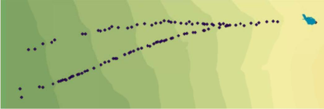
Figure C.9: Rockfall Simulation:  $R_n = 0.33$   $R_t = 0.87$ ; Slope Angle  $55^\circ$ ; Drop Height 10m
