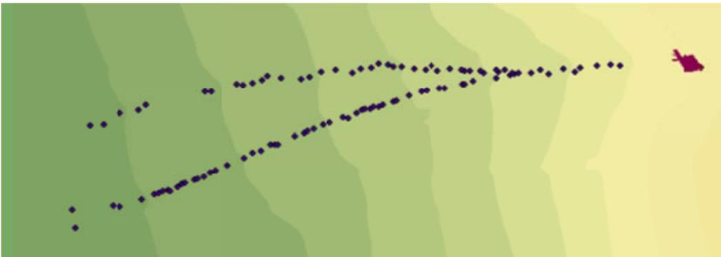
Figure C.18: Rockfall Simulation:  $R_n = 0.33$   $R_t = 0.87$ ; Slope Angle  $65^\circ$ ; Drop Height 30m
