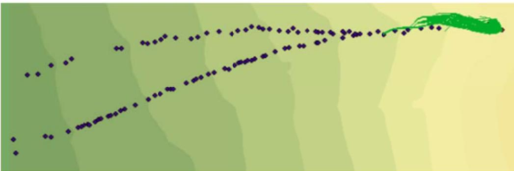
Figure C.88: Rockfall Simulation:  $R_n = 0.3$   $R_t = 0.5$ ; Slope Angle  $55^\circ$ ; Drop Height 60m
