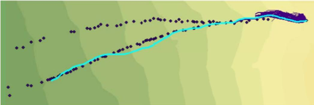
Figure C.79: Rockfall Simulation:  $R_n = 0.15$   $R_t = 0.8$ ; Slope Angle  $55^\circ$ ; Drop Height 60m
