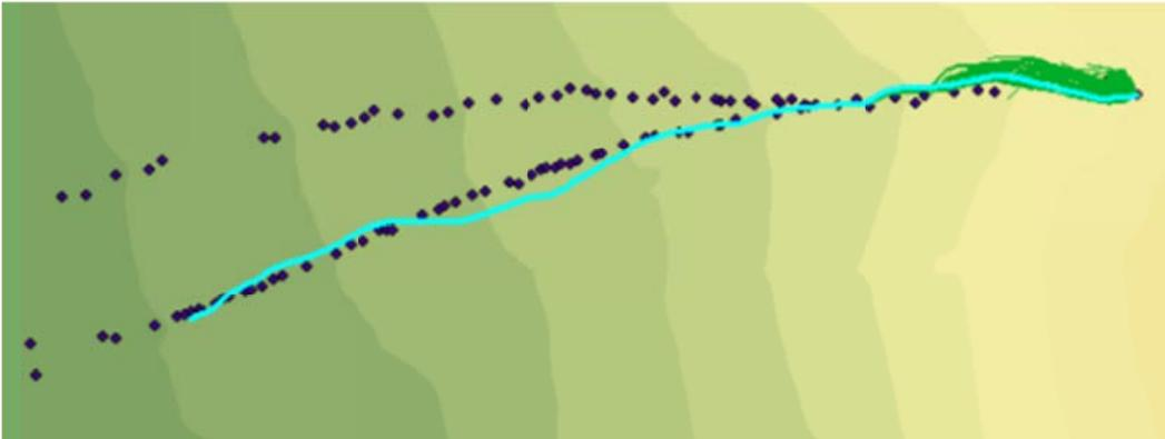
Figure C.61: Rockfall Simulation:  $R_n = 0.3$   $R_t = 0.77$ ; Slope Angle  $55^\circ$ ; Drop Height 60m
