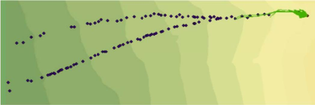
Figure C.54: Rockfall Simulation:  $R_n = 0.27$   $R_t = 0.8$ ; Slope Angle  $65^\circ$ ; Drop Height 50m
