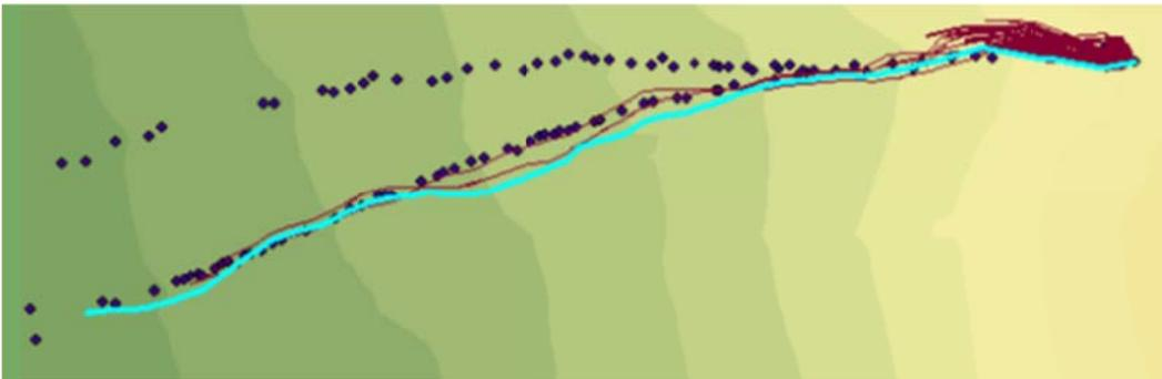
Figure 5.33: Typical Normal Reduced Tangential COR Value Simulation (55° Slope Angle and 70m Drop Height)
