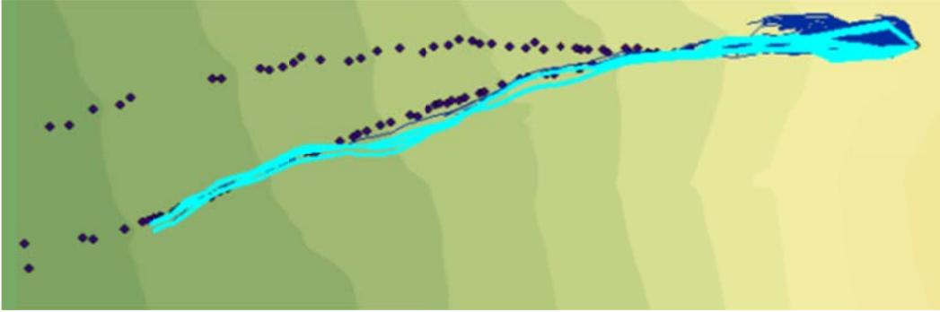
Figure C.50: Rockfall Simulation:  $R_n = 0.27$   $R_t = 0.8$ ; Slope Angle  $45^\circ$ ; Drop Height 70m
