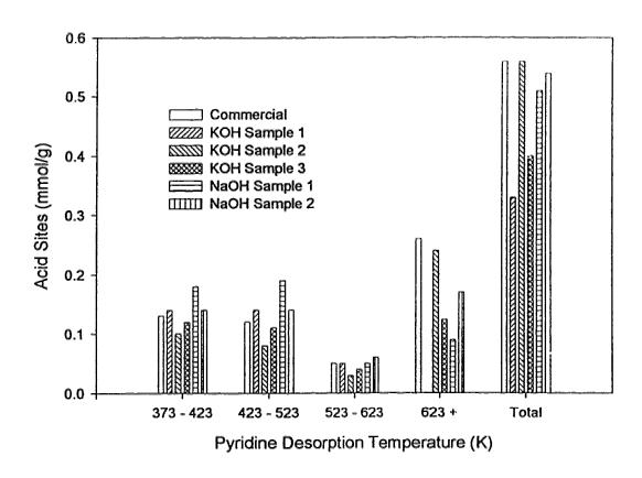
Figure 6.7: Distribution of Strengths of Acid Sites for Commercial, KOH Doped Catalyst (0.28 meq/g catalyst) and NaOH Doped Catalyst (0.26 meq/g catalyst). (See Appendix 6.2.)
