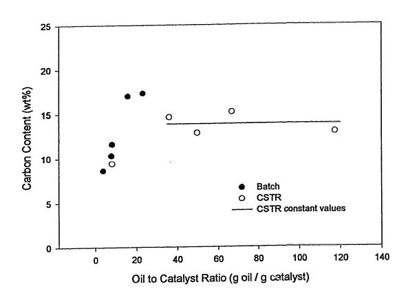
Figure 2.3: Carbon Content of Spent Catalyst as a Function of Cumulative Feed Oil to Catalyst Ratio. All experiments at 13.8 MPa, 430°C. Data for batch reactor are for repeated contacts of catalyst with fresh feed (see samples B1, B2, and B6 to B8 in Appendix 2.1), data for CSTR are from experiments C1,C2,C8,C13,C14 (Table 2.2).
