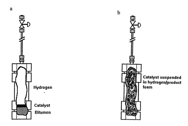
Figure 2.2a: Batch Reactor with Cut Away Section Showing Relative Amounts of Hydrogen, Bitumen and Catalyst after Loading.
