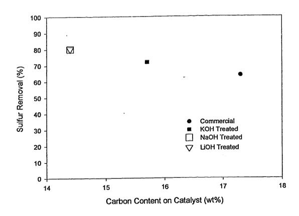
Figure 6.6: Average Hydrodesulfurization Activity for Commercial Catalyst and Catalysts Doped with 0.28 meq KOH / g catalyst, 0.26 meq NaOH / g catalyst and 0.26 meq LiOH / g catalyst versus Carbon Content of the Catalyst. All experiments were 1 h long at 430°C, 13.8 MPa.
