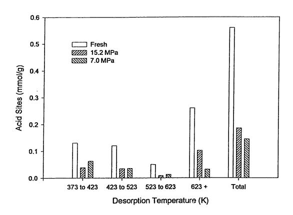
Figure 4.1: Distribution of Strengths of Acid Sites by Stepwise Thermal Desorption. The concentration of sites is shown on the ordinate while the abscissa values are the temperature ranges for desorption of pyridine.
