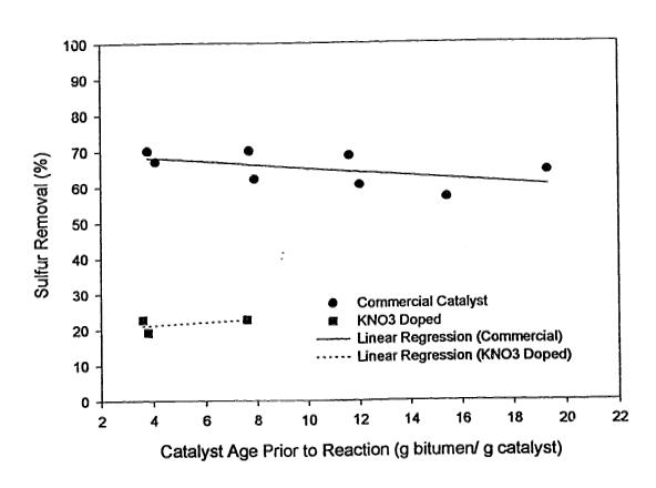
Figure 6.3: Hydrodesulfurization Activity for Commercial Catalyst and Catalyst Doped with 9.8 meq KNO<sub>3</sub>/g catalyst. (See Appendix 6.1) All experiments were 1 h long at 430°C, 13.8 MPa.
