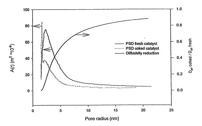
Figure 5.1: Pore Size Distribution (PSD) Based on Surface Area and the Reduction in Effective Diffusivity Caused by Coke Deposition. Total Surface Area =  $\int_{0}^{\infty} A(r)dr$ .
