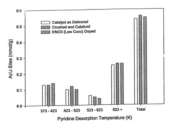
Figure 6.2: Distribution of Strengths of Acid Sites for Commercial Catalyst as Delivered, Crushed and Calcined Commercial Catalyst and Low Concentration (0.26 meq/g catalyst) KNO<sub>3</sub> Doped Catalyst. (See Appendix 6.2)
