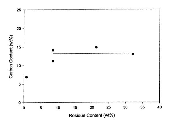
Figure 2.4: Carbon Content of Spent Catalyst as a Function of Residue Concentration in the CSTR. All experiments at 13.8 MPa, 430°C. The line represents the average carbon concentration observed at intermediate residue concentrations. (Data are from Runs C8 - C12, Table 2.2).
