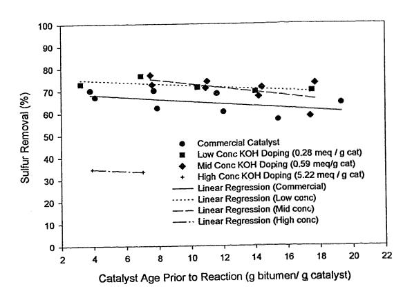
Figure 6.4: Hydrodesulfurization Activity for Commercial Catalyst and Catalyst Doped with 0.28 meq KOH / g catalyst, 0.59 meq KOH / g catalyst and 5.22 meq KOH / g catalyst. (See Appendix 6.1.) All experiments are 1 h long at 430°C, 13.8 MPa.
