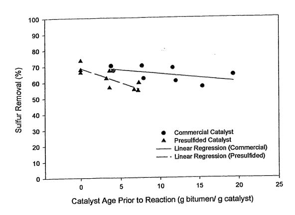
Figure 6.1: Hydrodesulfurization Activity for Commercial Catalyst and Presulfided Commercial Catalyst. (See Appendix 6.1.) All experiments were 1 h long at 430°C, 13.8 MPa.
