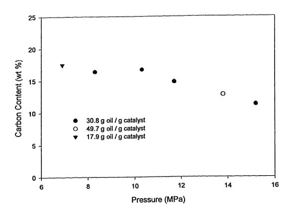
Figure 2.5: Carbon Content of Spent Catalyst as a Function of Hydrogen Pressure for CSTR Experiments. All experiments at 430°C. Data are available in Table 2.2 (Samples C3 to C7).
