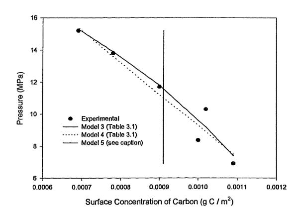
Figure 3.3: Surface Concentration of Carbon as a function of Hydrogen Pressure. Figure shows experimental data, and the curves fitted to Models 3 and 4, as defined in Table 3.1. Figure also shows the results of Model 5, as described in the text. It assumes that production of active hydrogen species is independent of hydrogen pressure.
