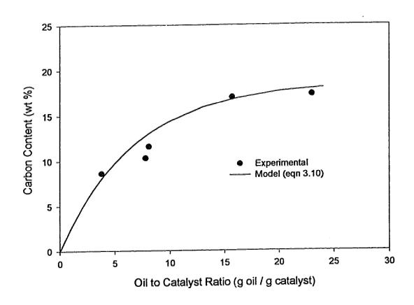
Figure 3.4: Carbon Concentration in Spent Catalyst as a Function of Cumulative Feed Oil to Catalyst Ratio in the Batch Reactor. All experiments at 13.8 MPa, 430°C. Model shown is per equation 3.10, where  $C_{\text{max}} = 18.56$  (wt%) and k = 0.15 (g cat/ g bitumen).
