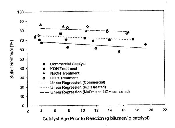
Figure 6.5: Hydrodesulfurization Activity for Commercial Catalyst and Catalysts Doped with 0.28 meq KOH/g catalyst, 0.26 meq NaOH/g catalyst and 0.26 meq LiOH/g catalyst. (See Appendix 6.1) All experiments were 1 h long at 430°C, 13.8 MPa.
