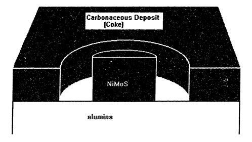
Figure 3.1: Schematic Representation of Catalyst Surface, Showing a Cross Section through the Metal Crystallite.
