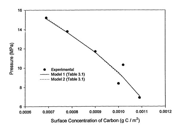
Figure 3.2: Surface Concentration of Carbon as a Function of Hydrogen Pressure (Models 1 and 2). Figure shows experimental data, and the curves fitted to Models 1 and 2, as defined in Table 3.1.
