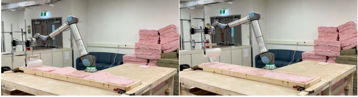
Figure D.3: H-GLPPR process for Scenario 3 with 15 x 3.5-inch (381 x 89 mm) fiberglass insulation
