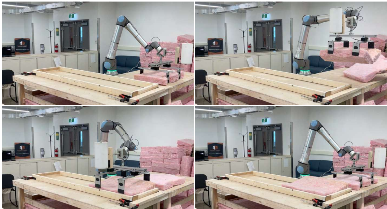
Figure 3.10: H-GLPPR process and completion with 15 x 3.5-inch (381 x 89 mm) mineral wool insulation size for Scenario 2 (Grasp 1st piece, Lift 1st piece, Place 1st piece, Grasp 2nd piece, Lift 2nd piece, Place 2nd piece, Press, Roll, Completion)
