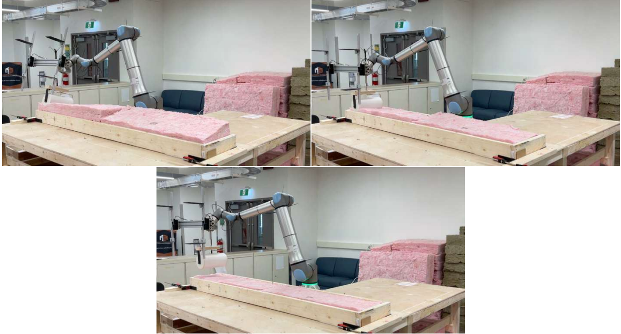
Figure D.11: H-GLPPR process for Scenario 2 with 15 x 5.5-inch (381 x 140 mm) fiberglass insulation
