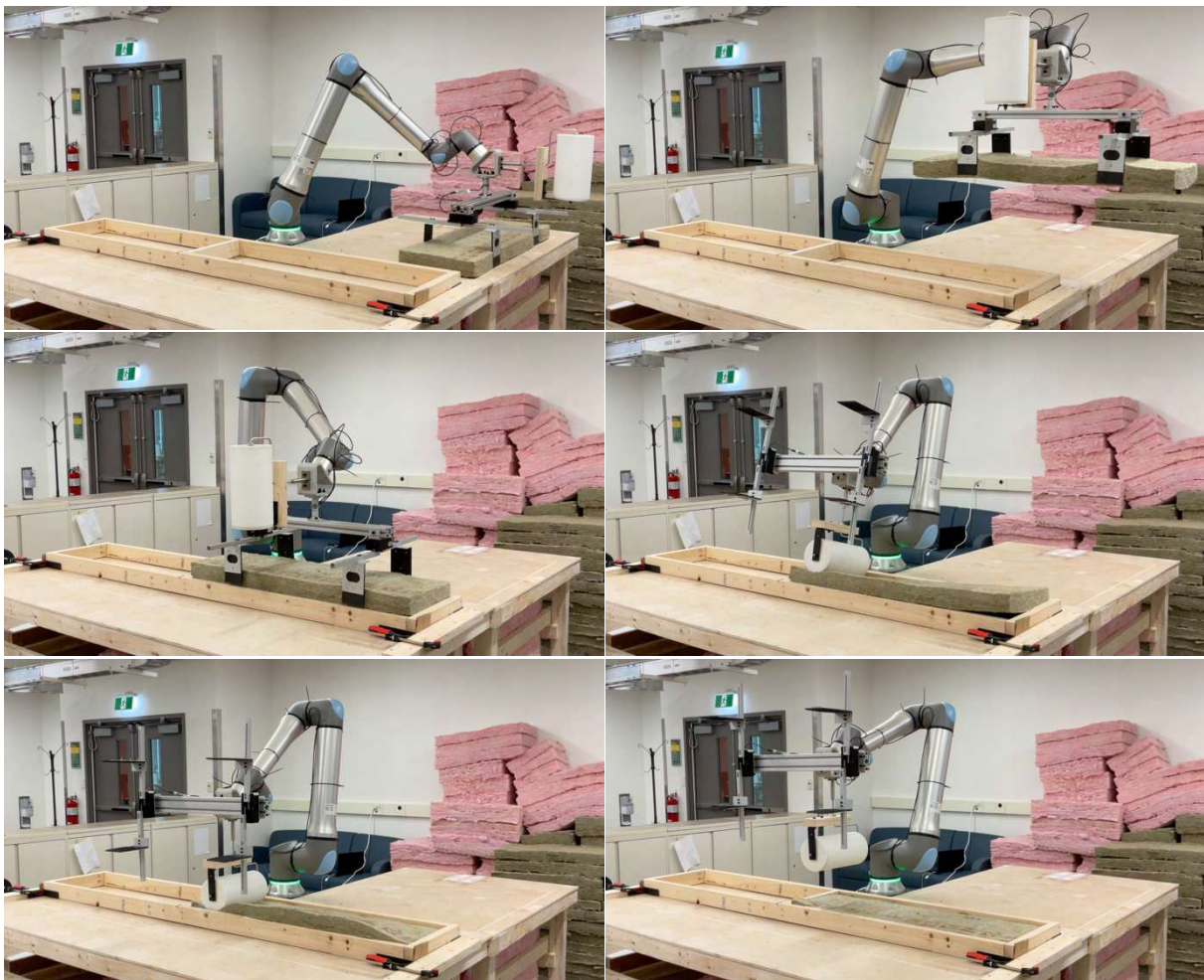
Figure D.4: H-GLPPR process for Scenario 1 with 15 x 3.5-inch (381 x 89 mm) mineral wool insulation
