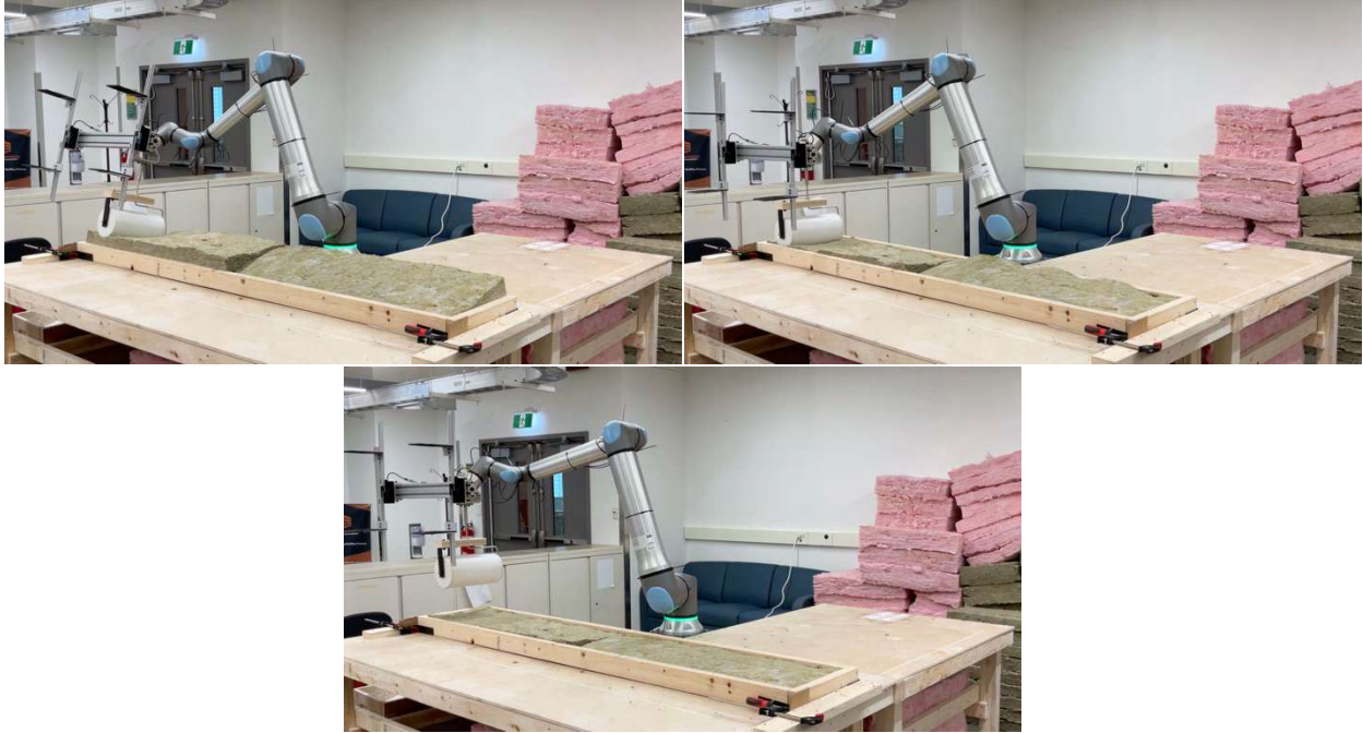
Figure 3.10: H-GLPPR process and completion with 15 x 3.5-inch (381 x 89 mm) mineral wool insulation size for Scenario 2 (Grasp 1st piece, Lift 1st piece, Place 1st piece, Grasp 2nd piece, Lift 2nd piece, Place 2nd piece, Press, Roll, Completion)
