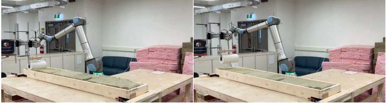
Figure D.15: H-GLPPR process for Scenario 3 with 15 x 5.5-inch (381 x 140 mm) mineral wool insulation
