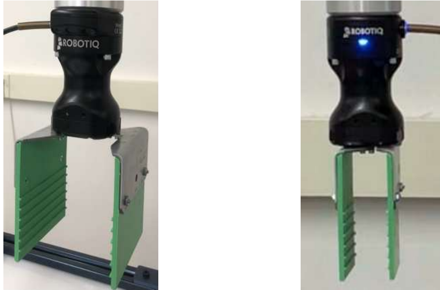
Figure 2.4: The prototyped robotic end-effector at fully open position (left) and at fully closed position (right)
