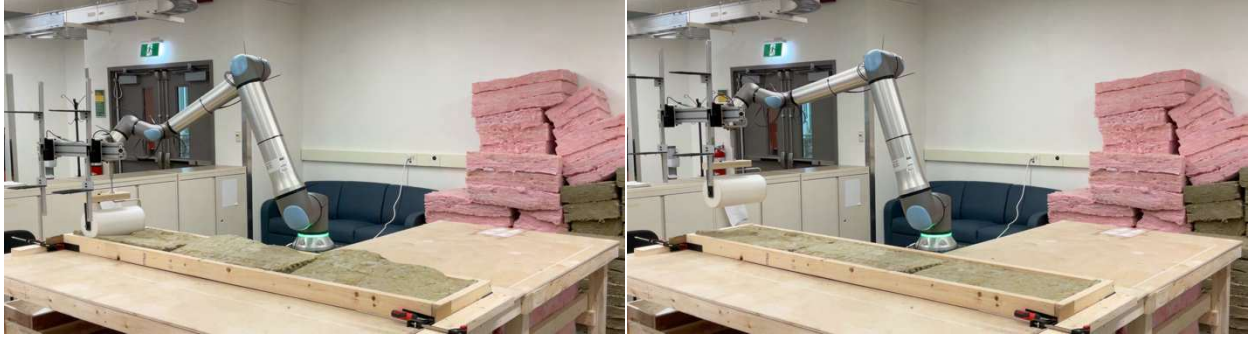
Figure D.5: H-GLPPR process for Scenario 3 with 15 x 3.5-inch (381 x 89 mm) mineral wool insulation
