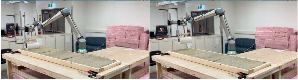
Figure D.10: H-GLPPR process for Scenario 3 with 23 x 3.5-inch (584 x 89 mm) mineral wool insulation
