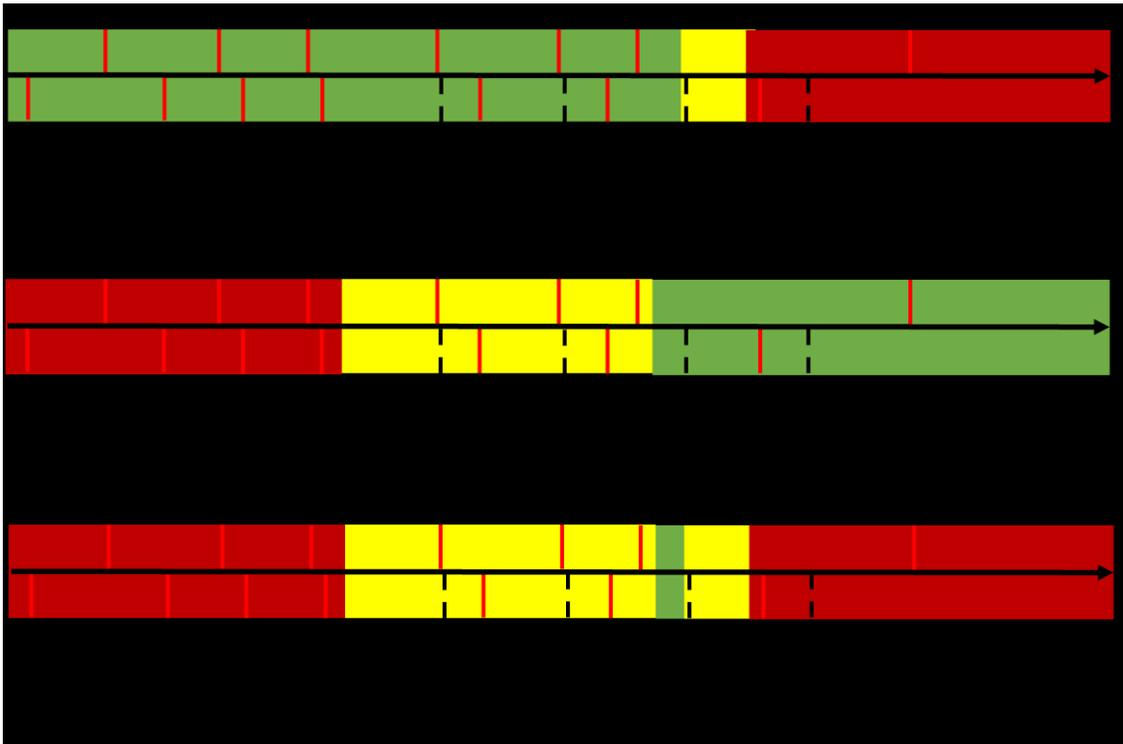
Fig. 14 Traffic light bars for SPC=30 at moderate fluid flow rates (0.72 to 1.31 bbl/day/ft<sup>2</sup>), (a) sand production, (b) retained permeability, and (c) overall design criteria
