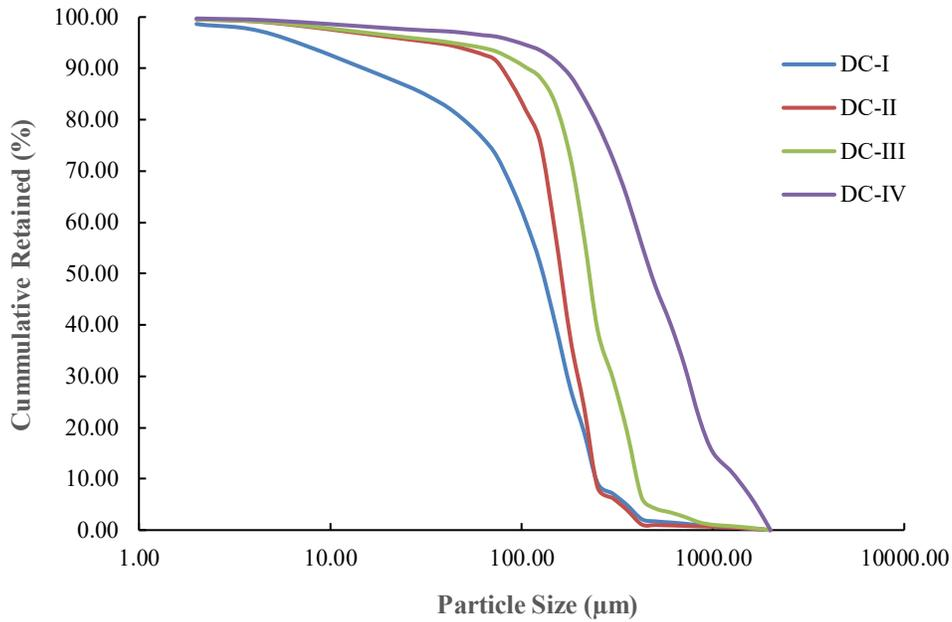
Fig. 2 PSD classes for McMurray Formation oil sands (Abram and Cain, 2014)
