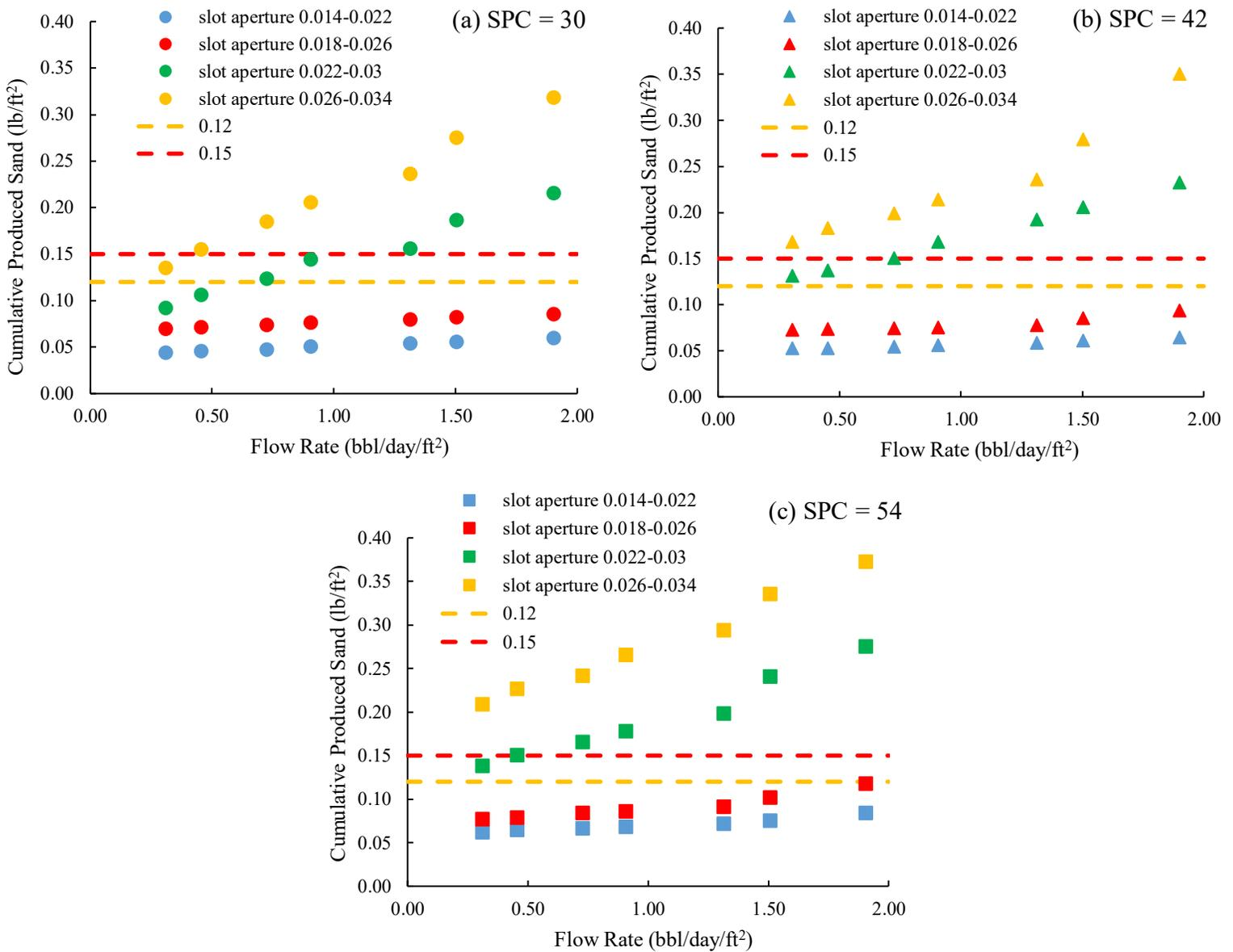
Fig. 8 Cumulative produced sand for different fluid flow rates (a) SPC=30, (b) SPC =42, and (c) SPC=54
