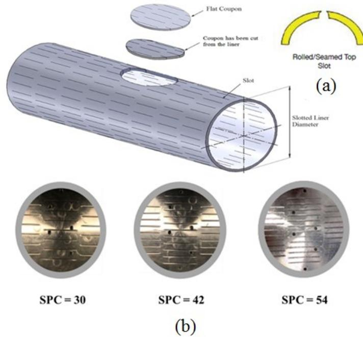
Fig. 5 Multi-slot coupons with seamed slots
