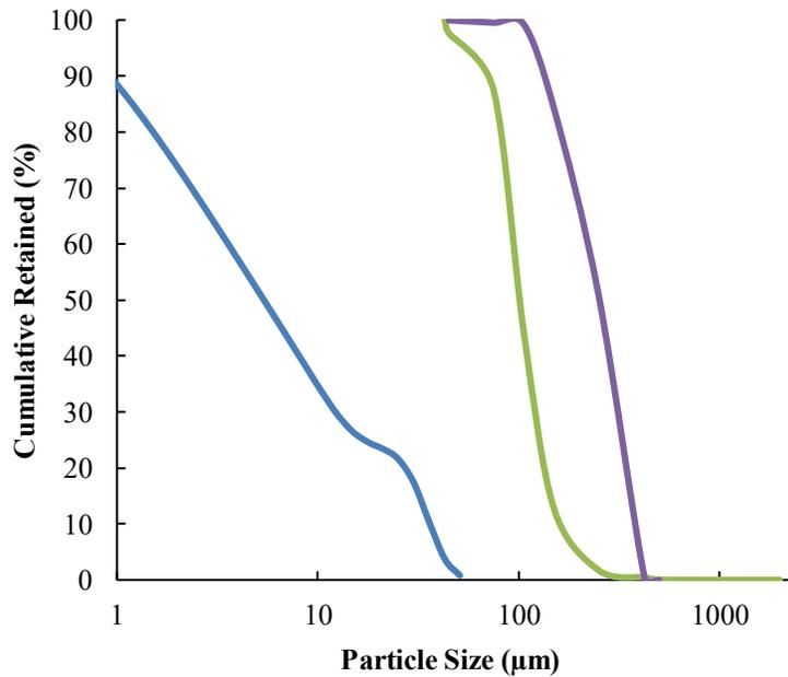
Fig. 3 PSD classes for three commercial sands
