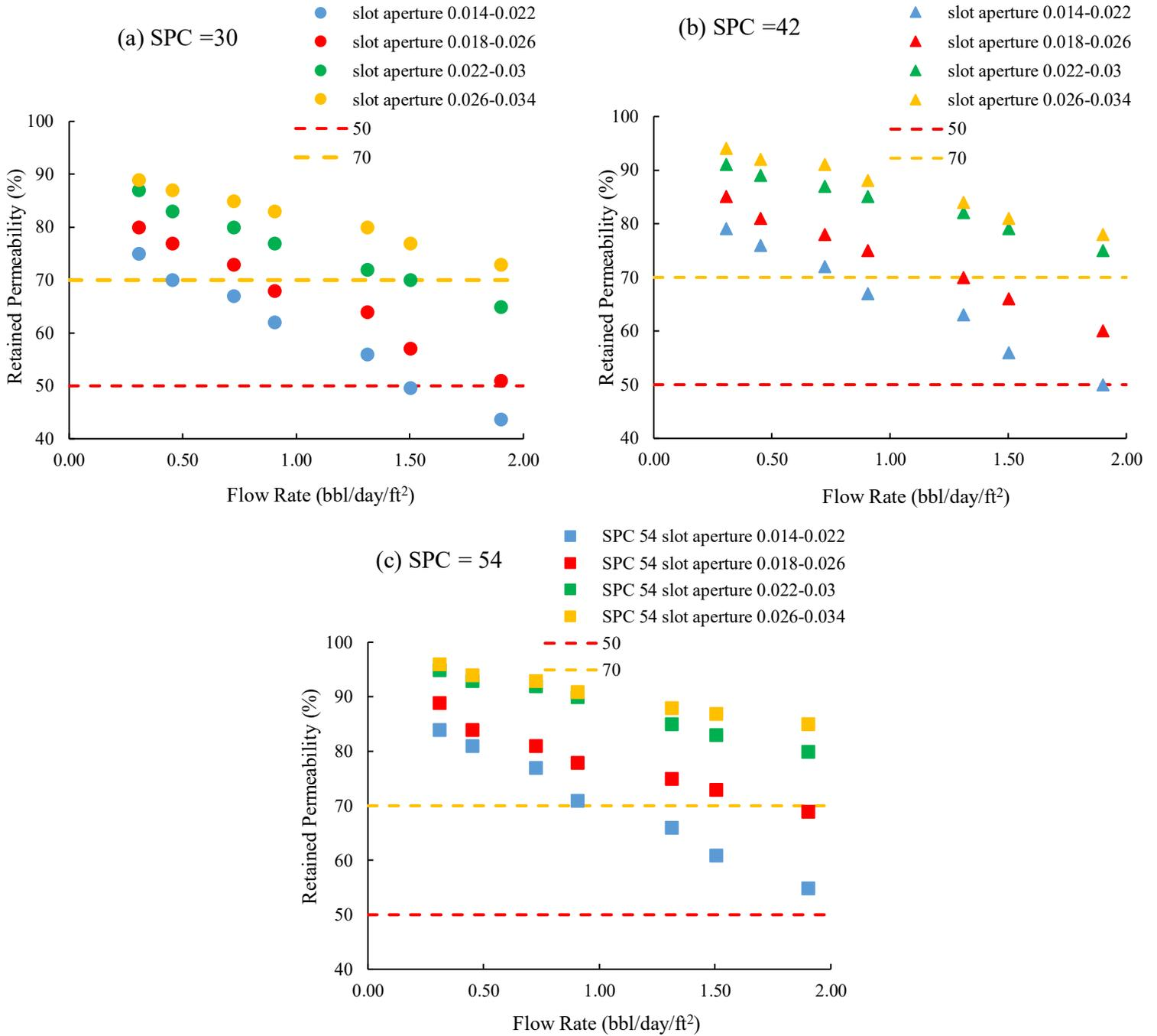
Fig. 9 Retained permeability at different fluid flow rates (a) SPC=30, (b) SPC=42, and (c) SPC=54
