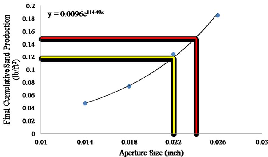
Fig. 11 Interpolation procedure in Traffic light bar of sand production for SPC=30 at the mild fluid flow rate (< 0.72 bbl/day/ft<sup>2</sup>)
