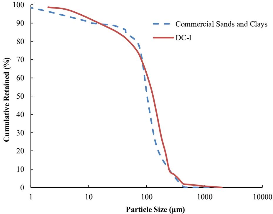
Fig. 4 PSD curves for DC-I and the commercial sand mixture
