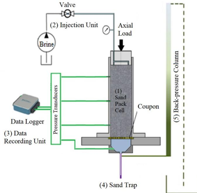
Fig. 6 The schematic view of the SRT apparatus
