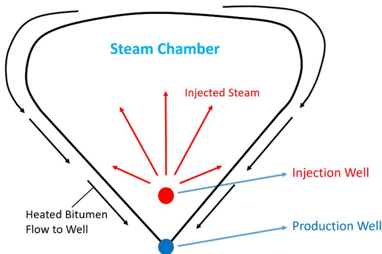
Fig. 1 The schematic concept of the steam chamber (modified from Butler, 1985)
