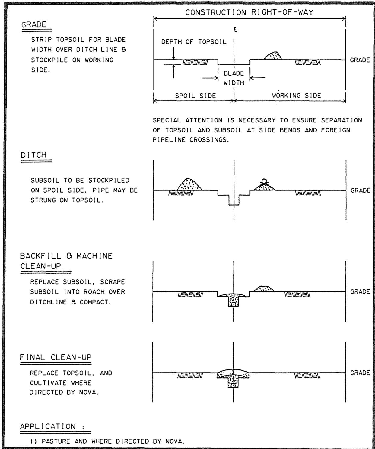
Figure 4. Topsoil Conservation over the Ditchline and Spoil Side during Summer Construction (NGTL 1990).
