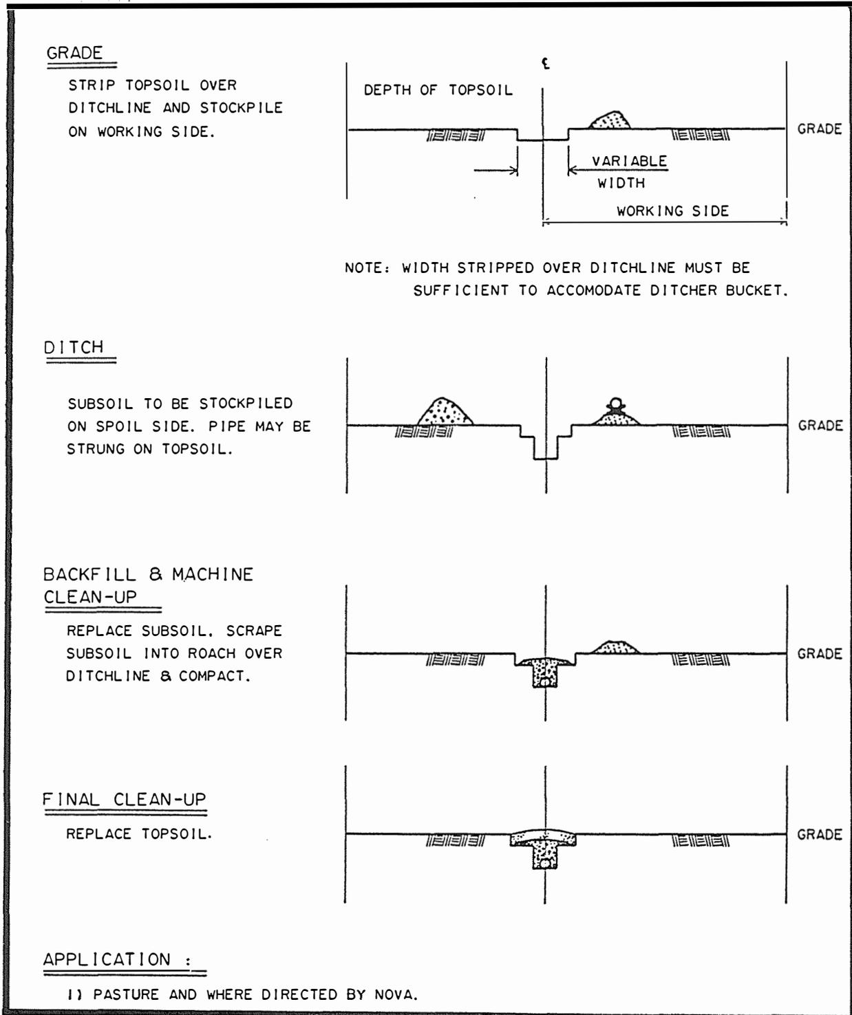
Figure 3. Topsoil Conservation using Blade Width Stripping during Summer Construction (NGTL 1990).
