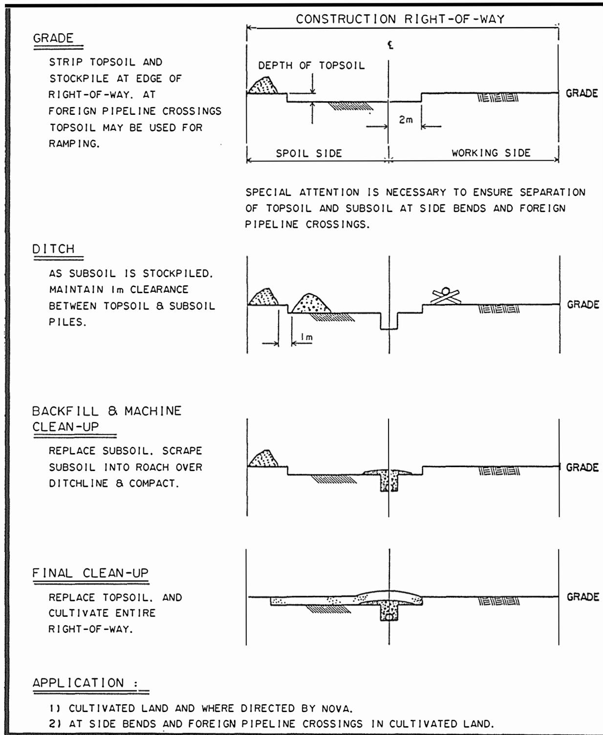
Figure 5. Topsoil Conservation over the Ditchline and Work Side during Summer Construction (NGTL 1992).
