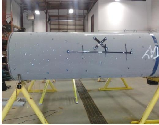
Figure 3.14 Complete pipe setup with reference cross, bars, and coded targets
