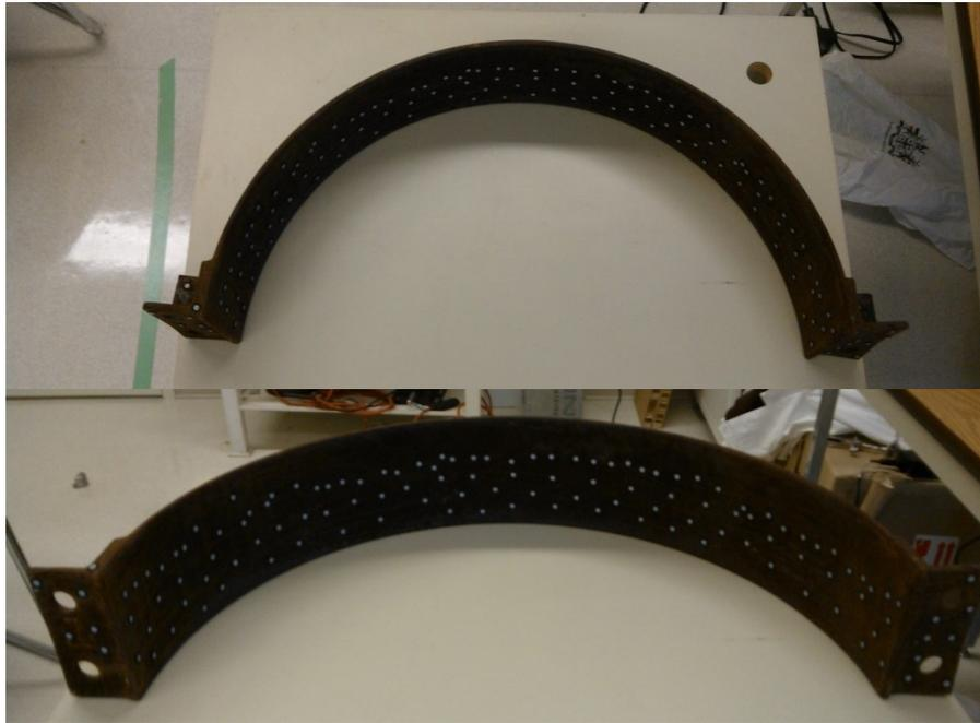
Figure 3.21 NPS 30 inch pipe clamp set up with reflective targets
