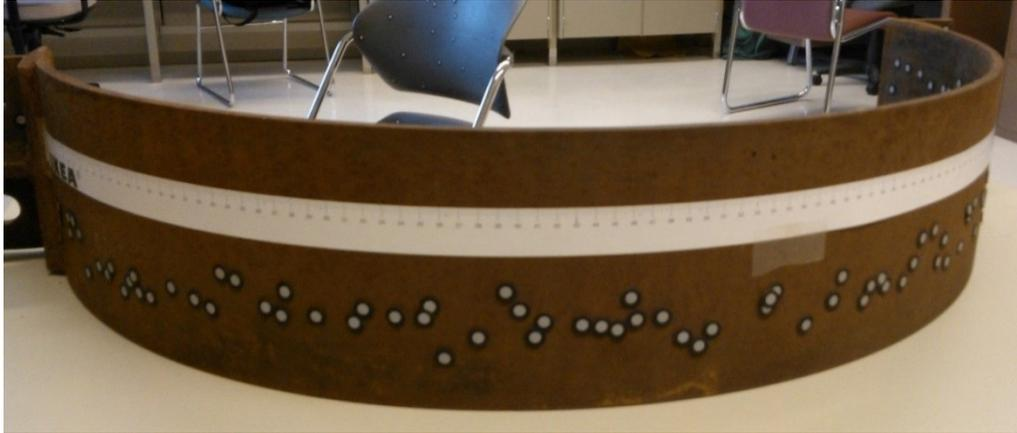
Figure 3.24 Measuring grid on the pipe clamp
