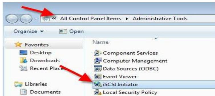
When the screen in Figure 33 appears, write down the SAN server IP and click connect.
