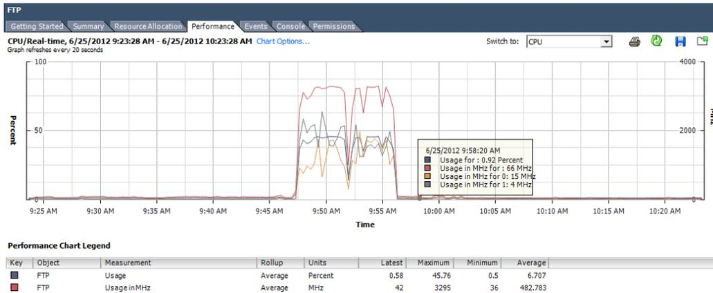
Under high load, when 20 GB data was being transferred to FTP server, the maximum rate at which the server received data was 1.5 Mbps and at that time network usage was 1.2 Mbps.
