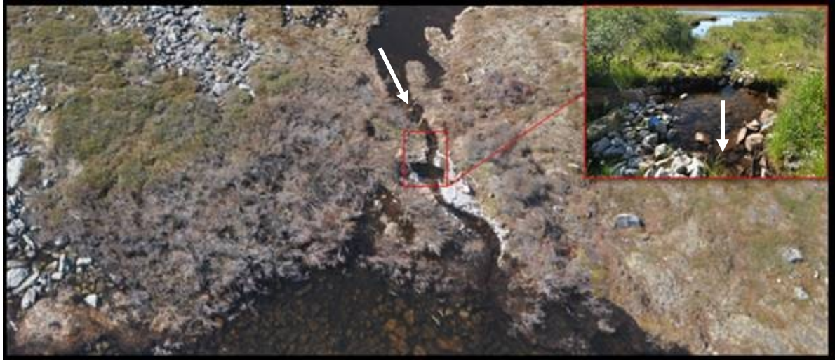
Figure 1-10. Nature-like treatment at M2S. M1L (downstream) is at the bottom; M2L (upstream) is at the top. Red box indicates location of photo insert depicting more detail of the choke-and-pool structure; white arrows indicate direction of flow. Photo taken June 7, 2012; insert photo taken June 27, 2013.
