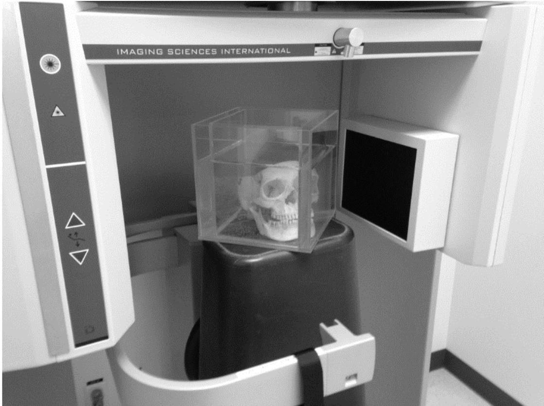
**Figure 3-1: Dry skull placed within container with water compartment to simulate tissue in the iCAT machine**
