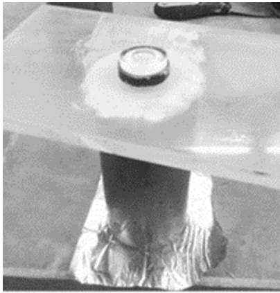
Figure 3- 4. Soilcrete before performing UCS test. Detail of gypsum cap on soilcrete being leveled.
