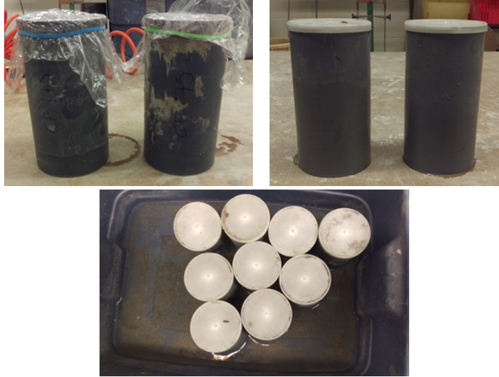
Figure E-4. Soilcrete specimens in plastic molds.
