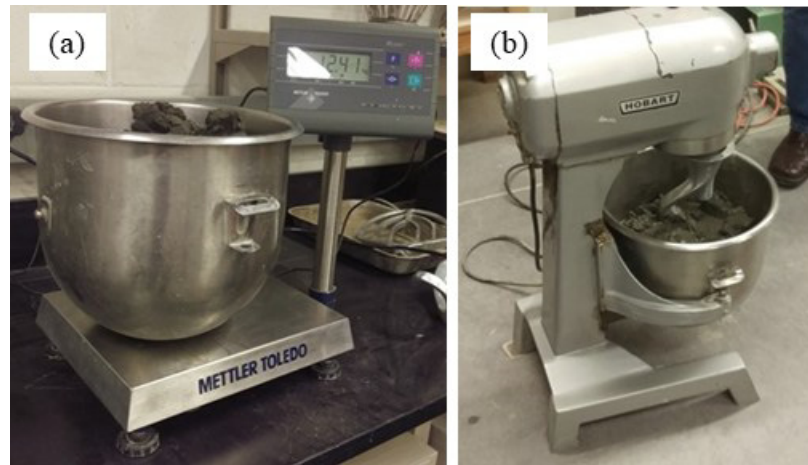
Figure E-2. (a) soil being weighed in dough mixer cup, and (b) cup with soil placed on dough mixer.
