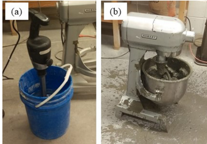
Figure E-3. (a) blender with bucket containing water-cement slurry, and (b) dough mixer with soil and slurry.
