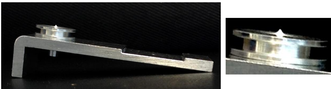
Figure 4.8. Collected pharmaceutical particles from one single pMDI actuation containing 300 \mu g actives
