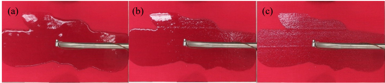
Figure 4.7. Fabric SS-3 with hydrophobic finish exposed to hot water at 90°C during cooling period – photographs taken (a) 10 s, (b) 30 s and (c) 60 s after the termination of the exposure in horizontal tests.
