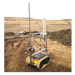
Figure 2.3: Robotic system for tailings characterization.
