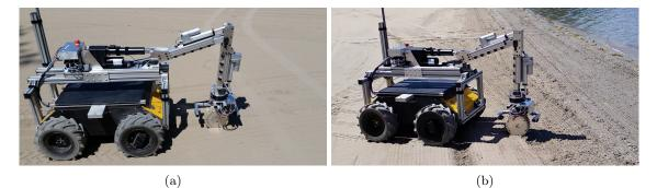
Figure 5.19: RTC-II deploying the instrumented terramechanics wheel on (a) dry sand, (b) transition between dry and wet sand.
