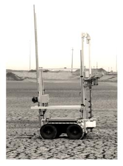
Figure 5.3: RTC-I collecting subsurface samples from an oil sands tailings DDA.
