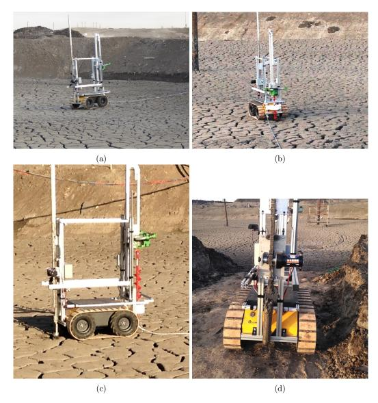
Figure 2.15: (a) RTC-I teleoperated into an experimental cell. (b) Drilling thought the crust. (c) Sampling tool lowered through the curst. (d) RTC-I with sample collected from 1.7 m depth.
