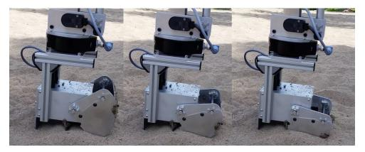
Figure 5.16: Sampler payload collecting a sample on dry sand.
