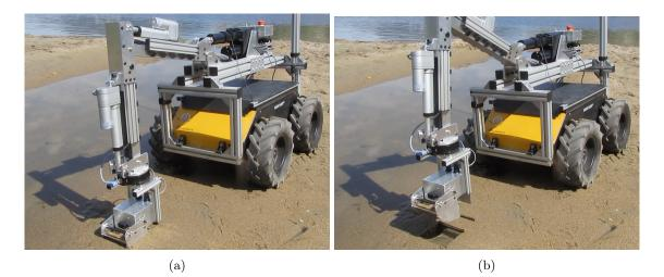
Figure 5.17: RTC-II collecting a sample on saturated sand. (a) The manipulator arm positions the sampler on the terrain and the scoop is closed slowly to collect material. (b) The manipulator lifts the instrument carrying a sample of saturated sand. The soil had sufficient cohesion to maintain the shape of the material collected after the sampler was removed form the ground.
