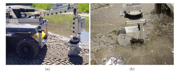
Figure 6.14: Surface samples are collected using a robotic manipulator on (a) sandy terrain and, (b) centrifuged tailings.
