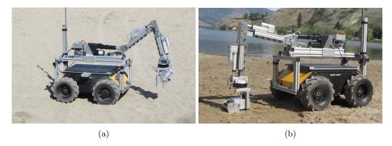
Figure 5.15: (a) RTC-II traversing dry uncompacted sand. (b) RTC-II deploying the surface sampler on wet sand.
