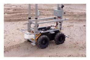
Figure 2.12: Field testing of RTC-I: Tailings sand surface characterization.
