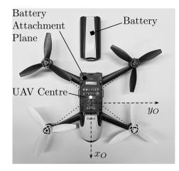
Figure 4.23: Location of UAV centre reference point. Frame O origin is located under and forward.
