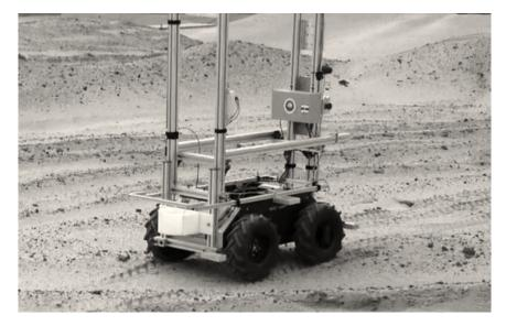
Figure 5.4: RTC-I conducting terramechanics experiments on dry tailings sand.
