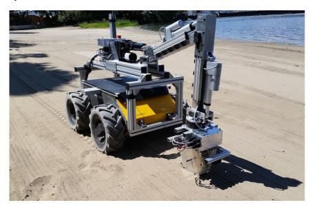
Figure 5.5: Robot manipulator mounted on a UGV.
