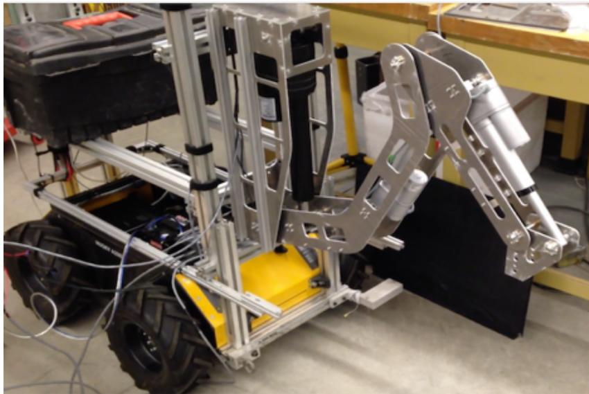
Figure 5.7: Robotic manipulator prototype for laboratory testing.
