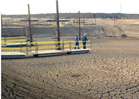
Figure 2.2: Floating dock on a tailings treatment test cell with two workers collecting samples.
