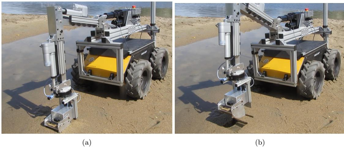
Figure 5.17: RTC-II collecting a sample on saturated sand. (a) The manipulator arm positions the sampler on the terrain and the scoop is closed slowly to collect material. (b) The manipulator lifts the instrument carrying a sample of saturated sand. The soil had sufficient cohesion to maintain the shape of the material collected after the sampler was removed from the ground.
