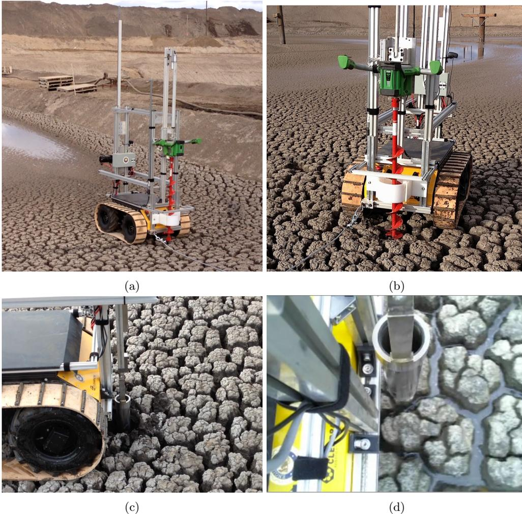
Figure 2.14: (a) RTC-I roving into an experimental cell. (b) Auger and drill subsystem test. (c) Sampler subsystem test. (d) On-board camera's view of the partially dried tailings surface.
