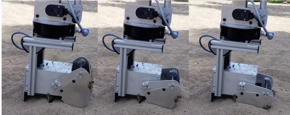
Figure 5.16: Sampler payload collecting a sample on dry sand.
