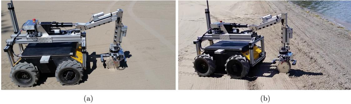
Figure 5.19: RTC-II deploying the instrumented terramechanics wheel on (a) dry sand, (b) transition between dry and wet sand.
