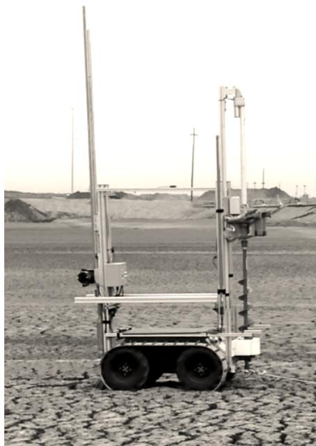
Figure 5.3: RTC-I collecting subsurface samples from an oil sands tailings DDA.
