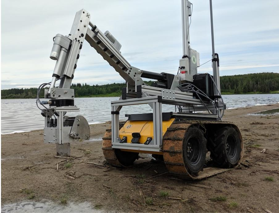
Figure 6.2: RTC-II with scoop sampler attached to the robotic manipulator. The robot is used to collect surface samples for environmental monitoring in mine waste.
