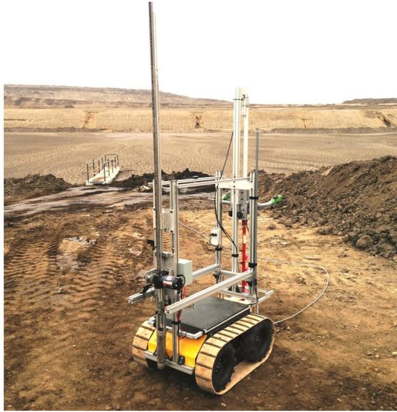
Figure 2.3: Robotic system for tailings characterization.
