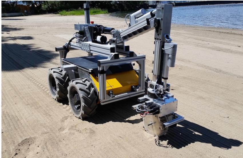
Figure 5.5: Robot manipulator mounted on a UGV.
