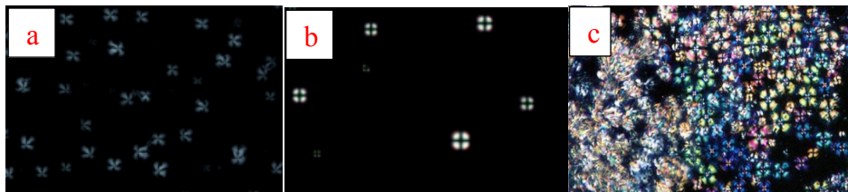
Figure 2-5 Liquid crystals patterns under polarized light: (a) fan-shaped pattern formed by 4'-Pentyl-4-biphenylcarbonitrile droplets sitting on the hydrophilic glass; (b) Maltese cross pattern formed by 4-Pentyl-4-biphenylcarbonitrile droplets sitting on the hydrophobic glass; [27] (c) other patterns formed during phase transition between a nematic (left) and smectic A (right) phases [28].
