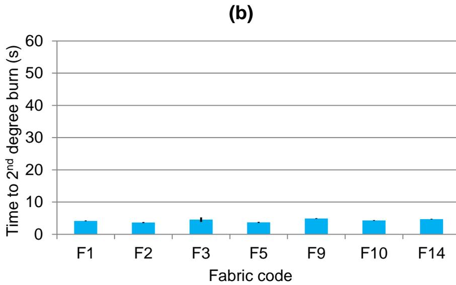
*Figure 4.26 Means ( $\pm$ SEM) of (a) absorbed energy and (b) time to second-degree burn against hot oil for single-layered fabrics*
