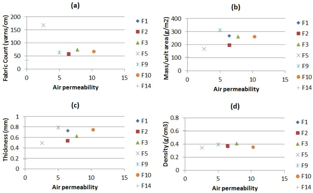
Figure 5.1 Relationship between air permeability and physical properties of fabrics.
