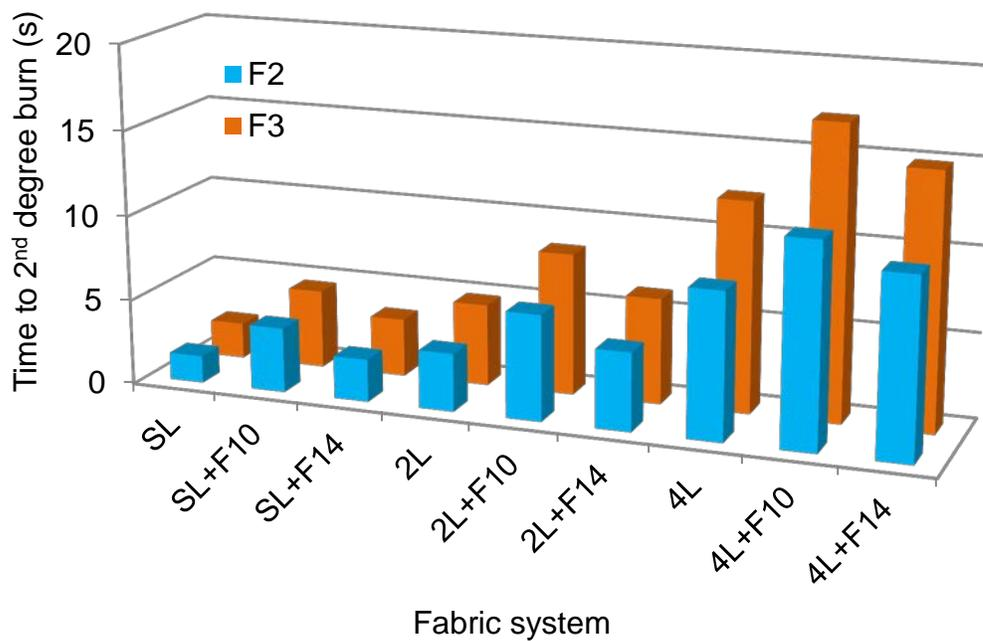
Figure 4.11 Means of time to second-degree burn against hot surface contact for multiple-layer fabrics
