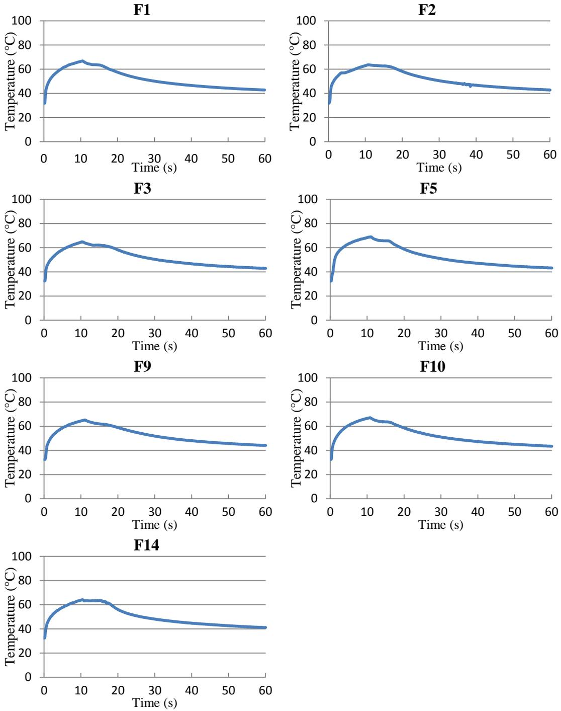
Figure 4.27 Temperature rise over time of single layers during hot oil exposure
