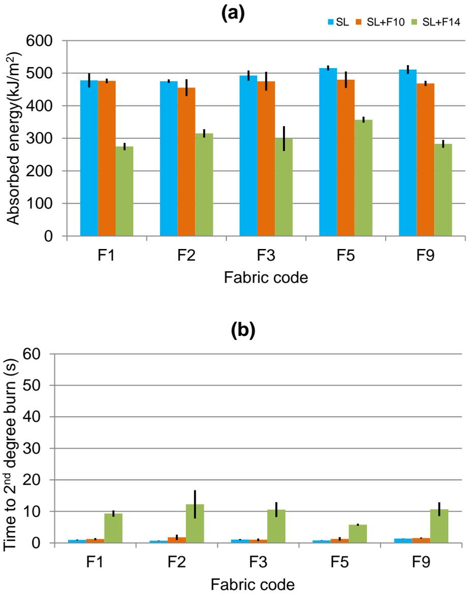
Figure 4.13 Comparison of means ( $\pm$ SEM) of (a) absorbed energy and (b) time to second-degree burn between single-layered fabrics with and without aprons against steam
