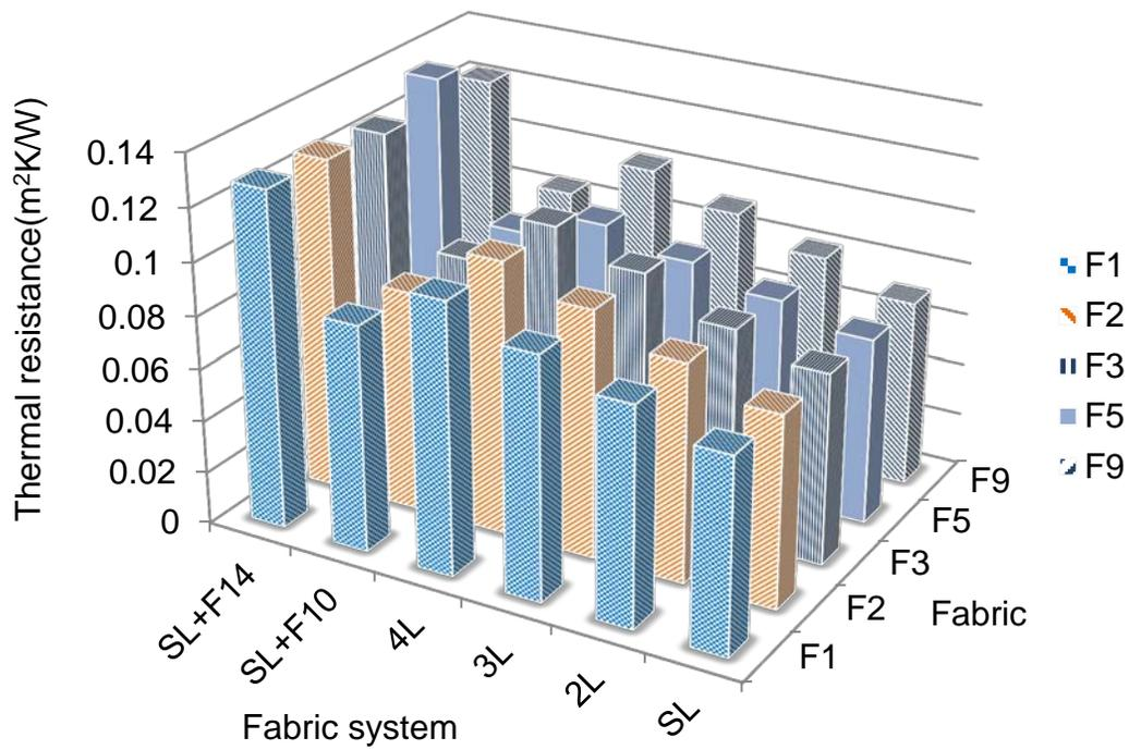
Figure 4.6 Comparison of means of thermal resistance of different fabric systems.
