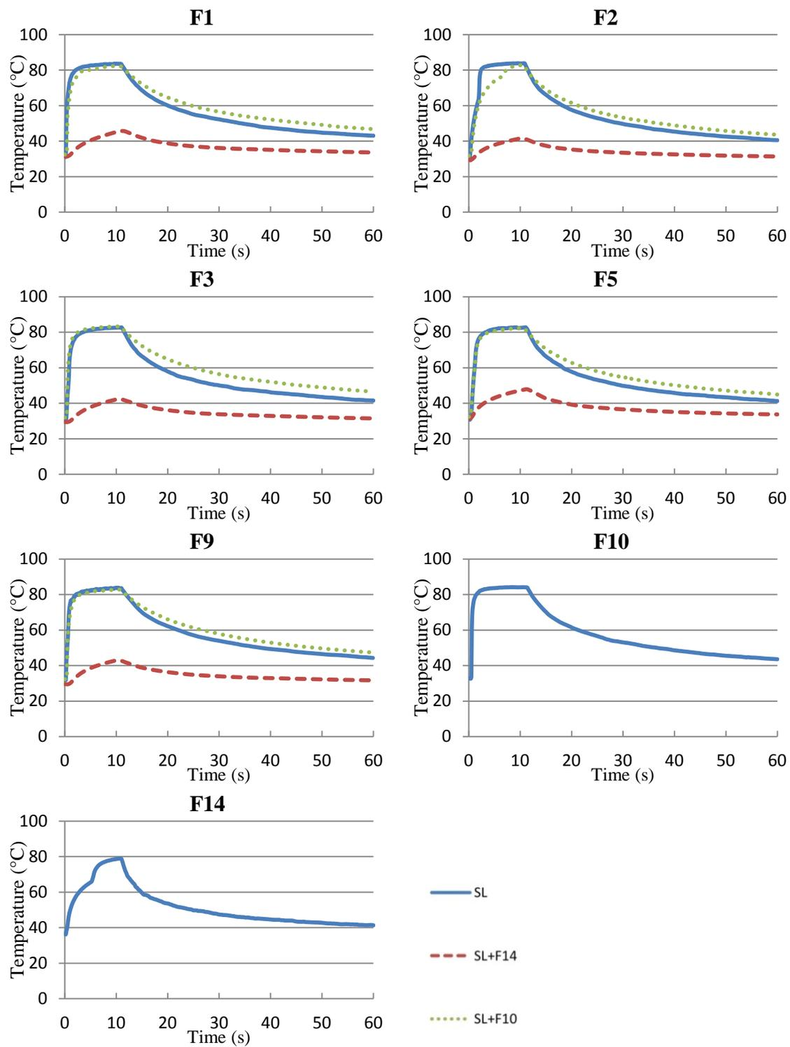
Figure 4.22 Temperature rise over time for single-layered fabrics with and without aprons during hot water tests
