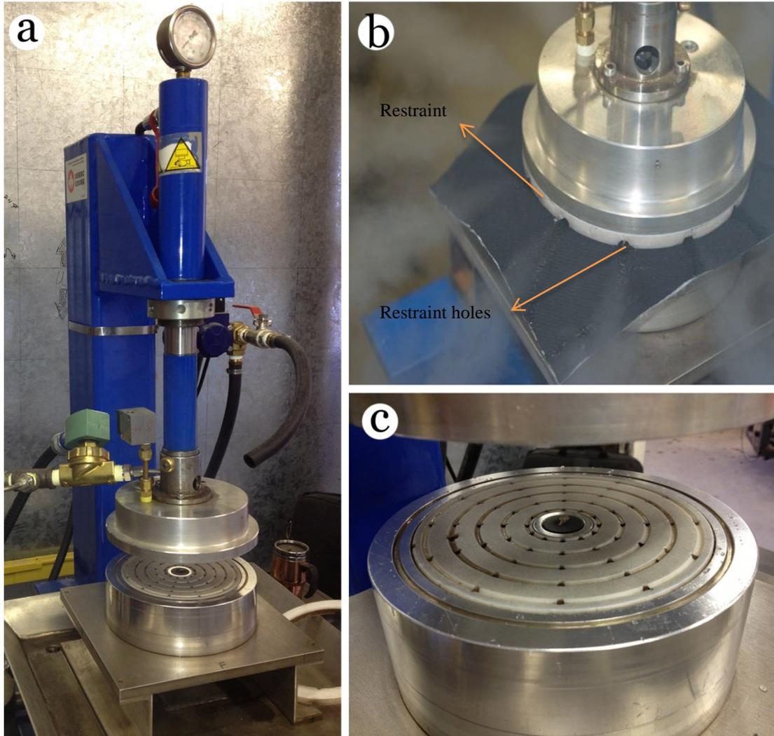
*Figure 2.2 a) Steam resistance test apparatus; b) steam exposure during test; c) sensor and support*
