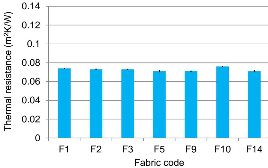
Figure 4.4 Means ( $\pm$ SEM) of thermal resistance of single-layered fabrics
