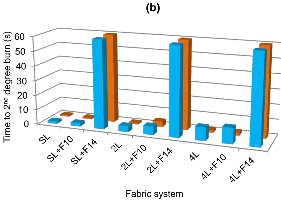
Figure 4.21 Comparison of (a) absorbed energy and (b) time to second-degree burn for multiple-layer fabric systems against hot water
