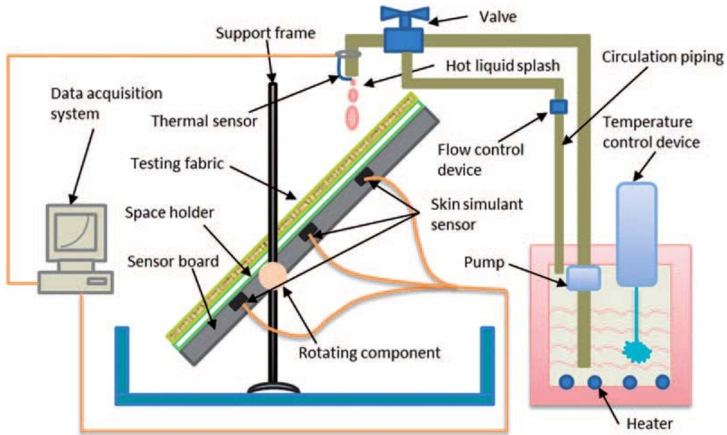
Figure 3.3 Schematic of hot liquid splashes test apparatus (Lu, Song, Ackerman, et al., 2012)
