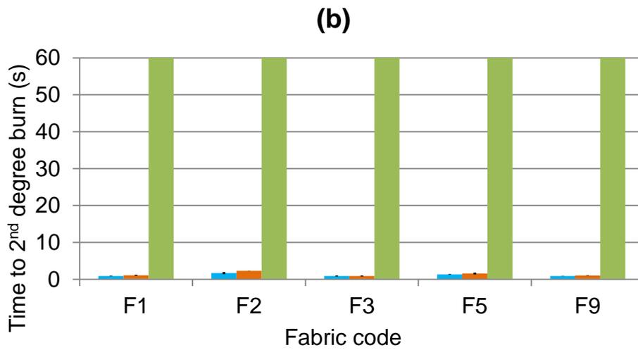
Figure 4.20 Mean ( $\pm$ SEM) of (a) absorbed energy and (b) time to second-degree burn against hot water for single-layered fabrics
