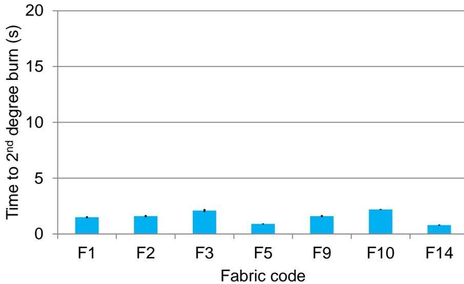
Figure 4.9 Means ( $\pm$ SEM) of time to second-degree burn against hot surface contact for single-layered fabrics.
