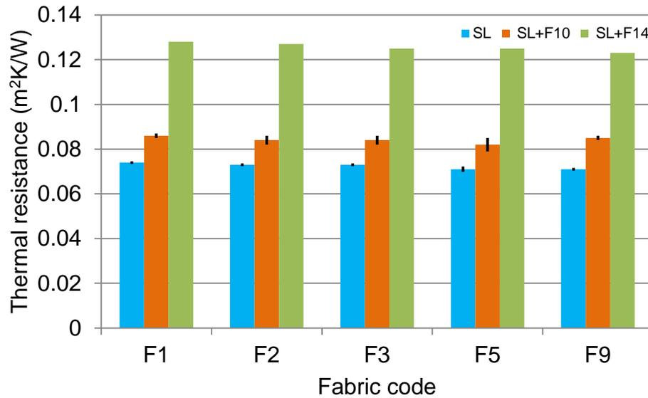
Figure 4.5 Comparison of means ( $\pm$ SEM) of thermal resistance among single-layered fabrics with and without aprons.
