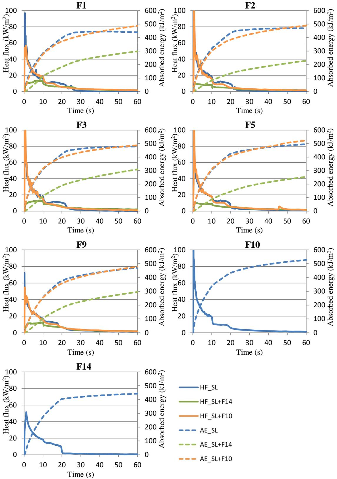
Figure 4.16 Heat flux (HF) and absorbed energy (AE) over time during steam exposure for single layered fabric with and without aprons
