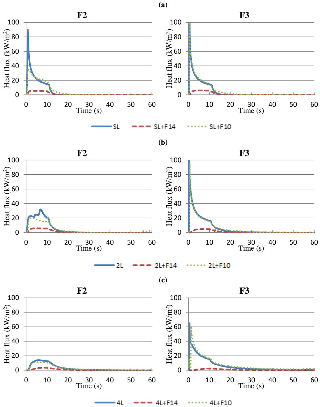
Figure 4.25 Heat flux over time during hot water for F2 and F3 fabric systems a) single layer; b) two layers; c) four layers
