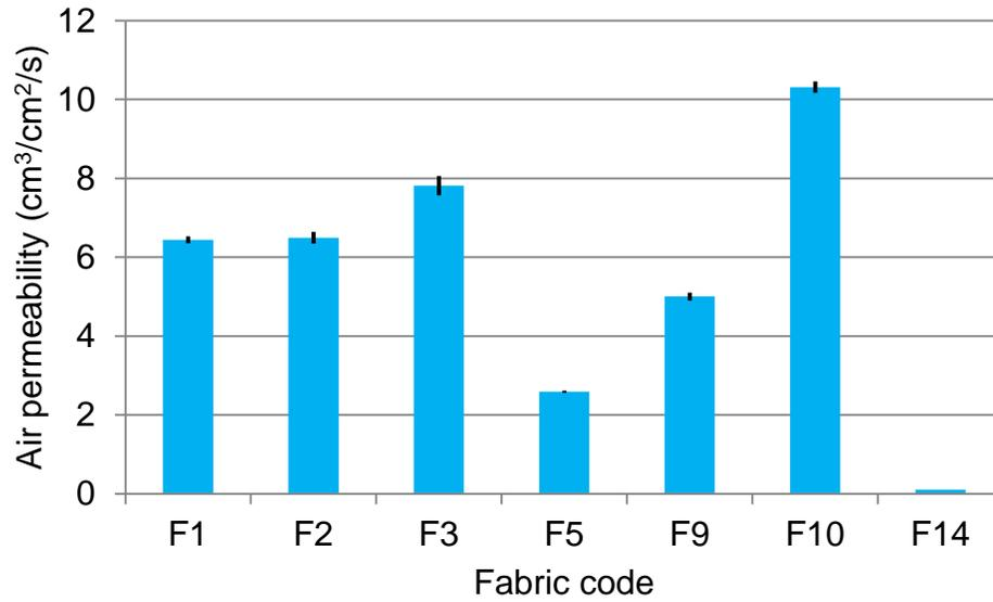
Figure 4.1 Means ( $\pm$ SEM) of air permeability of single-layered fabrics
