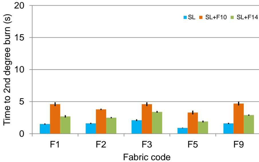
Figure 4.10 Comparison of means ( $\pm$ SEM) of time to second-degree burn against hot surface contact between single-layered fabrics with and without aprons
