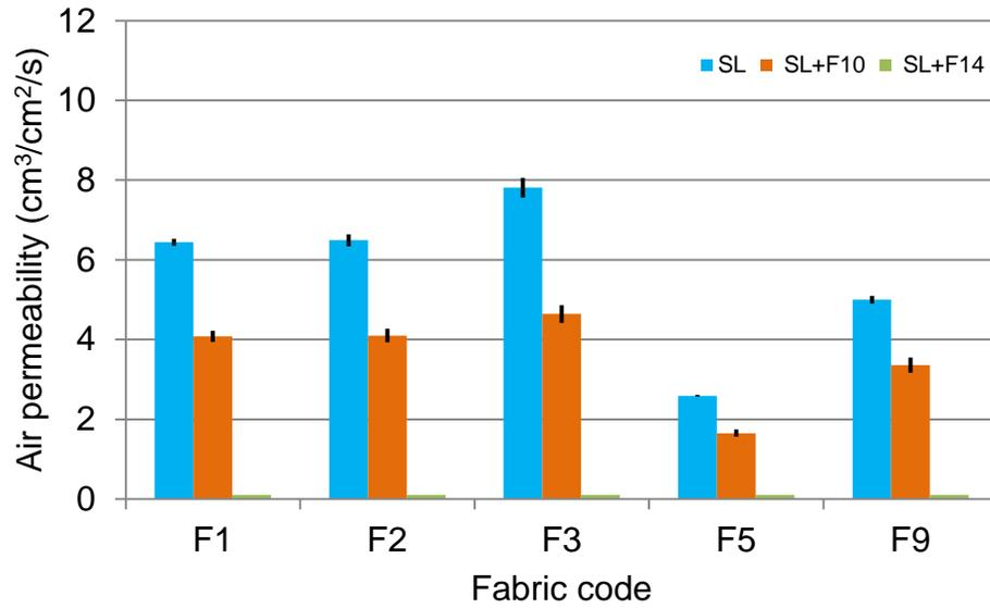
Figure 4.2 Comparison of means ( $\pm$ SEM) of air permeability among single-layered fabrics with and without aprons.
