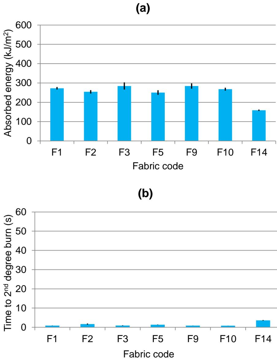
*Figure 4.19 Mean ( $\pm$ SEM) of (a) absorbed energy and (b) time to second-degree burn against hot water for single-layered fabrics*
