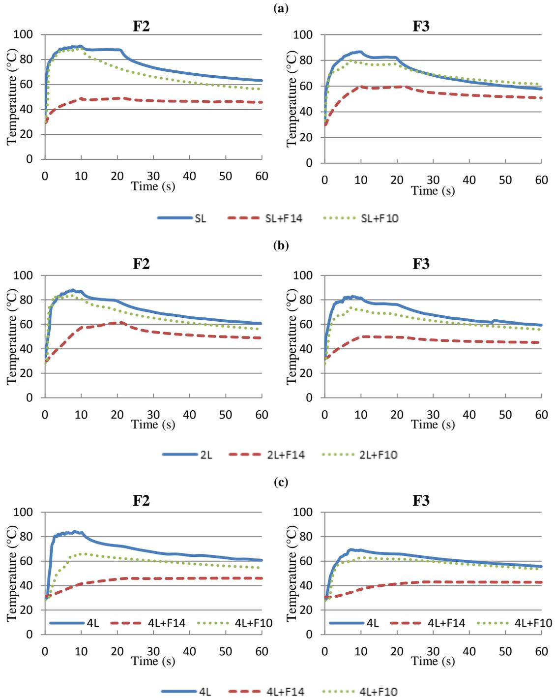
Figure 4.17 Temperature rise over time during steam exposure for F2 and F3 fabric systems a) single layer; b) two layers; c) four layers
