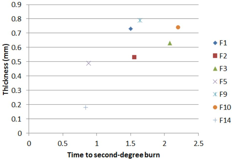
Figure 5.2 Relationship between time to second-degree burn and thickness of fabrics.
