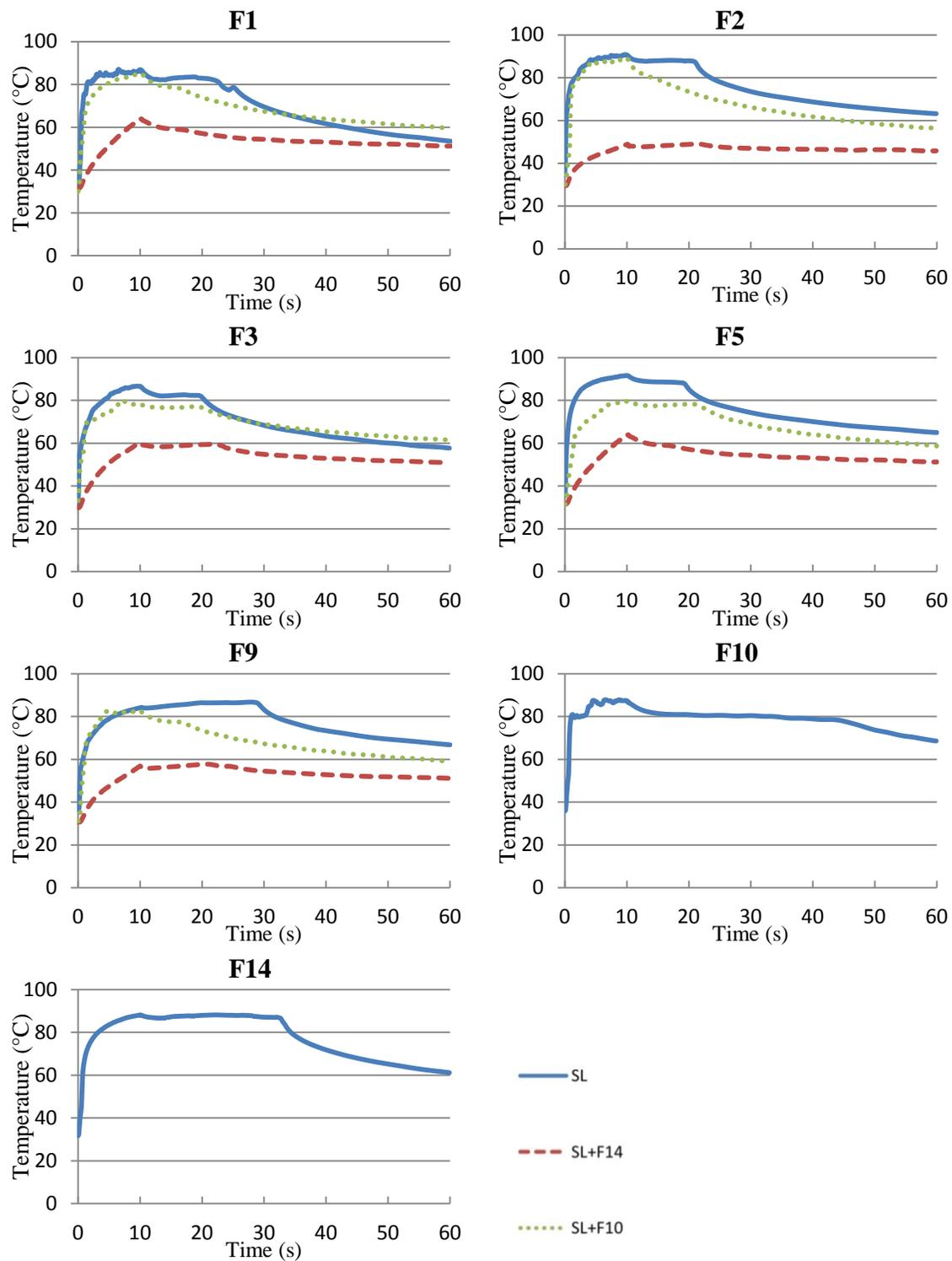
Figure 4.15 Temperature rise over time for single-layered fabrics with and without aprons during steam exposure
