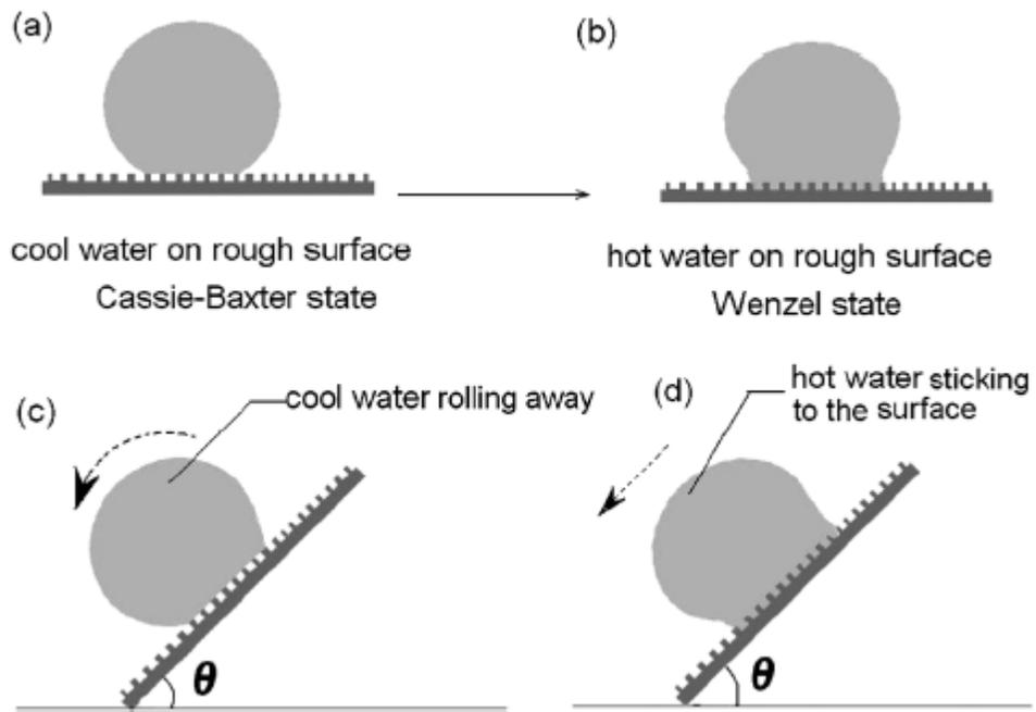
*Figure 2.1 Wetting state of cool water and hot water on rough Teflon surfaces (Liu et al., 2009)*
