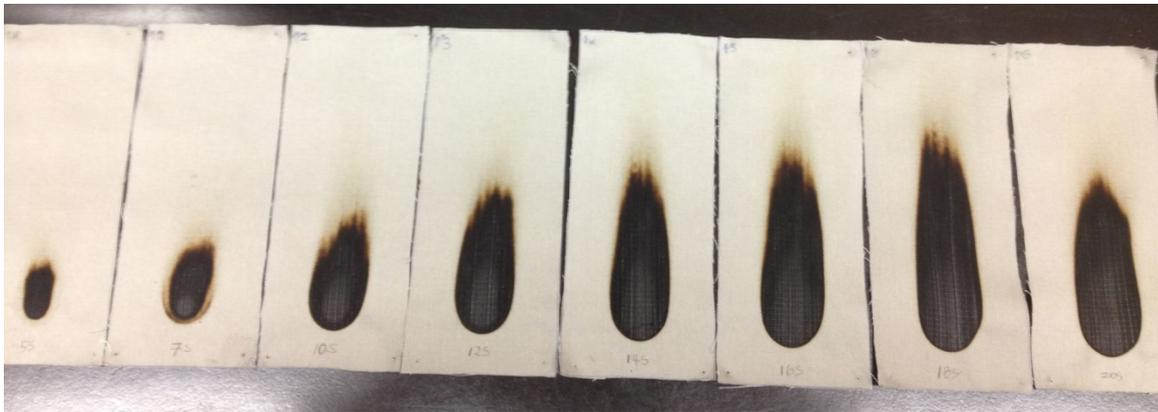
*Figure 4.8 Surface ignition pattern of F1 (FR cotton) specimens. From left to right, the time of applied flame is 5, 7, 10, 12, 14, 16, 18 and 20 seconds, respectively.*
