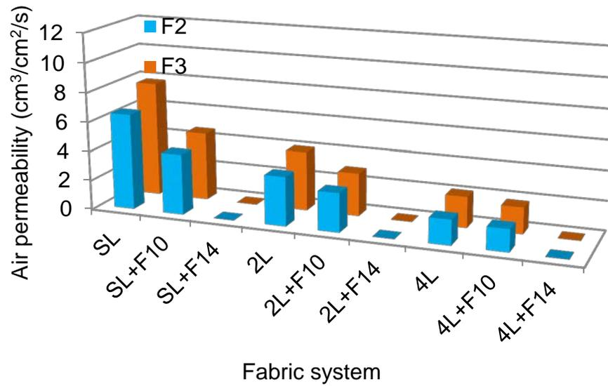
Figure 4.3 Comparison of means of air permeability for multiple-layer fabrics
