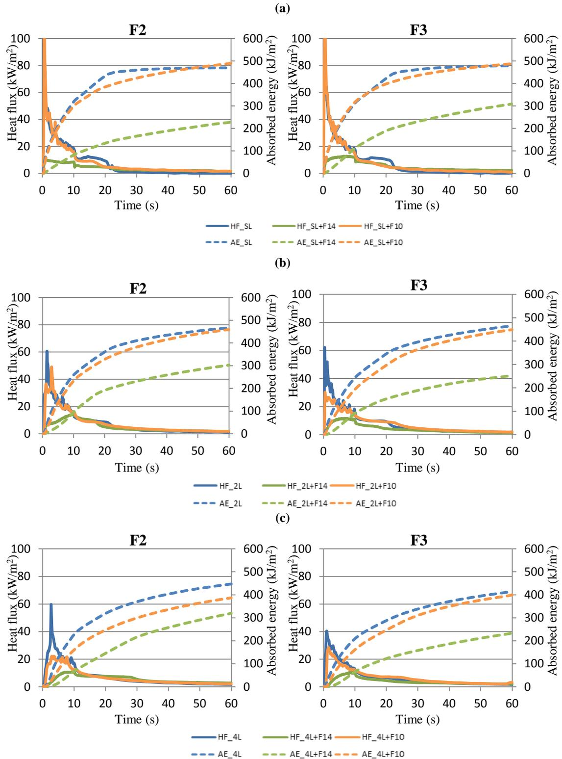
Figure 4.18 Heat flux and absorbed energy over time during steam exposure for multiple-layer fabric system a) single layer; b) two layers; c) four layers
