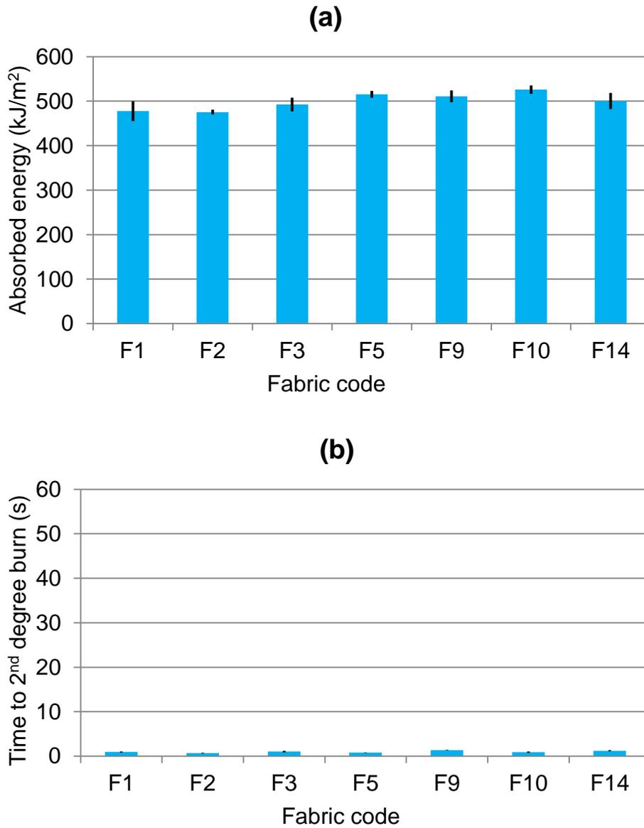
Figure 4.12 Means ( $\pm$ SEM) of (a) absorbed energy and (b) time to second-degree burn of single-layered fabrics against steam at 10 Psi,  $108\pm 5^{\circ}\text{C}$
