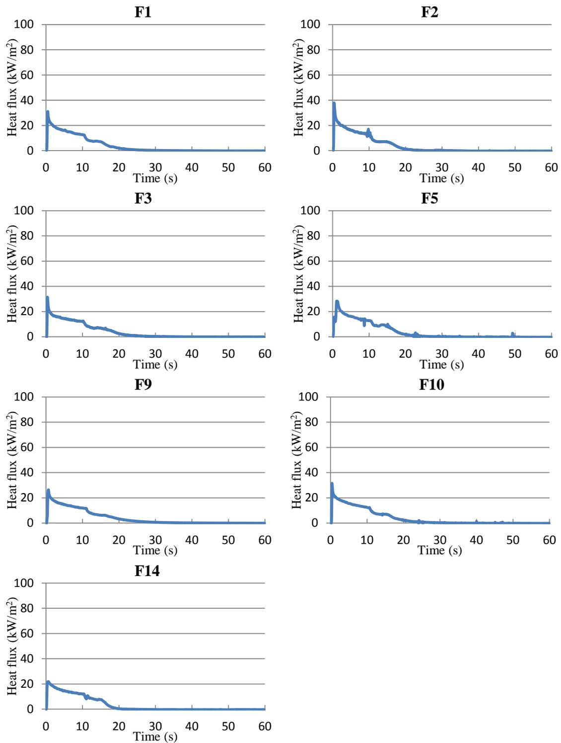
Figure 4.28 Heat flux over time of single layers during hot oil exposure
