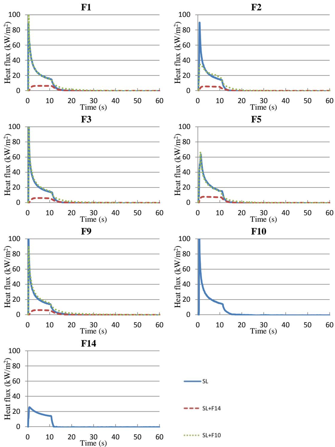
Figure 4.23 Heat flux over time of single-layered fabrics with and without aprons during hot water test
