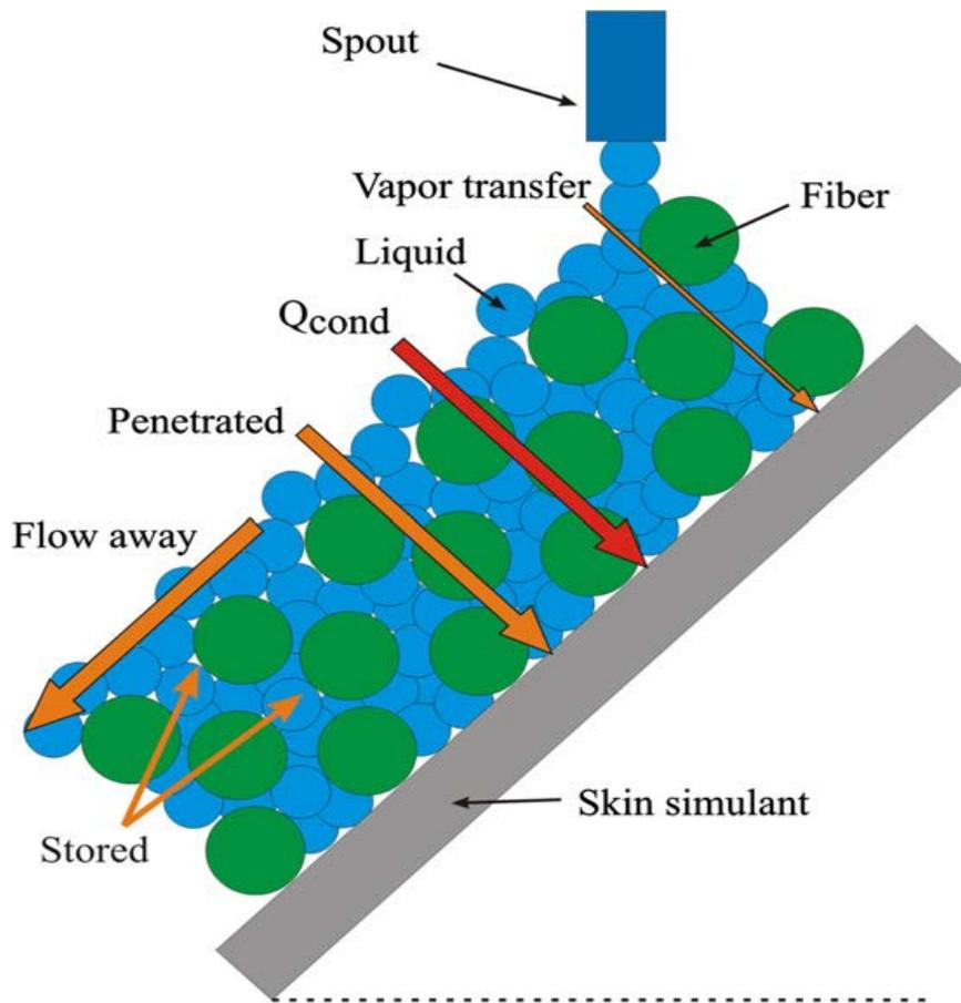
Figure 5.3 Heat and mass transfer in fabric during hot liquid exposure (Lu, Song, Ackerman, et al., 2012)
