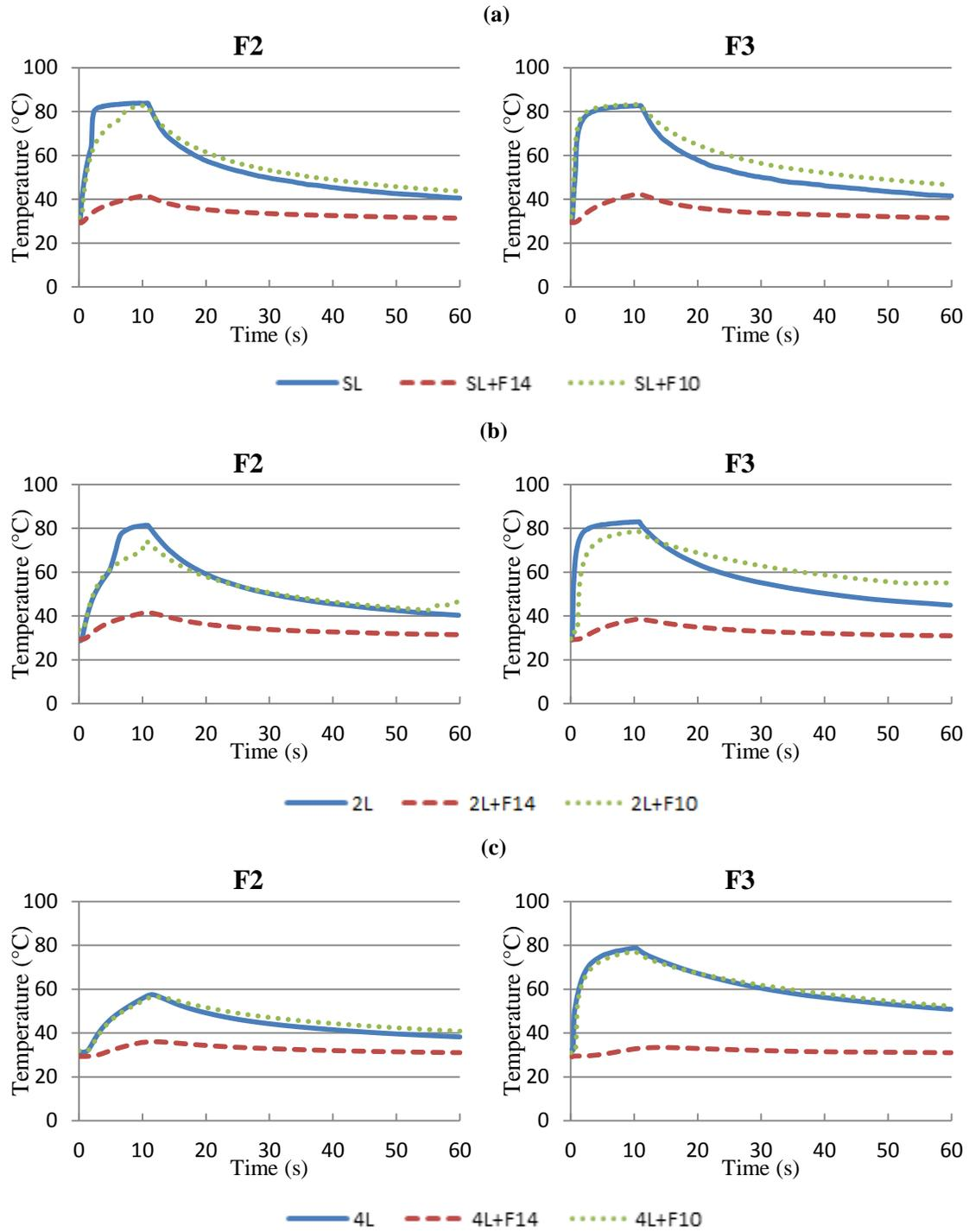
Figure 4.24 Temperature rise over time during hot water for F2 and F3 fabric systems a) single layer; b) two layers; c) four layers
