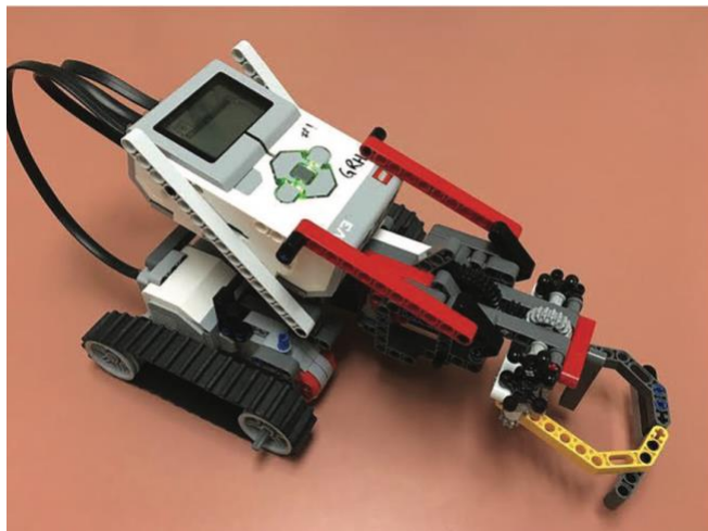
Figure 1. Lego Mindstorms robot with a gripper to grasp objects that were placed on top of blocks.
