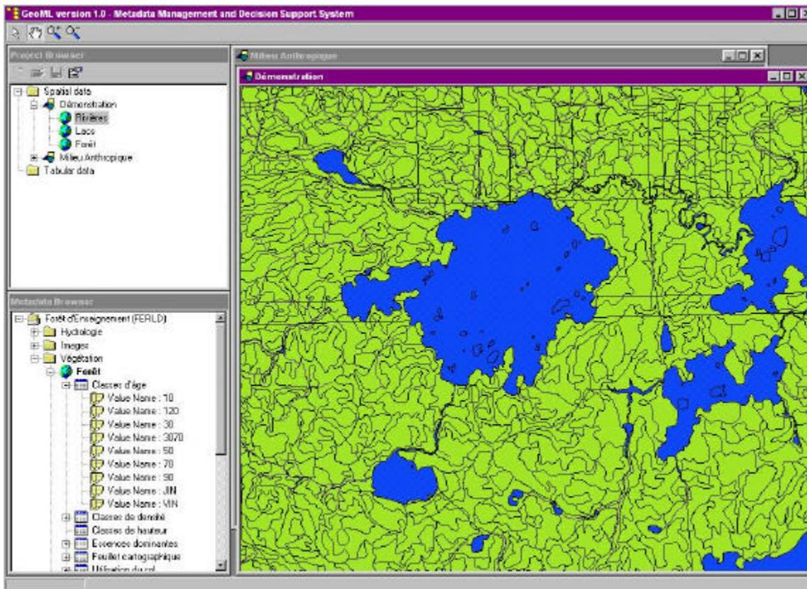
**Figure 3** – Screen capture from the software tool showing the metadata tree (lower left) and a map displayed using MapObjects.
