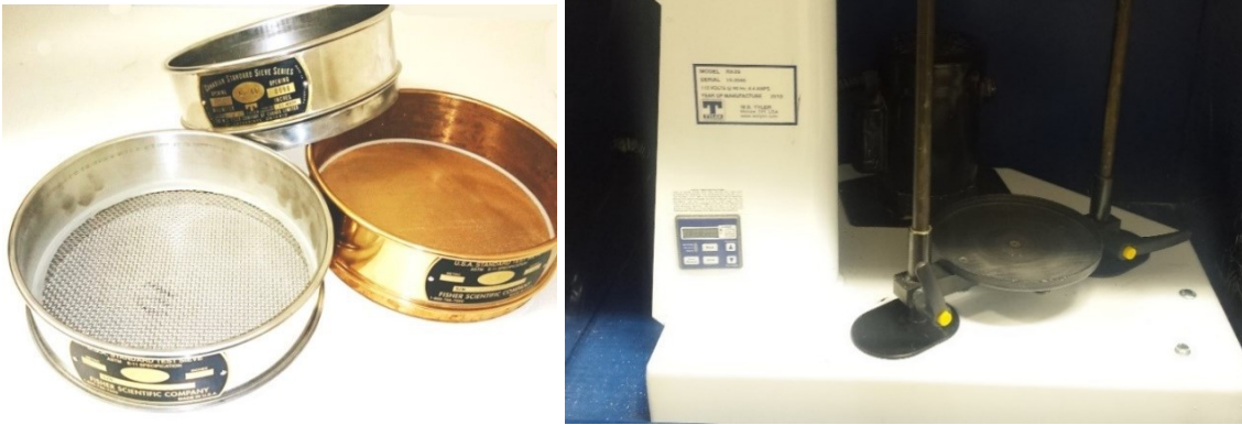
Figure 3-6: (a) ASTM US Sieves (b) Ro-Tap RX-29 mechanical shaker.
