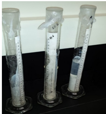
Figure 3-14: Image of a settling suspension progressing to equilibrium and settling columns used for gel point estimation.
