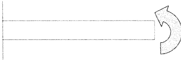
Figure 4.11: Sample loading of a beam used to illustrate geometric nonlinearities.
