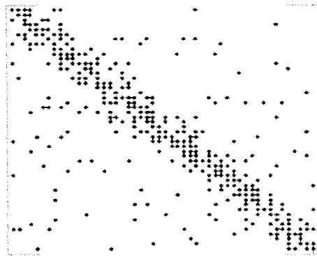
Figure 4.5: Representation of a typical global stiffness matrix. The markers represent the non-zero members.
