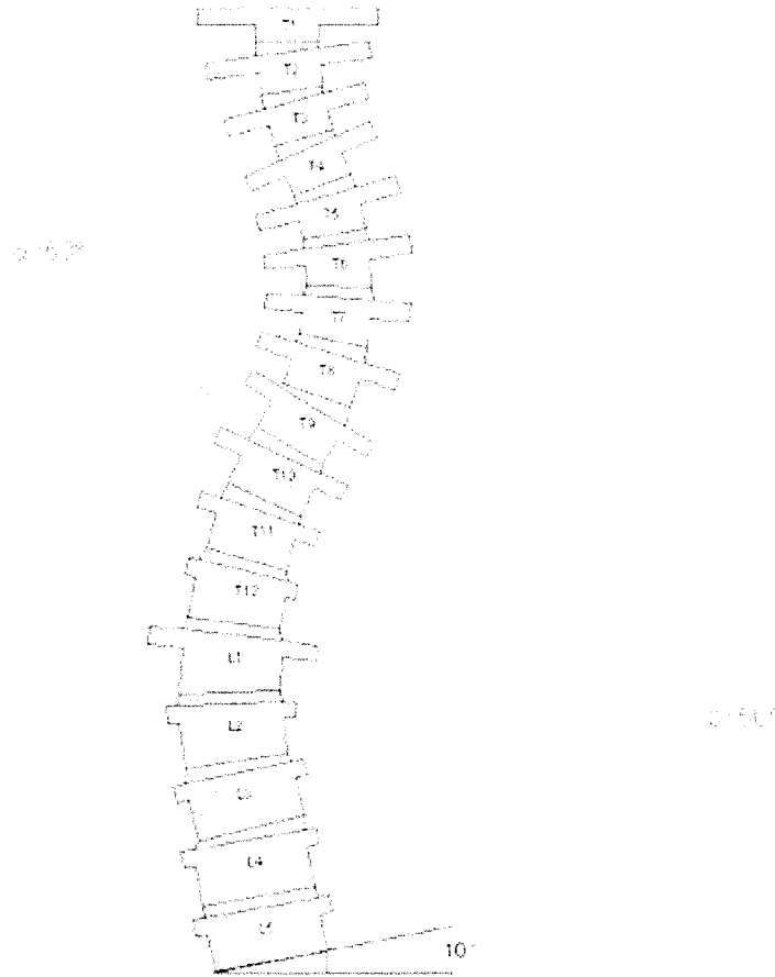
Figure 6.3: Posterior view of the Spinal Model for Cobb angles \alpha = 60^\circ , \beta = 50^\circ , and Lumbar Obliquity, LO = 10^\circ .
