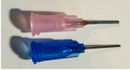
Figure S3.2 Needle tip geometries, Pink 20G, Blue 22G
