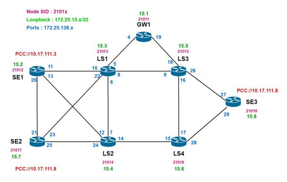
Figure 5-3 Network IP and SID details
