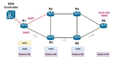
Figure 2-5 Segments determined by controller
