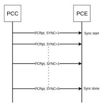
Figure 5-8 LSP State Synchronization.
