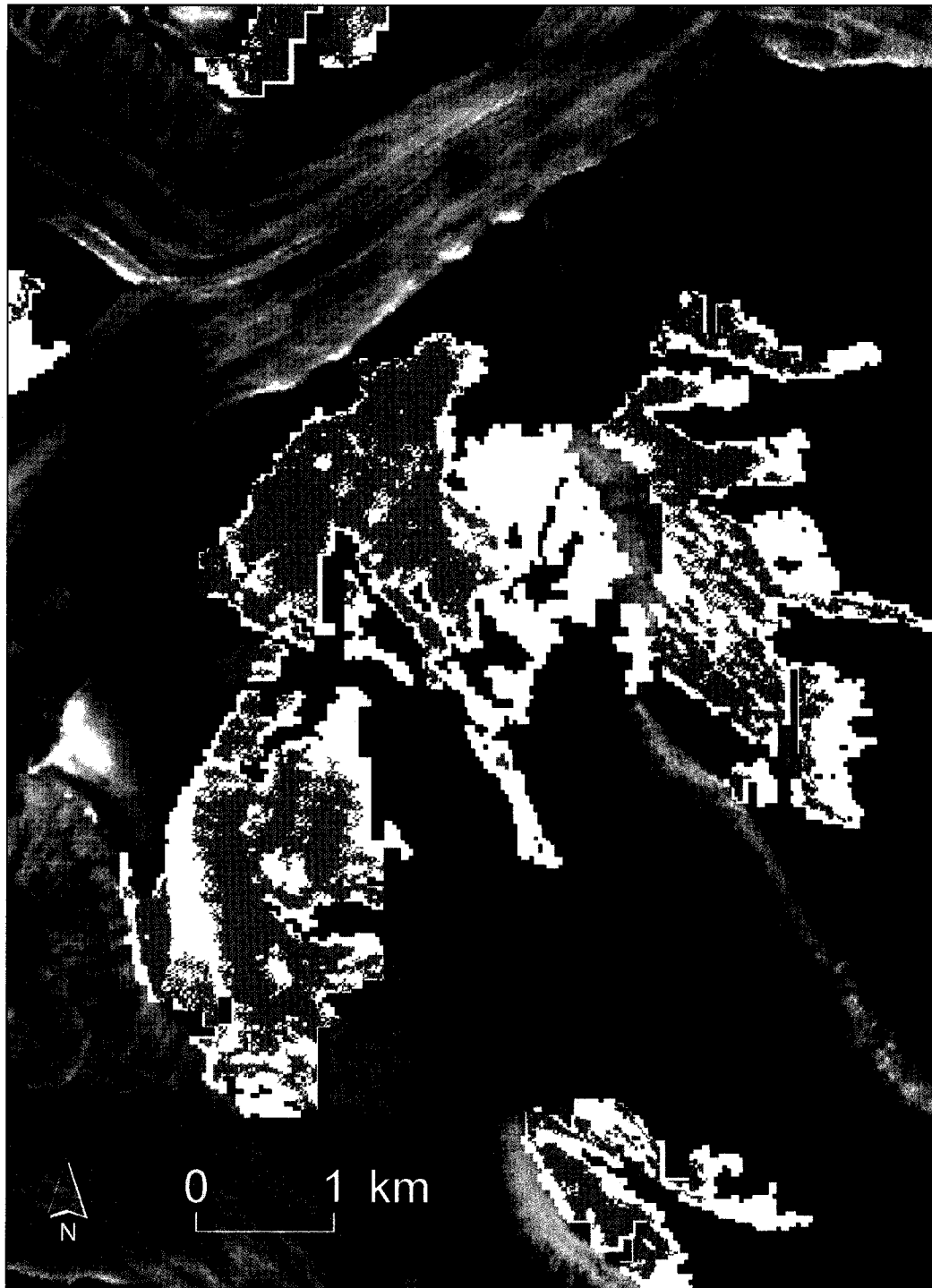
Figure 3. 7 ASTER (dark grey) and ETM+ (light grey) supervised classifications in topographically complex terrain. ASTER's superior spatial resolution (15 m) achieves higher accuracies in areas such as this, where broad diffuse trimlines delineate the former perennial ice cover. ETM+ results show an over classification of the recently deglaciated LIA ice cover relative to the ASTER classification.
