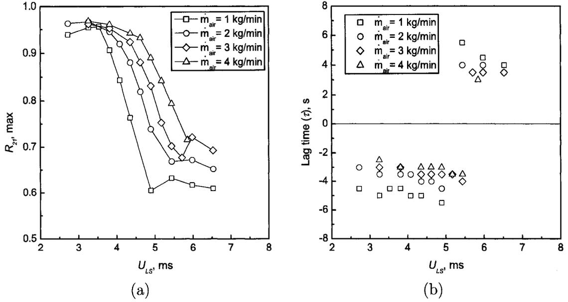
Figure 4.11: (a) Maximum normalized cross-correlation and (b) mean lag time, between signals sampled at the middle of the conduit and just upstream the nozzle ( $R_{21}$ ), as function of liquid superficial velocity, for the standard configuration.
