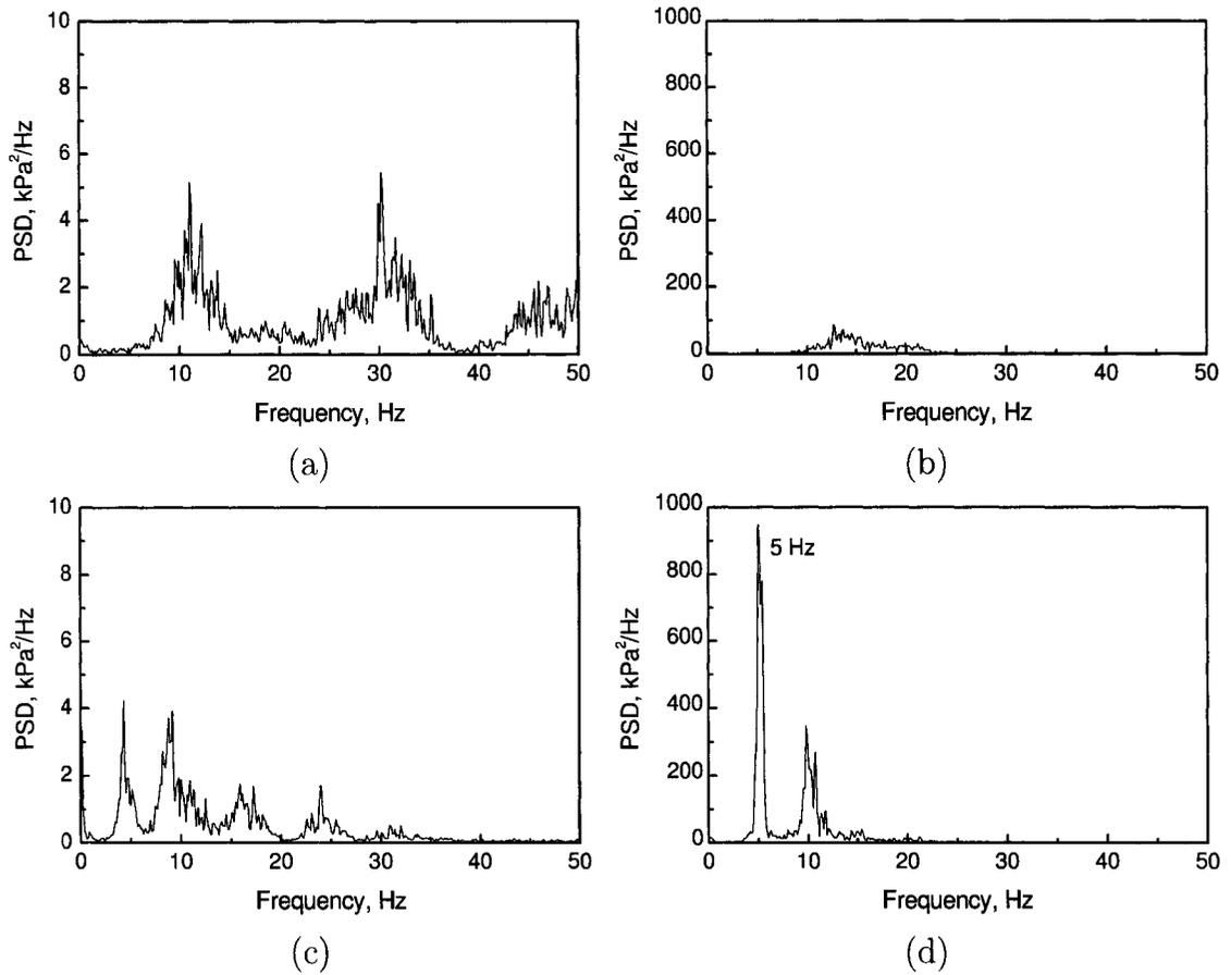
Figure 5.7: PSD of the pressure fluctuation signal for stable (left) and unstable (right) conditions with the short (top) and long (bottom) conduit. Flow rates at 2 kg/min of air and 151.4 and 75.7 kg/min of water, for the stable and unstable condition, respectively.
