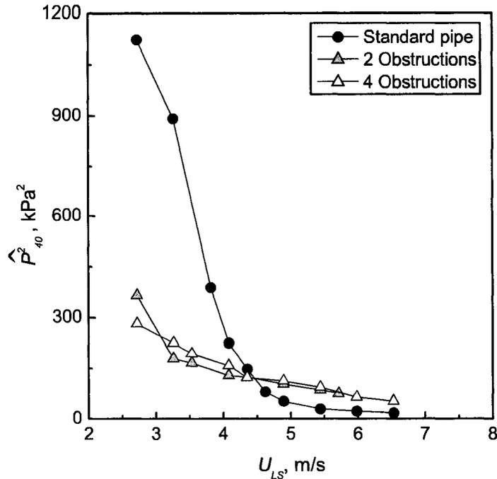
Figure 5.15: Comparison of 2 and 4 peripheral obstructions with the standard pipe for 2 kg/min of air flow.
