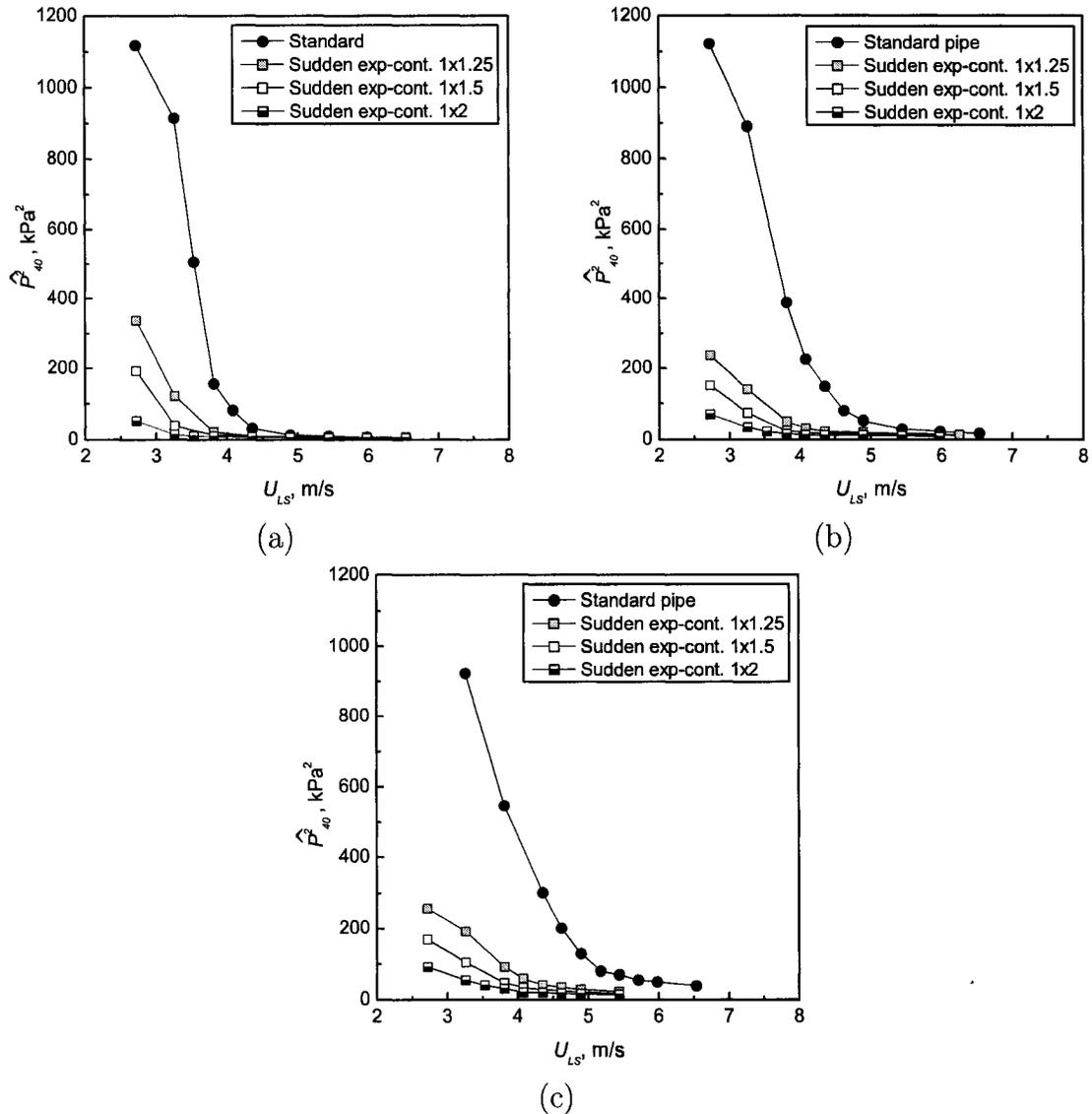
Figure 5.10: Comparison of the different sudden expansion-contractions with the standard pipe for (a) 1 kg/min, (b) 2 kg/min, and (c) 3 kg/min of air flow.
