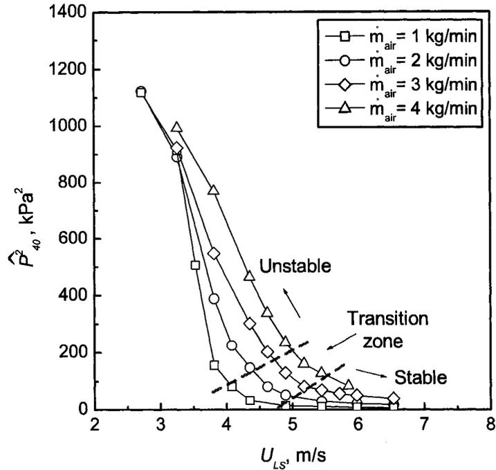
Figure 4.15: Area beneath the PSD for frequencies below 40 Hz, of the pressure fluctuation signal sampled just upstream of the nozzle, as function of liquid superficial velocity, for the standard configuration. Each curve corresponds to a constant air flow rate.
