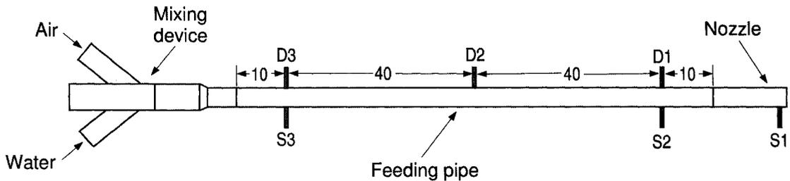
Figure 3.3: Schematic of the standard configuration with pressure transducers along the pipe. Dimensions shown in cm.
