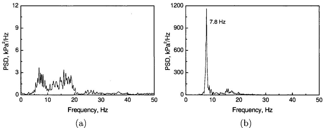
Figure 4.13: PSD of the pressure fluctuation signal sampled just upstream of the nozzle for (a) a stable (2 kg/min of air and 151.4 kg/min of water), and (b) an unstable (2 kg/min of air and 75.7 kg/min of water) condition. Note different scales in (a) and (b).
