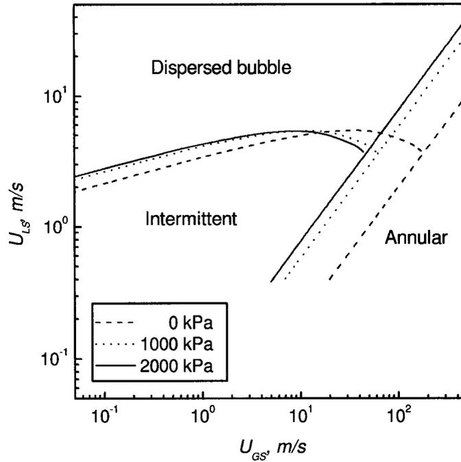
Figure 2.2: Flow pattern map based on the model by Taitel and Dukler (1976) with gas and liquid superficial velocities as coordinates. Air and water as fluids at 20°C, 2.43 cm ID pipe, and different operating pressures. The transition from intermittent to annular flow is the one modified by Barnea et al. (1982).
