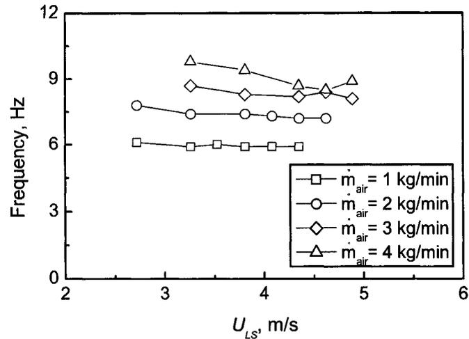
Figure 5.2: Frequency of pulsation for unstable conditions as function of the liquid superficial velocity for the standard feeding pipe.
