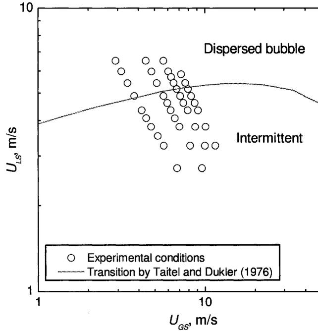
Figure 3.8: Flow map with the experimental conditions for the evaluation of the standard configuration. The dispersed bubble - intermittent transition by Taitel and Dukler (1976), is superimposed as reference.
