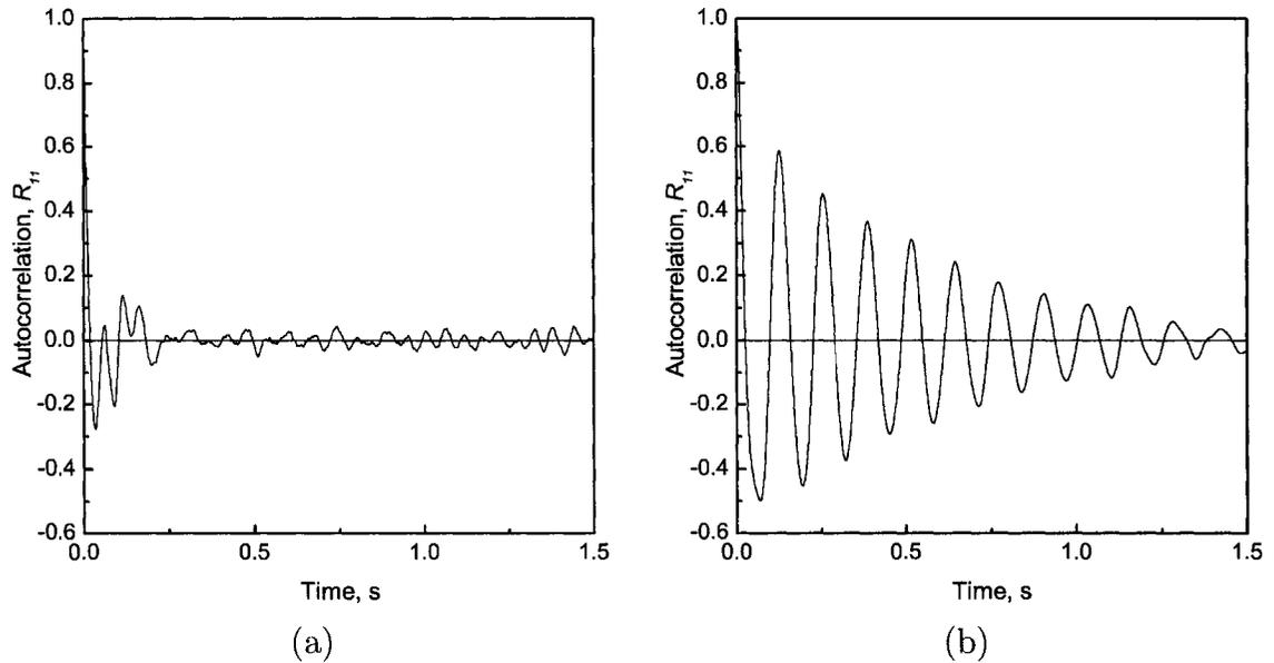
Figure 4.12: Normalized autocorrelation of the pressure fluctuation signal sampled just upstream of the nozzle ( $R_{11}$ ), for (a) a stable (2 kg/min of air and 151.4 kg/min of water), and (b) an unstable (2 kg/min of air and 75.7 kg/min of water) condition.
