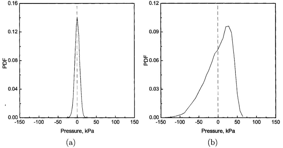
Figure 4.4: Probability density function of the pressure fluctuation signal for (a) a stable (2 kg/min of air and 151.4 kg/min of water) and (b) an unstable (2 kg/min of air and 75.7 kg/min of water) condition.
