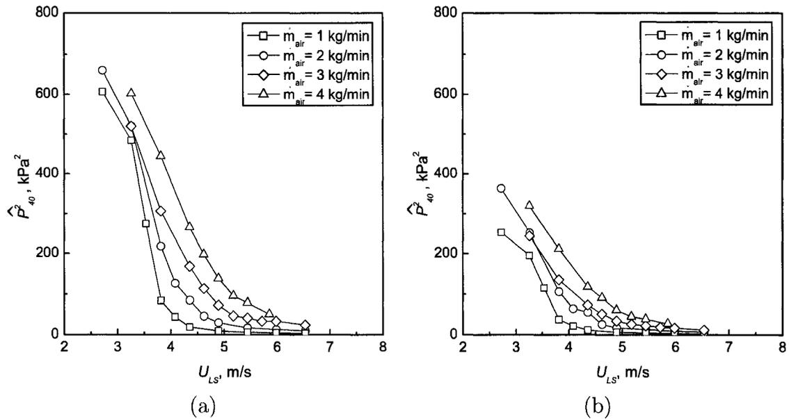
Figure 4.17: Area beneath the PSD for frequencies below 40 Hz of the signals sampled (a) at the middle of the conduit (D2), and (b) after the mixing device, for the standard configuration.
