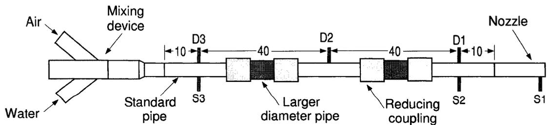
Figure 3.5: Schematic with the set-up for the evaluation of sudden expansion-contractions of the pipe cross-section. Dimensions shown in cm.
