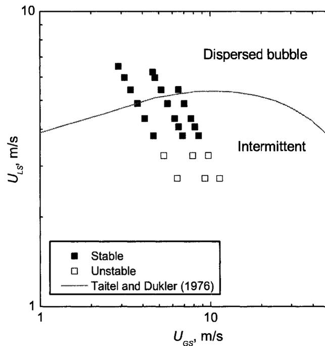
Figure 5.11: Flow map of the operating points with their corresponding stability condition for the 1x1.5 configuration. The transition dispersed bubble–intermittent flow by Taitel and Dukler (1976), is superimposed as reference.
