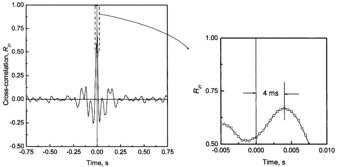
Figure 4.9: Normalized cross-correlation between signals sampled at the middle of the conduit and just upstream of the nozzle ( $R_{21}$ ), for a stable condition (2 kg/min of air and 151.4 kg/min of water).
