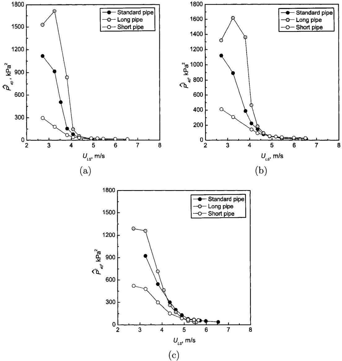
Figure 5.5: Comparison of short and long conduit with respect to the standard, for (a) 1 kg/min, (b) 2 kg/min, and (c) 3 kg/min of air flow.
