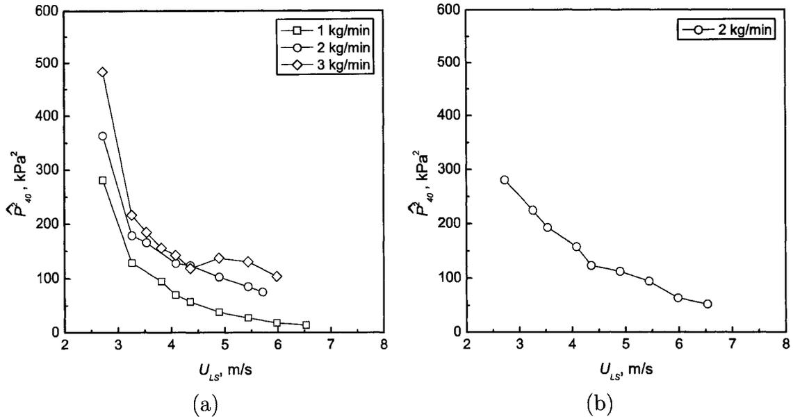
Figure 5.14: Area beneath the PSD for frequencies below 40 Hz ( $\widehat{P}_{40}^2$ ), of the pressure fluctuation signal, for configurations with (a) 2, and (b) 4 peripheral obstructions along the feeding pipe.
