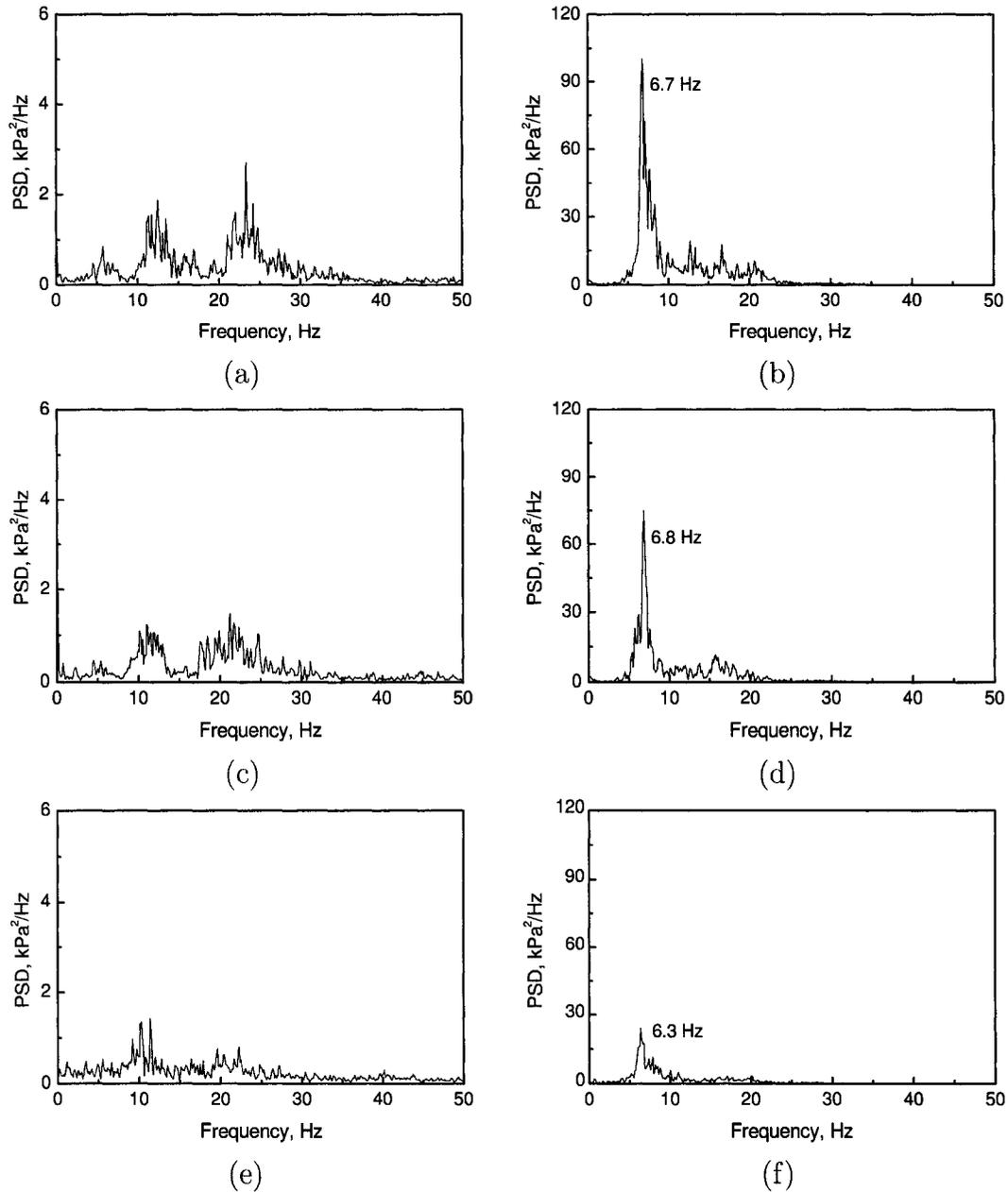
Figure 5.13: PSD of the pressure fluctuation signal for stable (left) and unstable (right) conditions, with the 1x1.25 (top), 1x1.5 (middle) and 1x2 (bottom) configurations. Flow rates at 2 kg/min of air and 151.4 and 75.7 kg/min of water, for the stable and unstable condition, respectively
