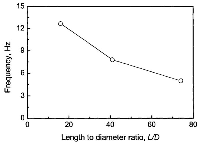
Figure 5.8: Frequency of pulsation as function of the length to diameter ratio ( $L/D$ ) for an unstable condition (2 kg/min of air and 75.7 kg/min of water).
