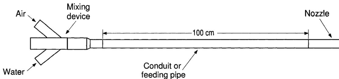
Figure 3.2: Schematic with the arrangement of the nozzle, conduit and mixing device.
