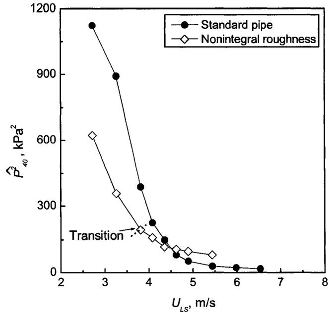
Figure 5.18: Comparison of nonintegral roughness with the standard pipe for 2 kg/min of air flow.
