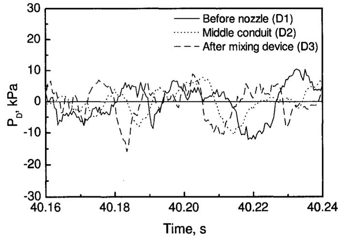
Figure 4.10: Pressure fluctuation signals along the conduit for a stable condition (2 kg/min of air and 151.4 kg/min of water).
