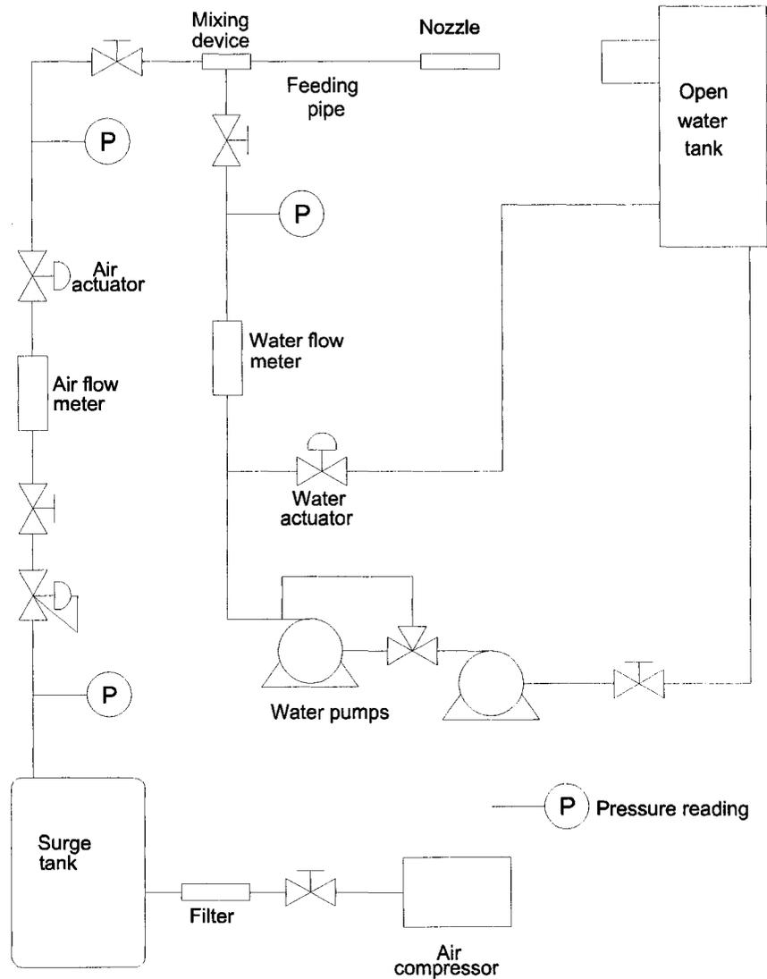
Figure 3.1: Schematic of the commercial-scale spray testing facility at the Syncrude Research Center (Edmonton, Alberta).
