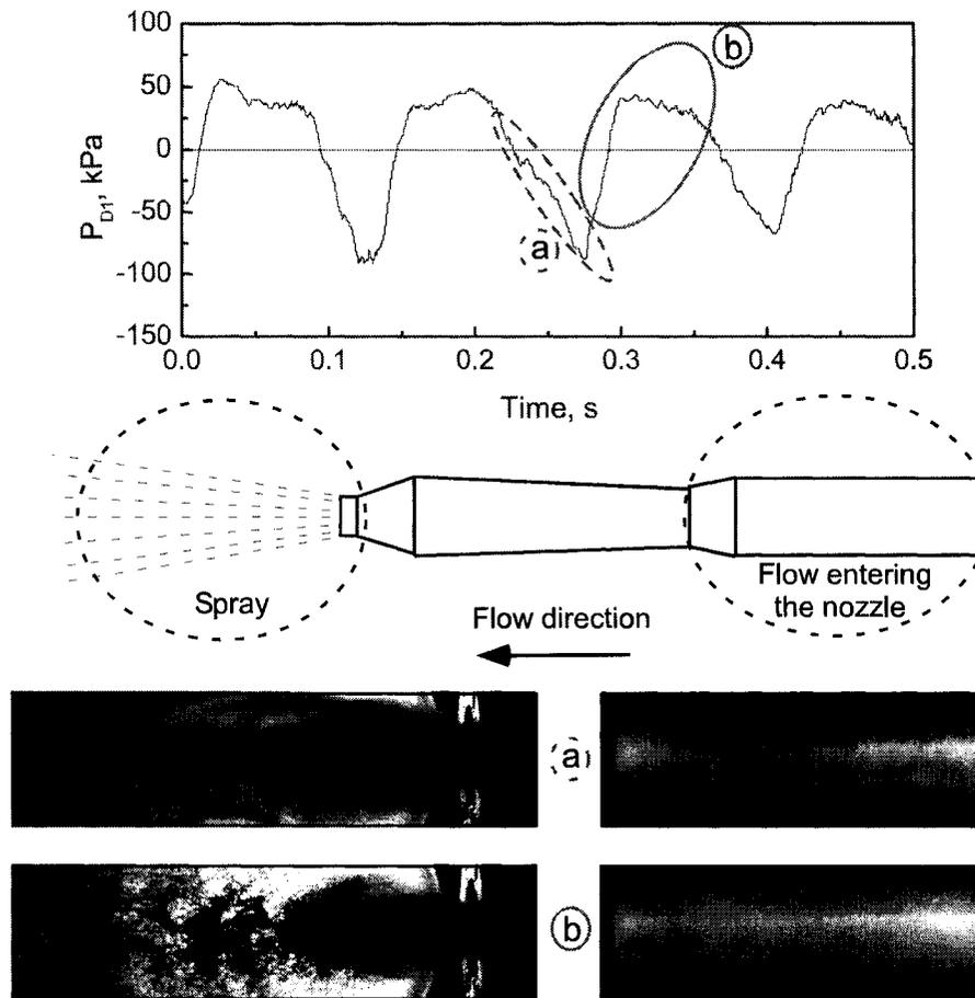
Figure 4.3: Images of the spray and flow in the pipe correlated with the pressure fluctuation signal for an unstable condition (2 kg/min of air and 75.7 kg/min of water). Two main sections were identified: (a) important amounts of gas in the pipe and spray with good droplet dispersion, (b) liquid filling the pipe and spray with ligaments and big droplets.
