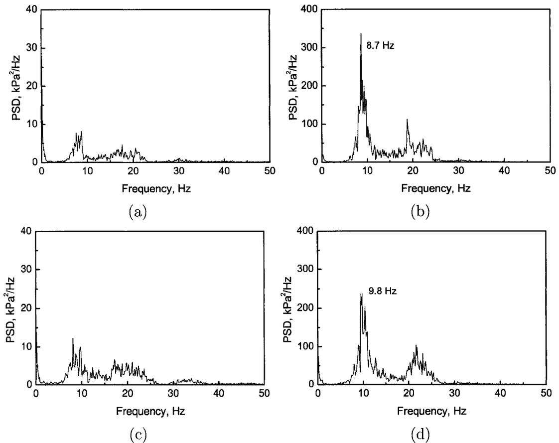
Figure 4.14: PSD of the pressure fluctuation signal sampled just upstream of the nozzle for stable (left) and unstable (right) conditions at 3 kg/min (top) and 4 kg/min (bottom) of air. Water flow rates at (a) 166.6 kg/min, (b) 90.8 kg/min, (c) 162.8 kg/min, and (d) 90.8 kg/min.
