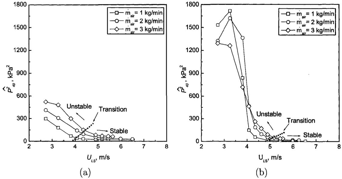
Figure 5.4: Area beneath the PSD for frequencies below 40 Hz ( $\widehat{P}_{40}^2$ ), of the pressure fluctuation signal for the (a) *short*, and (b) *long* conduit.
