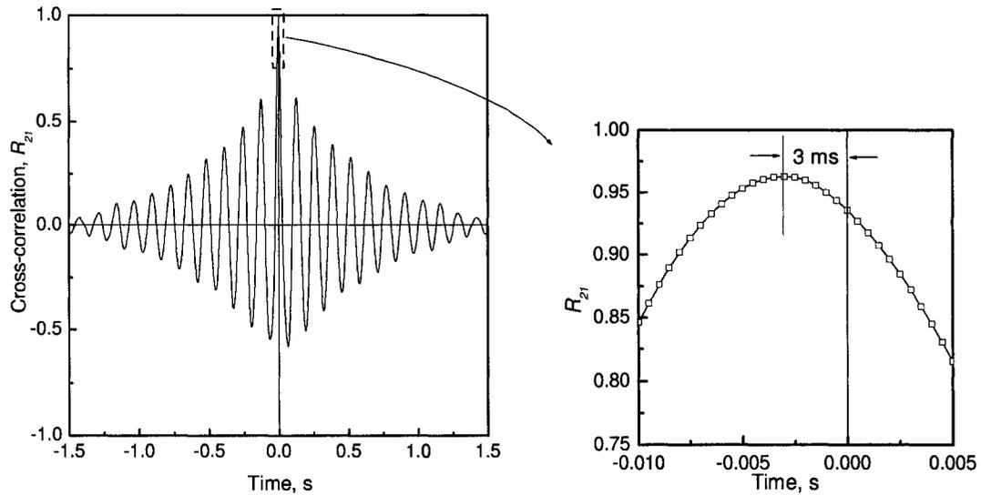
Figure 4.7: Normalized cross-correlation between the signals recorded at the middle of the conduit and just upstream of the nozzle ( $R_{21}$ ), for an unstable condition (2 kg/min of air and 75.7 kg/min of water).
