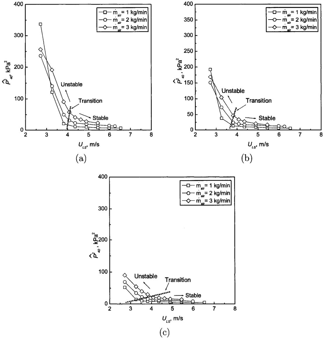
Figure 5.9: Area beneath the PSD for frequencies below 40 Hz ( $\widehat{P}_{40}^2$ ), of the pressure fluctuation signal, for the configurations with sudden expansion-contractions: (a) 1x1.25, (b) 1x1.5, and (c) 1x2.
