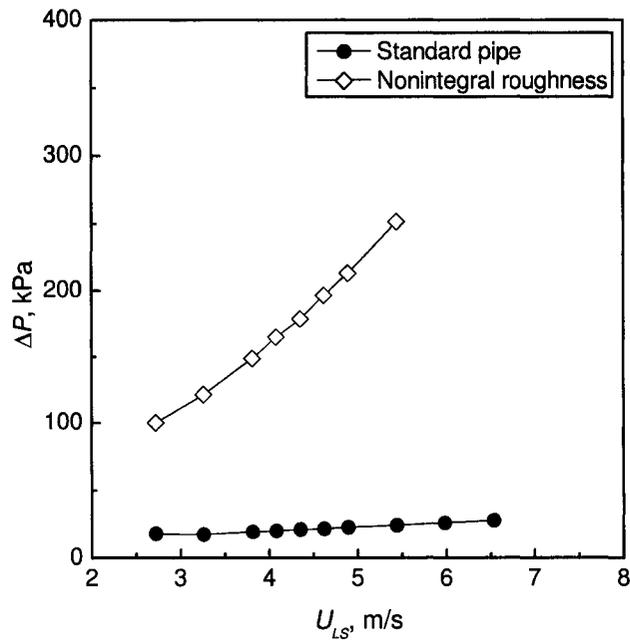
Figure 5.19: Pressure drop along the feeding pipe for the standard and nonintegral roughness configurations.
