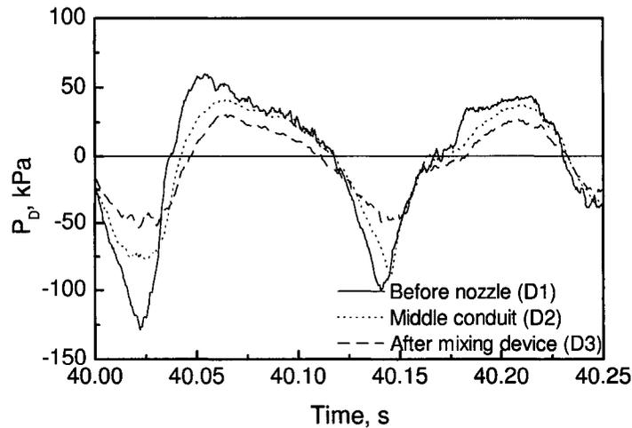
Figure 4.8: Pressure fluctuation signals along the conduit for an unstable condition (2 kg/min of air and 75.7 kg/min of water).
