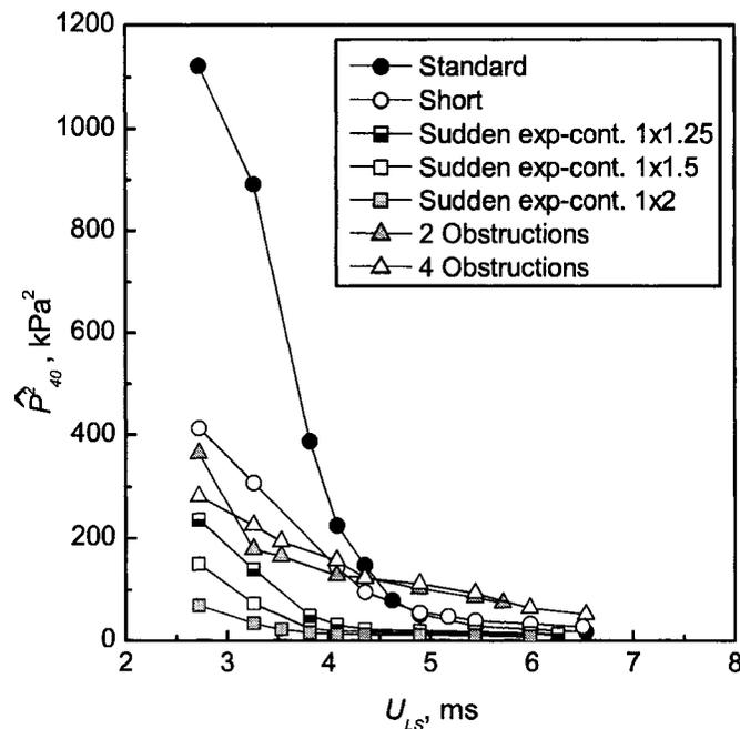
Figure 5.21: Area beneath the PSD for frequencies below 40 Hz ( $\widehat{P}^2_{40}$ ), of the pressure fluctuations, for most of the feeding pipe configurations evaluated at 2 kg/min of air.
