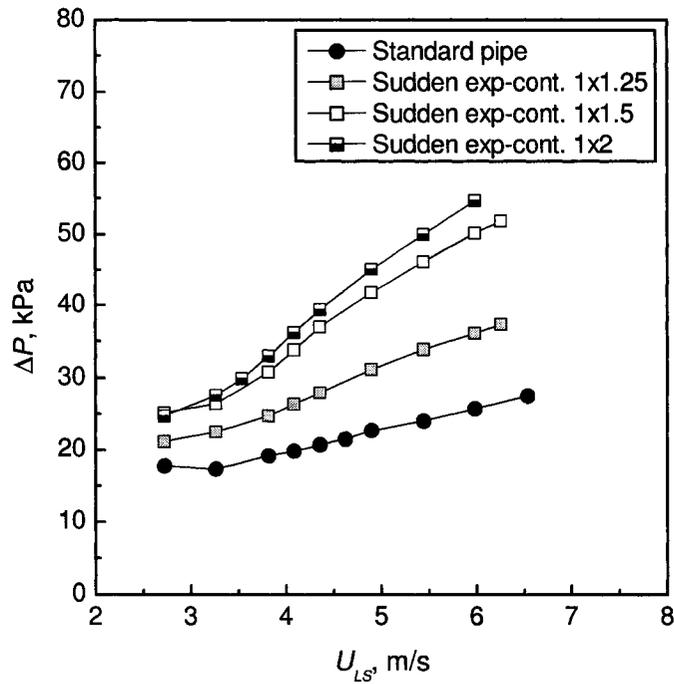
Figure 5.12: Pressure drop along the feeding pipe for the standard and sudden expansion-contractions arrangement.
