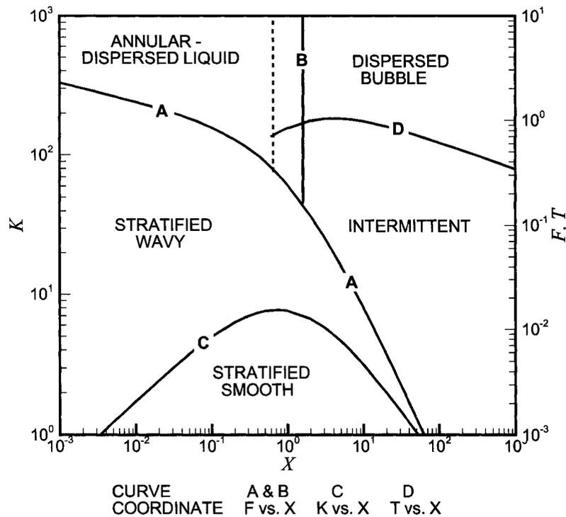
Figure 2.1: Dimensionless flow pattern map based on the model by Taitel and Dukler (1976) to predict flow regime transitions in horizontal gas-liquid flow. The dotted line corresponds to the annular-intermittent transition modified by Barnea et al. (1982).
