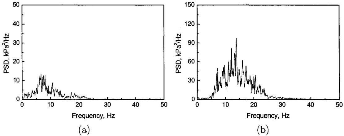
Figure 5.20: PSD of the pressure fluctuation signal for (a) a stable, and (b) an unstable condition, for the configuration with nonintegral roughness. Flow rates at 2 kg/min of air and 151.4 and 75.7 kg/min of water, for the stable and unstable condition, respectively.
