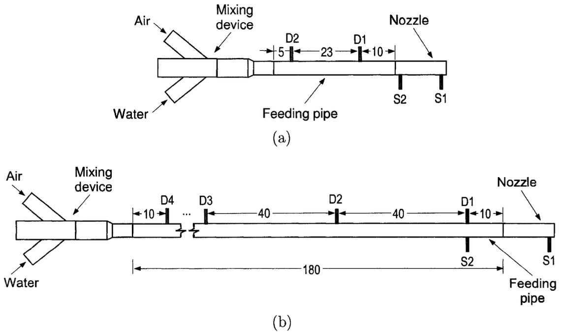
Figure 3.4: Schematic with the set-up for the evaluation of a (a) 38 cm ( $L/D \approx 16$ ), and (b) 180 cm ( $L/D \approx 74$ ) long pipe. Dimensions shown in cm.
