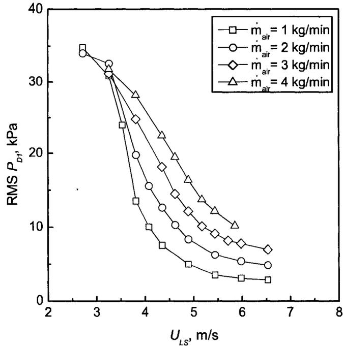
Figure 4.5: Root mean square of the pressure fluctuation signal sampled upstream the nozzle, as function of liquid superficial velocity, for the standard configuration. Each curve corresponds to a constant air flow rate.
