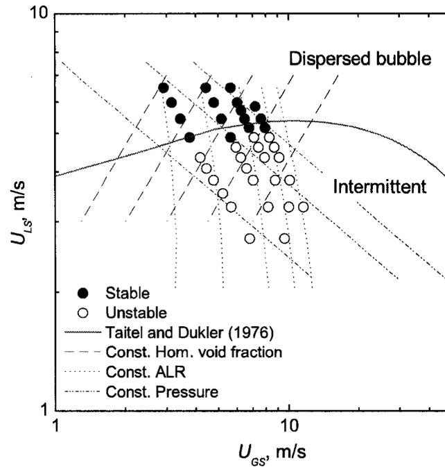
Figure 5.1: Flow map with the operating points and their corresponding stability condition for the standard configuration. The transition dispersed bubble – intermittent flow by Taitel and Dukler (1976) is superimposed as reference.
