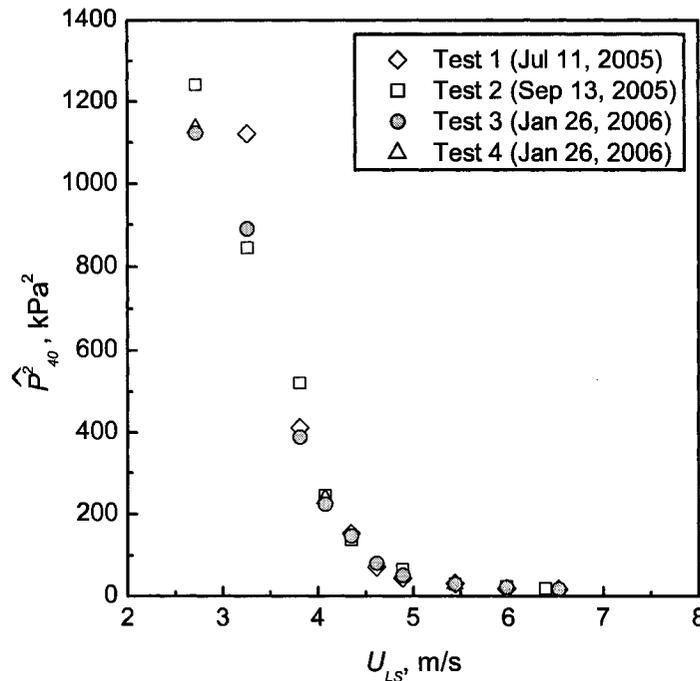
Figure 5.3: Area beneath PSD for frequencies below 40 Hz ( $\hat{P}_{40}^2$ ), for different tests performed with the standard configuration, at 2 kg/min of air.
