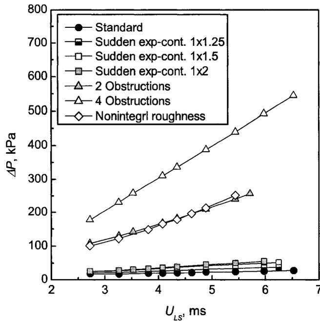
Figure 5.22: Pressure drop along the feeding pipe for configurations improving the gas and liquid mixing along the conduit.
