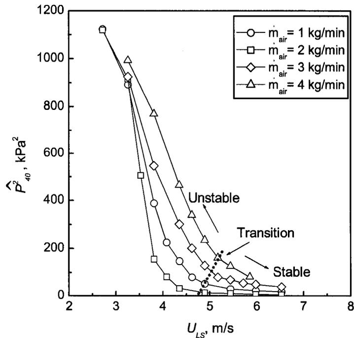
Figure 4.16: Stability transition for the standard configuration, based on the area beneath the PSD for frequencies below 40 Hz ( $\hat{P}_{40}^2$ ), of the pressure fluctuation signal sampled just upstream of the nozzle.
