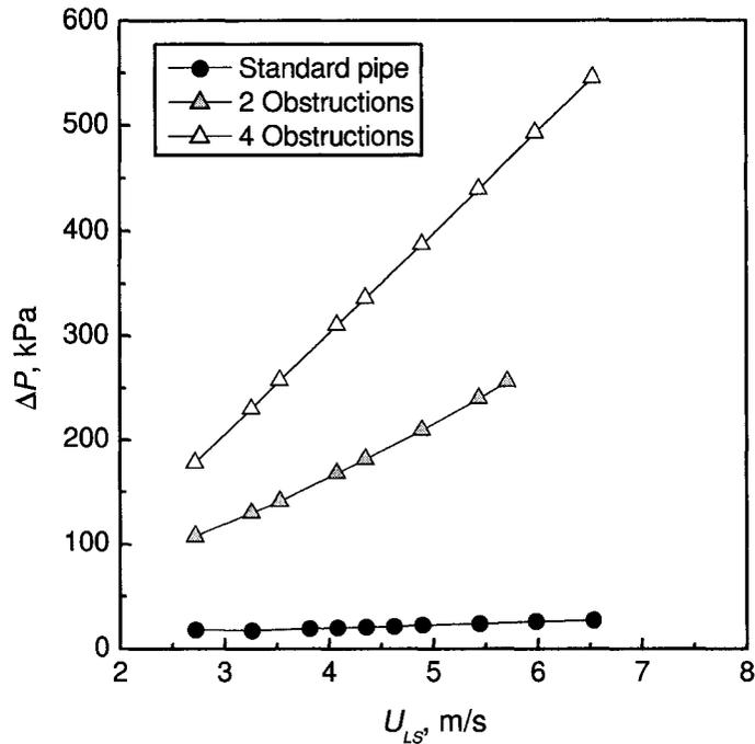
Figure 5.16: Pressure drop along the feeding pipe for the standard conduit and configurations with peripheral obstructions along the pipe.
