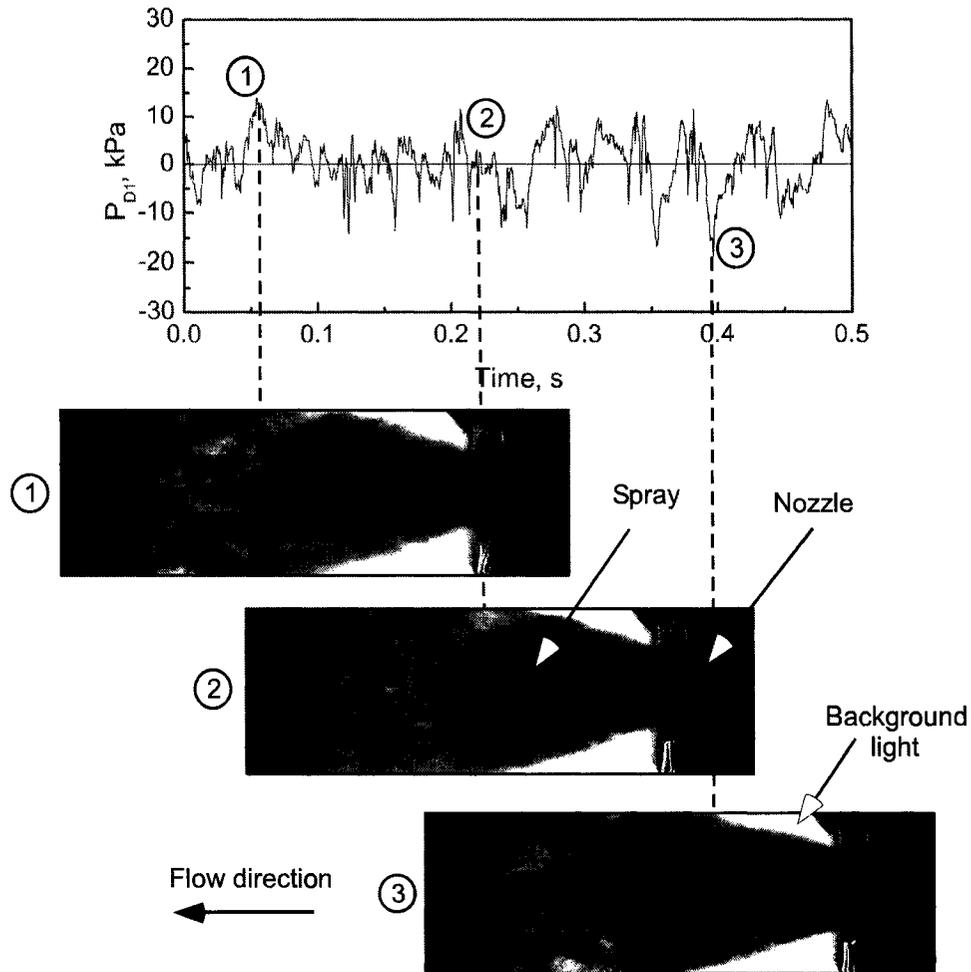
Figure 4.2: Spray pattern at certain points of the pressure fluctuation signal for a stable condition (2 kg/min of air and 151.4 kg/min of water).
