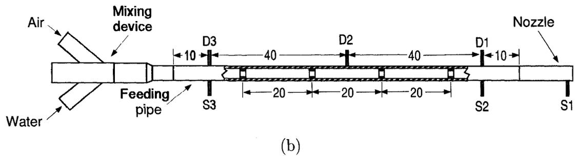
Figure 3.6: Schematic with the set-up for the evaluation of the effect of (a) 2 and (b) 4 peripheral obstructions. Dimensions shown in cm.
