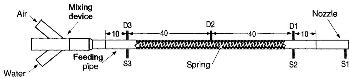
Figure 3.7: Schematic with the set-up for the evaluation of the pipe with nonintegral roughness. Dimensions shown in cm.
