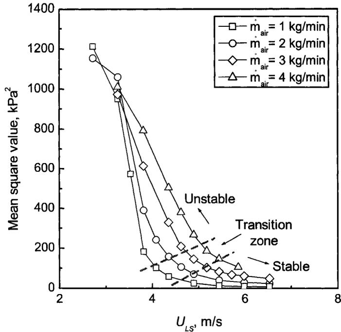
Figure 4.6: Mean square value of the pressure fluctuation signal sampled upstream the nozzle, as function of liquid superficial velocity, for the standard configuration. Each curve corresponds to a constant air flow rate.
