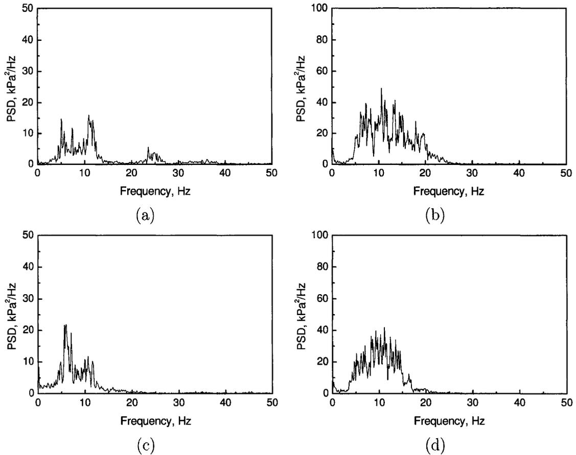
Figure 5.17: PSD of the pressure fluctuation signal for stable (left) and unstable (right) conditions with 2 obstructions (top) and 4 obstructions (bottom) configurations. Flow rates at 2 kg/min of air and 151.4 and 75.7 kg/min of water, for the stable and unstable condition, respectively.
