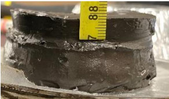
Figure 12. Profile view of centrifuge cake during ambient air-drying with un-even distribution of water content over depth.
