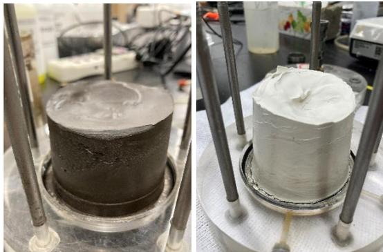
Figure 4. Centrifuge cake (left) and Speswhite Kaolin (right) at the end of the Tempe cell test under an applied matric suction of 400kPa
