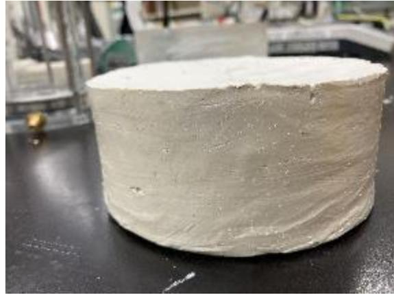
Figure 13. Profile view of air-dried Speswhite kaolin with uniform distribution of water content over depth.
