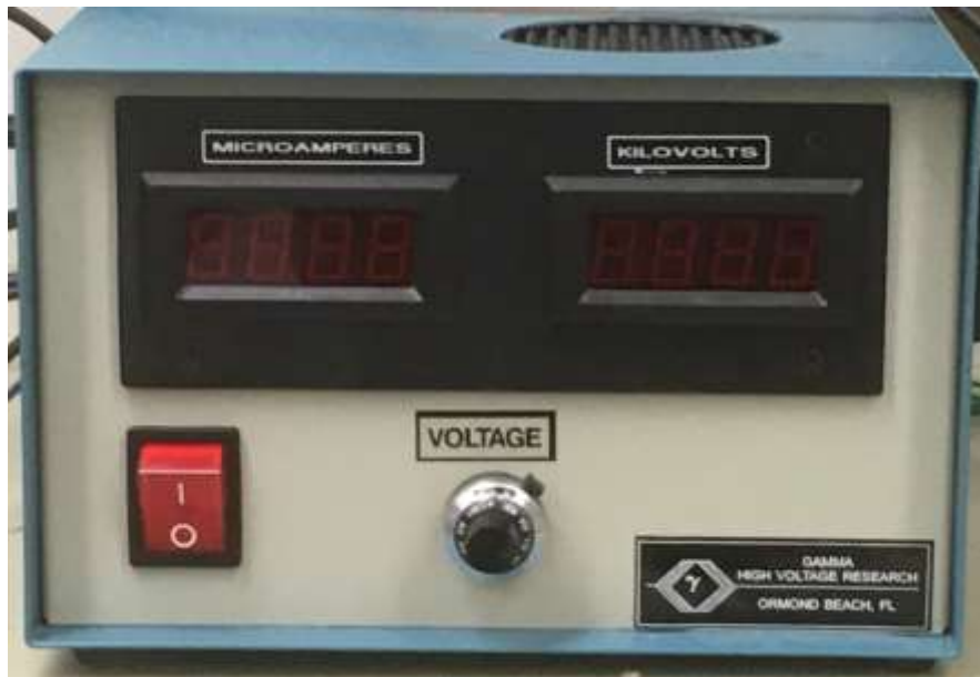
Figure 3-ES-100 High Voltage Source
