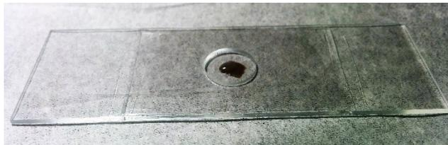
**Figure 4-1: Well type slide with glass coverslip bottom for imaging wet MFT and dilute MFT samples in epifluorescence microscope.**
