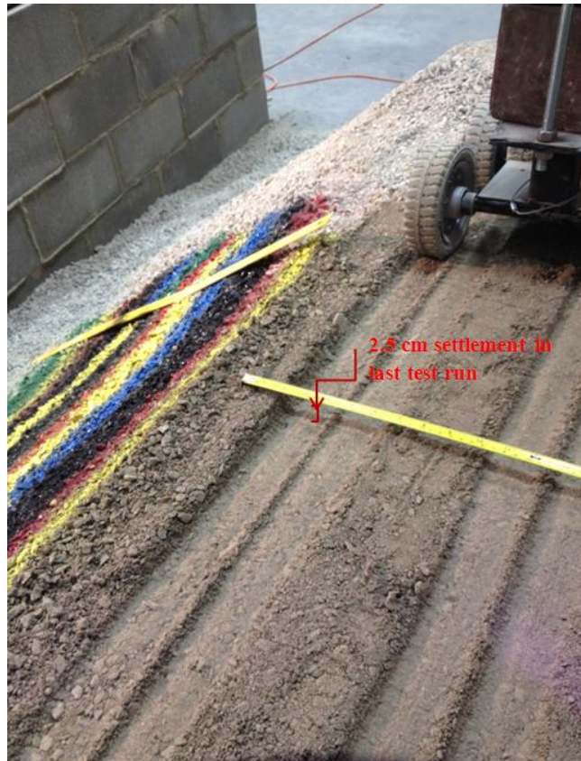
Figure 133: 2.5cm settlement in to ground after 20 test run
