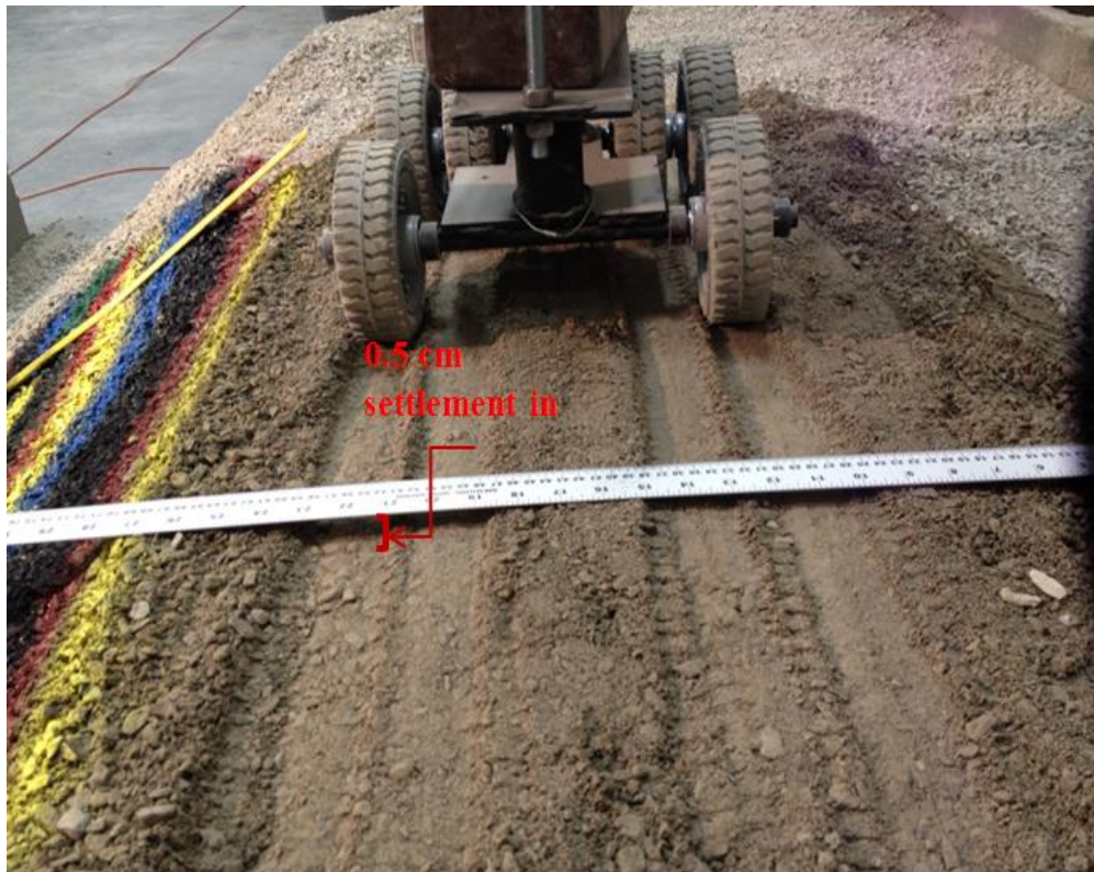
Figure 132: 0.5 cm settlement in to ground after second test run
