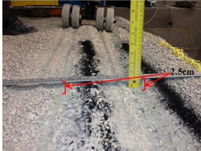
Figure 42: Ground profile of truck movement in 17 cm from edge
