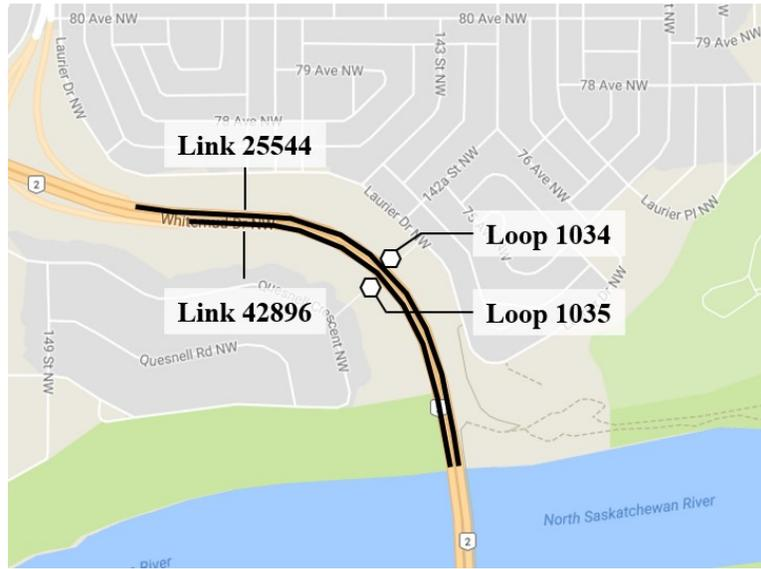
**FIGURE 4.4 Locations of Dual-Loop Detector on Whitemud Drive**
