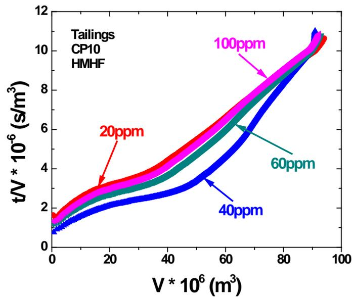
Figure C-4 Specific Resistance of Filtration of Tailings with CP10 Addition at Temperature above Corresponding LCST: (top) Comparison with Blank Sample (bottom) Magnification of Curves of Different Dosages
