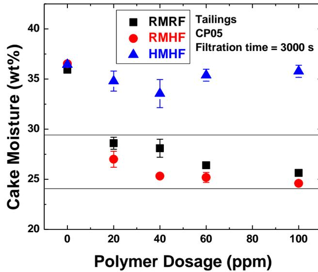
Figure 7-2-2 Moisture Content of Tailings Filter Cake in Different Filtration Cases with CP05 as Flocculant
