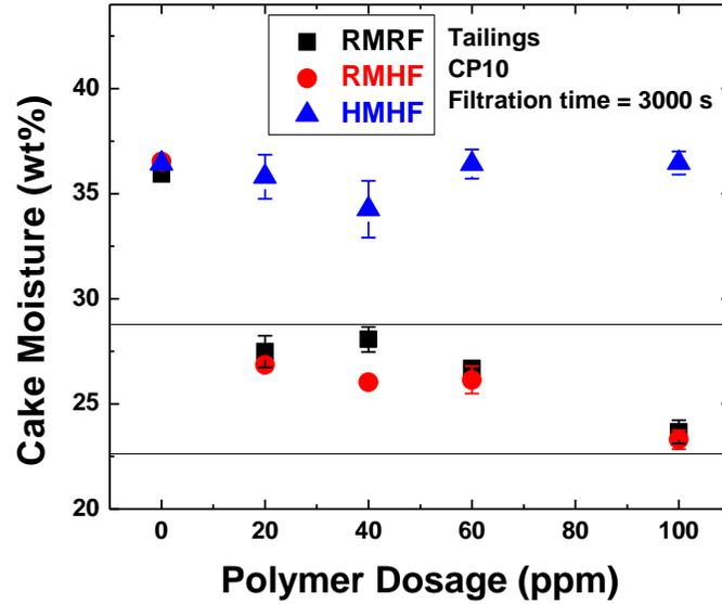
Figure 7-2-4 Moisture Content of Tailings Filter Cakes in Different Filtration Cases with CP10 as Flocculant
