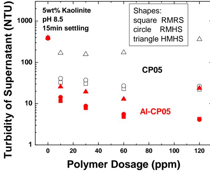
Figure 6-3-2 Comparison between Al-CP05 and CP05 on Supernatant Turbidity of Kaolinite Suspensions
