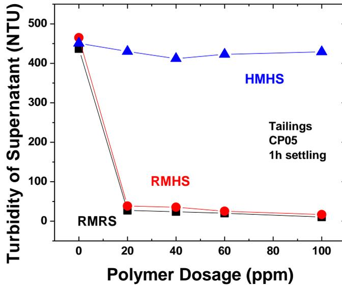
Figure 7-1-2 Supernatant Turbidity of Tailings in Different Settling Cases with CP05 as Flocculant
