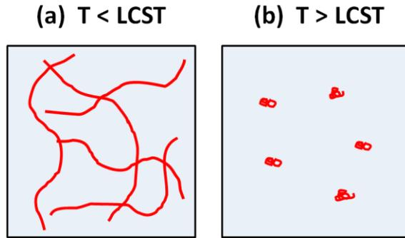
Figure 2-2-3 Schematics of the Coil-Globule Transition of Temperature Sensitive Polymers
