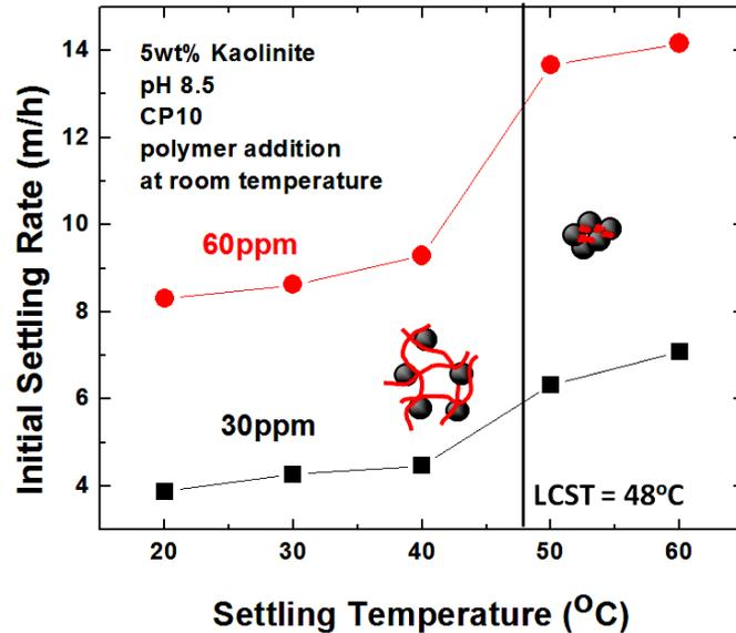
Figure 5-1-7 Effect of Settling Temperature on Settling of Kaolinite Suspensions with CP10 Added at Room Temperature
