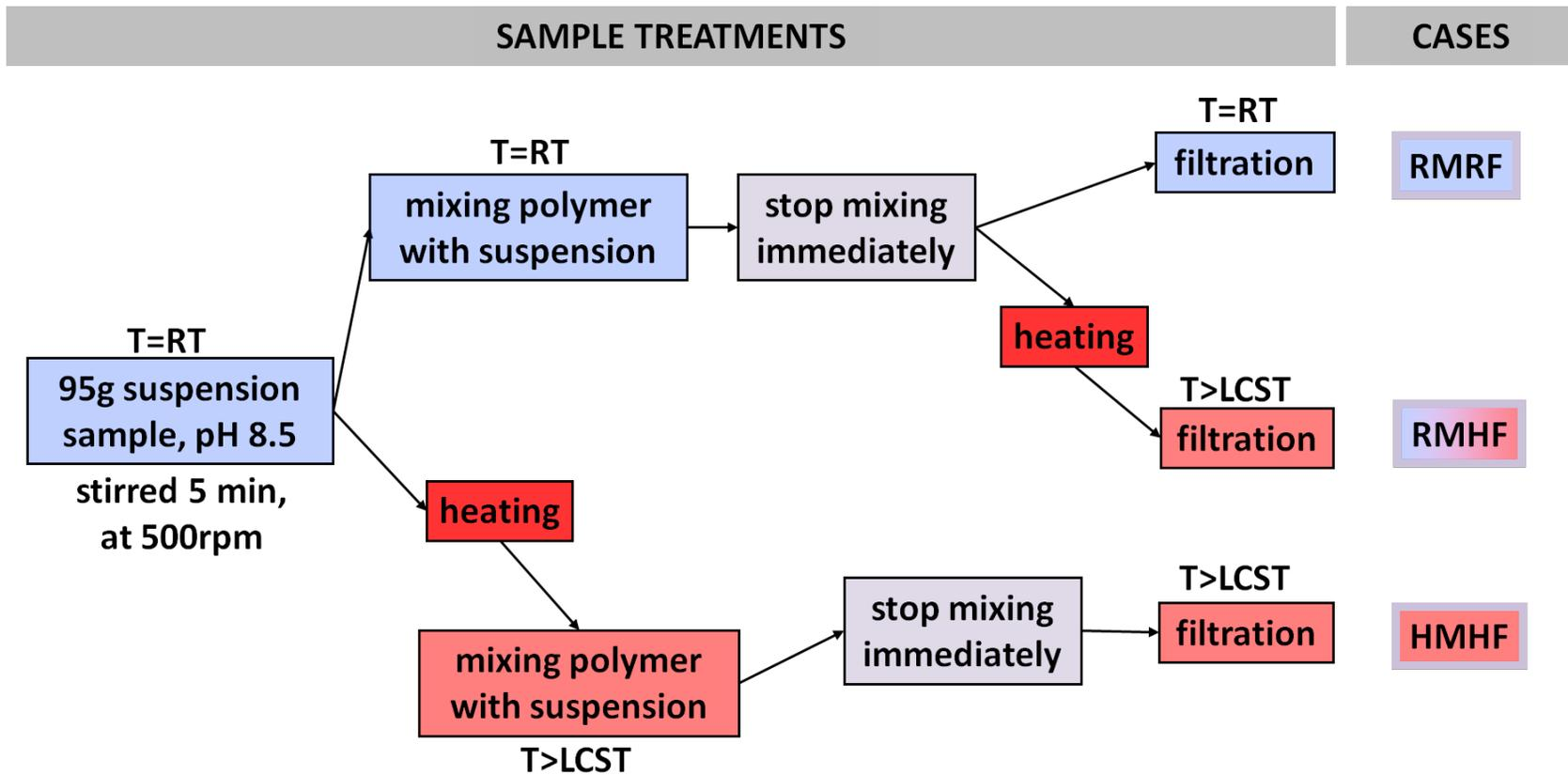
Figure 3-4-1 Proposed Cases Used in Filtration Tests
