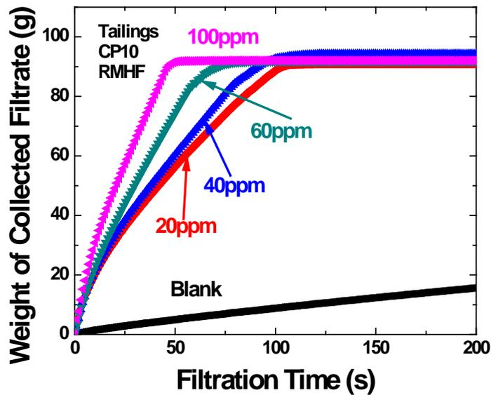
Figure B-6 Filtration Curves of Mixing CP10 with Laboratory Extraction Tailings at Room Temperature and Filtration at Temperature above Corresponding LCST
