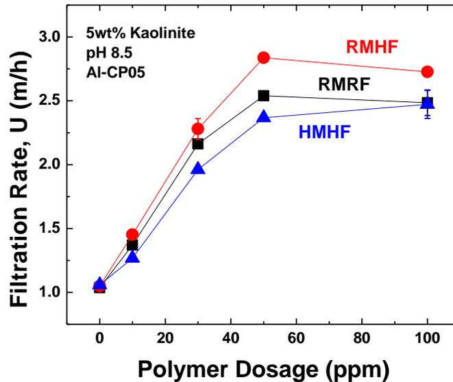
Figure 6-2-1 Filtration of Kaolinite Suspensions with Al-CP05 Addition in Different Filtration Cases
