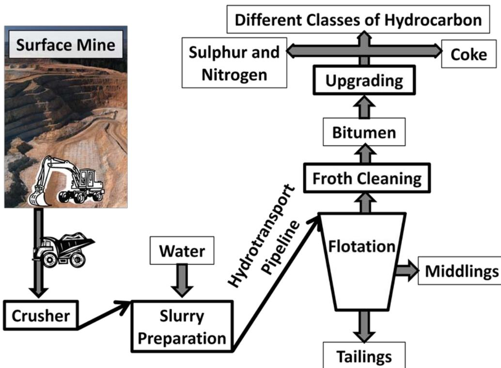
Figure 1-1-1 Schematic Flowchart of Bitumen Production [3]
