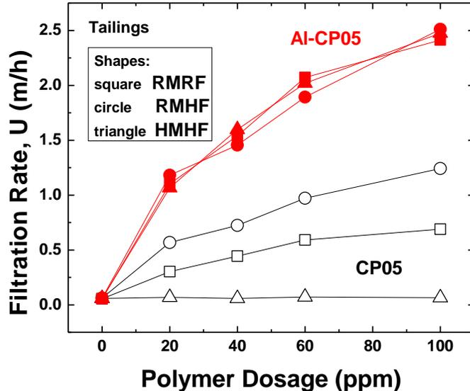
Figure 7-3-4 Comparison between Al-CP05 and CP05 on Filtration Performance of Tailings
