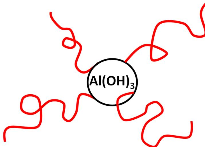
Figure 2-2-1 Schematic Diagram of the Proposed Structure of an Inorganic-Organic Hybrid Polymer Molecule
