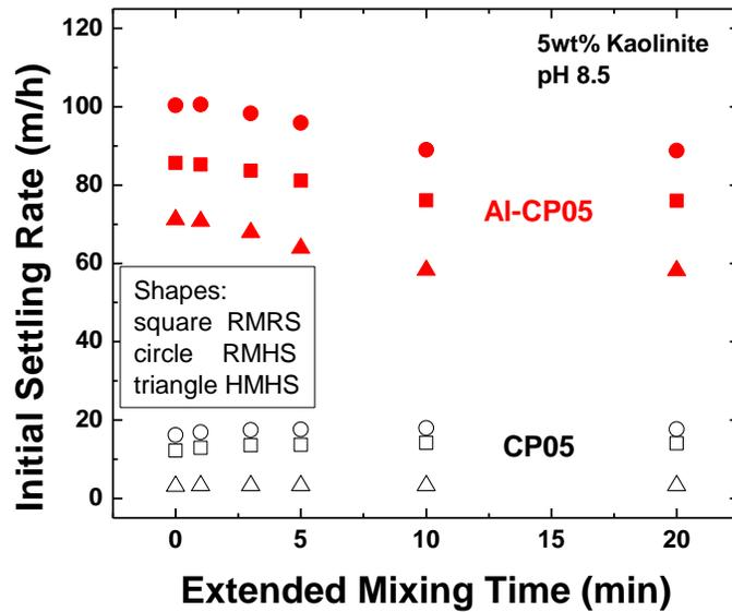
Figure 6-3-3 Comparison between Al-CP05 and CP05 on Floc Strength of Kaolinite Suspensions
