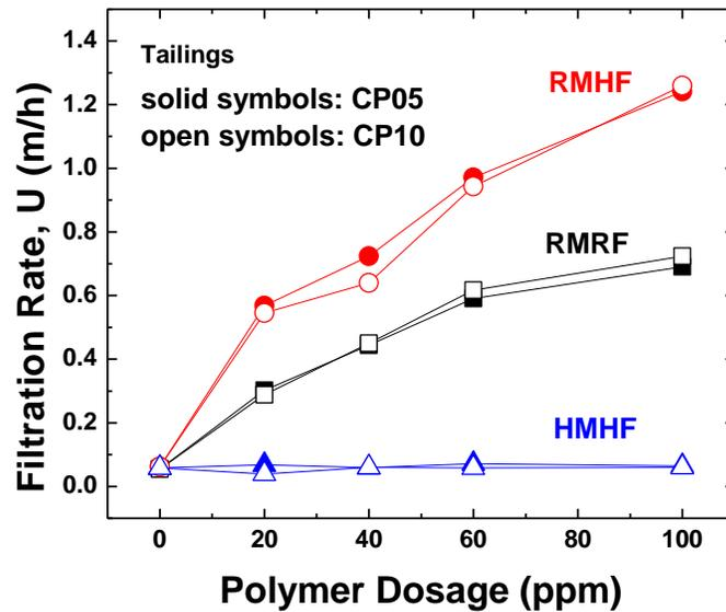
Figure 7-3-2 Comparison between CP05 and CP10 on Filtration Performance of Tailings
