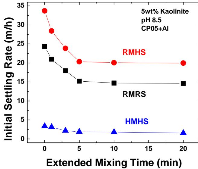
Figure 6-1-8 Effect of Mixing Time on Settling of Kaolinite Suspensions in Different Settling Cases with {CP05+Al} as Flocculant
