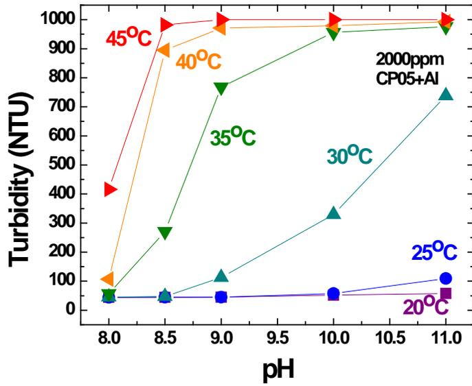
Figure D-4 The pH Induced Coil-Globule Transition of CP05+Al
