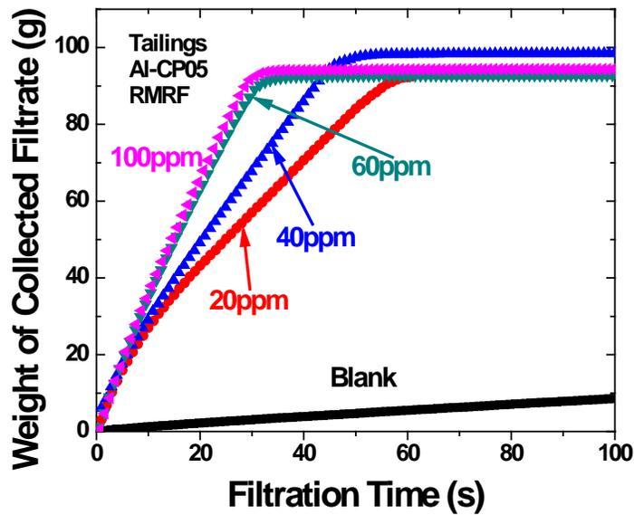
Figure B-8 Filtration Curves of Mixing Al-CP05 with and Filtration of Laboratory Extraction Tailings at Room Temperature
