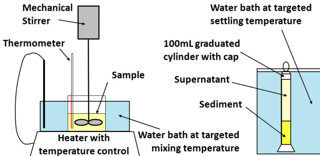
Figure 3-3-2 Schematic Setup of Settling Experiment
