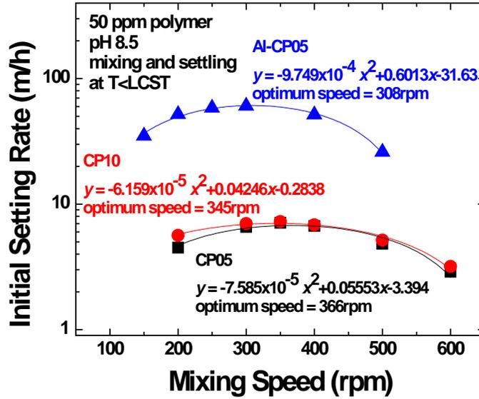
Figure 3-2-2 Mixing Condition of Each Flocculants in 5 wt% Kaolinite Suspensions at Temperatures below LCST
