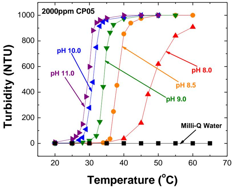
Figure 4-5-3 Lower Critical Solution Temperatures of CP05 at Different pH
