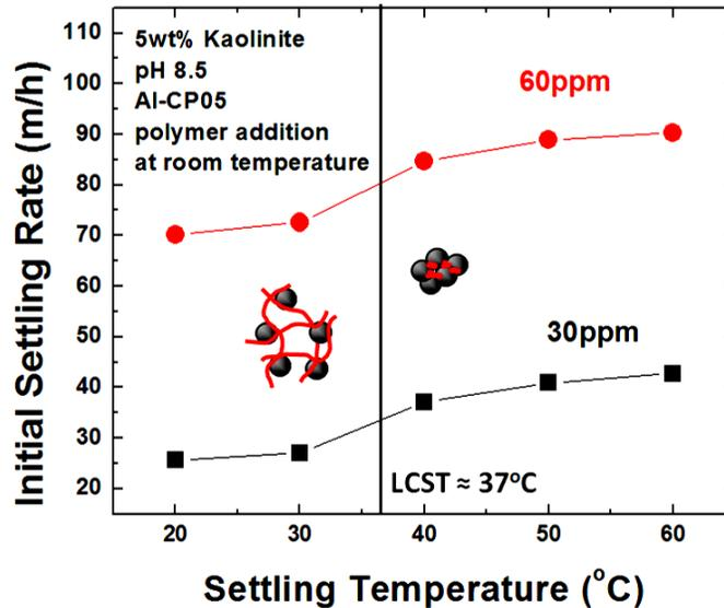
Figure 6-1-2 Effect of Settling Temperature on Settling of Kaolinite Suspensions with Al-CP05 Added at Room Temperature
