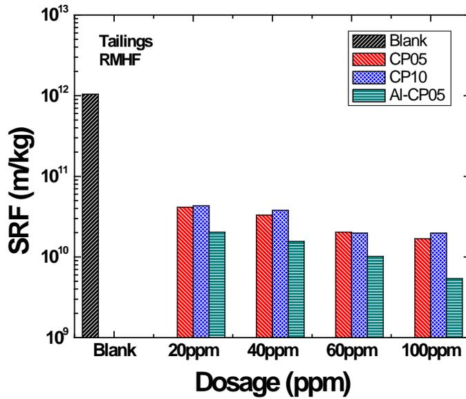
Figure C-12 Specific Resistances to Filtration of Tailings at Temperature above Corresponding LCST with Different Flocculants Added at Room Temperature
