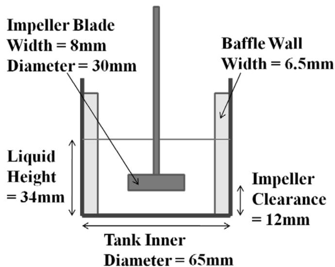
Figure 3-2-1 Schematics and Dimensions of Mixing Container
