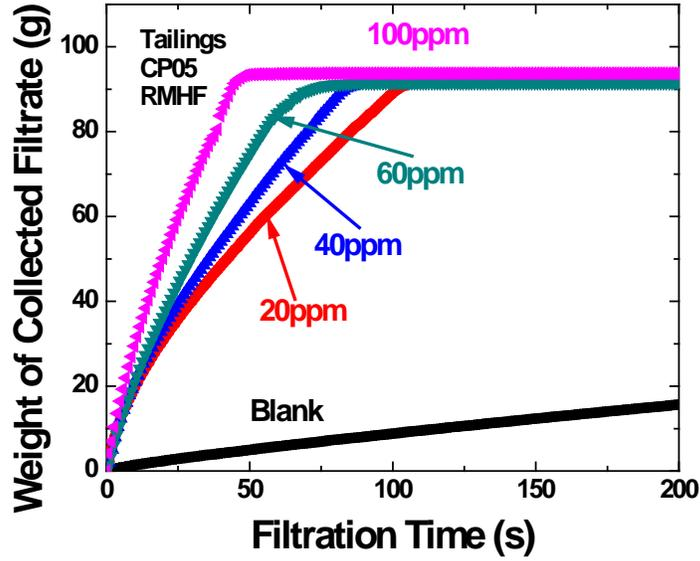
Figure B-3 Filtration Curves of Mixing CP05 with Laboratory Extraction Tailings at Room Temperature and Filtration at Temperature above Corresponding LCST
