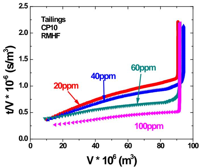
Figure C-6 Specific Resistance of Filtration of Tailings at Temperature above Corresponding LCST with CP10 Addition at Room Temperature: (top) Comparison with Blank Sample (bottom) Magnification of Curves of Different Dosages
