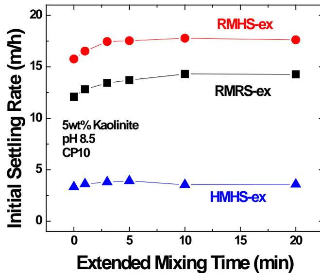
Figure 5-1-10 Effect of Mixing Time on Settling of Kaolinite Suspensions in Different Settling Cases with CP10 as Flocculant
