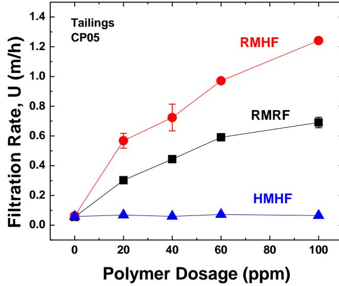
Figure 7-2-1 Filtration Performance of CP05 on Tailings in Different Filtration Cases
