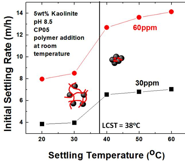
Figure 5-1-2 Effect of Settling Temperature on Settling of Kaolinite Suspensions with CP05 Added at Room Temperature
