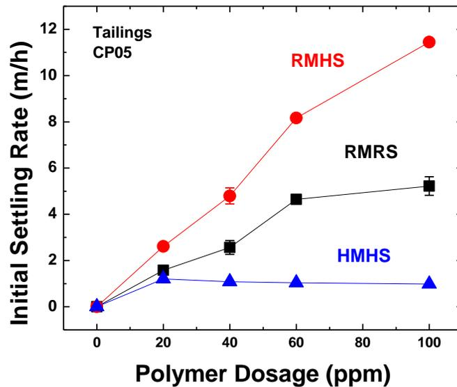
Figure 7-1-1 Settling Performance of CP05 on Tailings in Different Settling Cases
