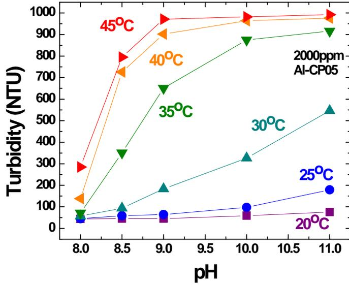
Figure D-3 The pH Induced Coil-Globule Transition of Al-CP05
