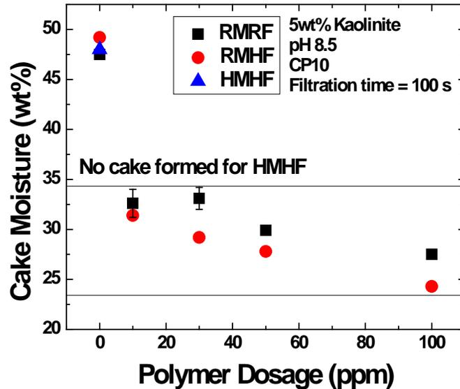
Figure 5-2-4 Moisture Content of Kaolinite Filter Cake in Different Filtration Cases with CP10 as Flocculant
