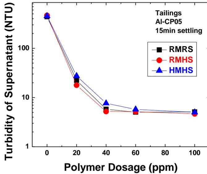
Figure 7-1-6 Supernatant Turbidity of Tailings in Different Settling Cases with AI-CP05 as Flocculant
