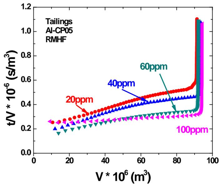
Figure C-9 Specific Resistance of Filtration of Tailings at Temperature above Corresponding LCST with Al-CP05 Addition at Room Temperature: (top) Comparison with Blank Sample (bottom) Magnification of Curves of Different Dosages
