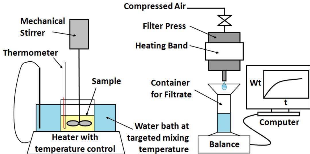
Figure 3-4-2 Schematic Setup of Filtration Experiment
