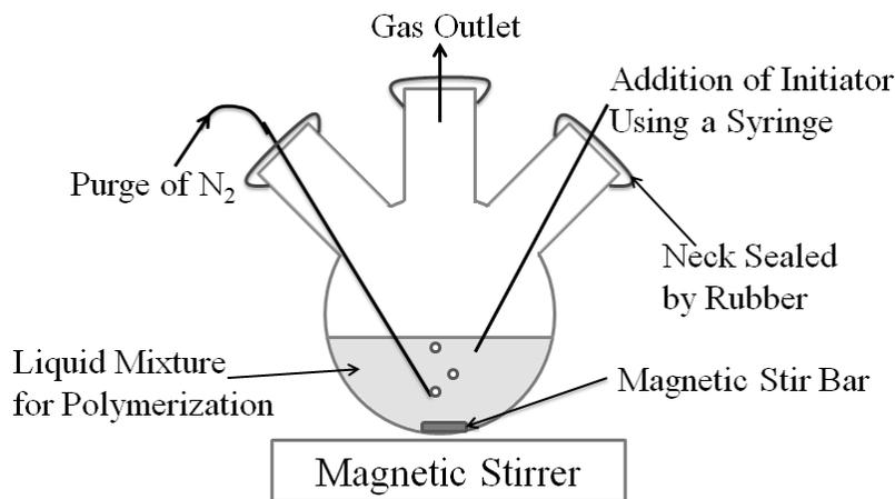
Figure 4-2-1 Apparatus used for Polymerization Reaction
