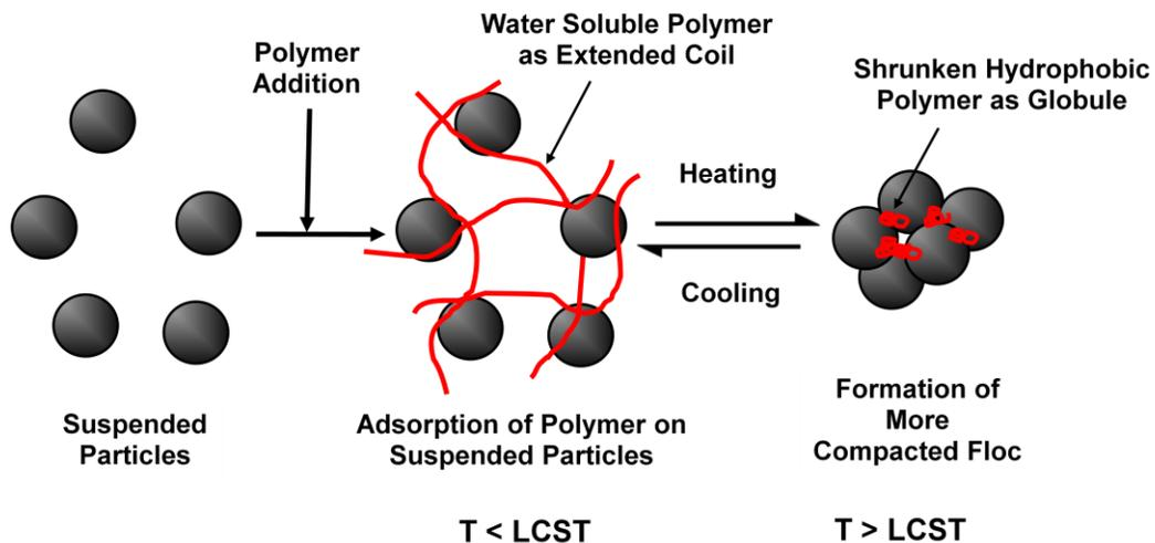
Figure 2-2-4 Proposed Flocculation Mechanism of Temperature Sensitive Polymers [39]
