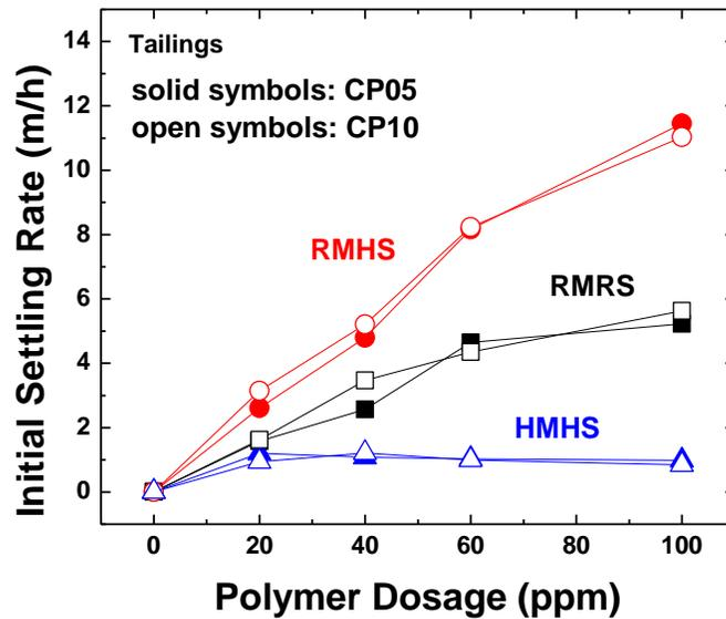
Figure 7-3-1 Comparison between CP05 and CP10 on Settling Performance of Tailings
