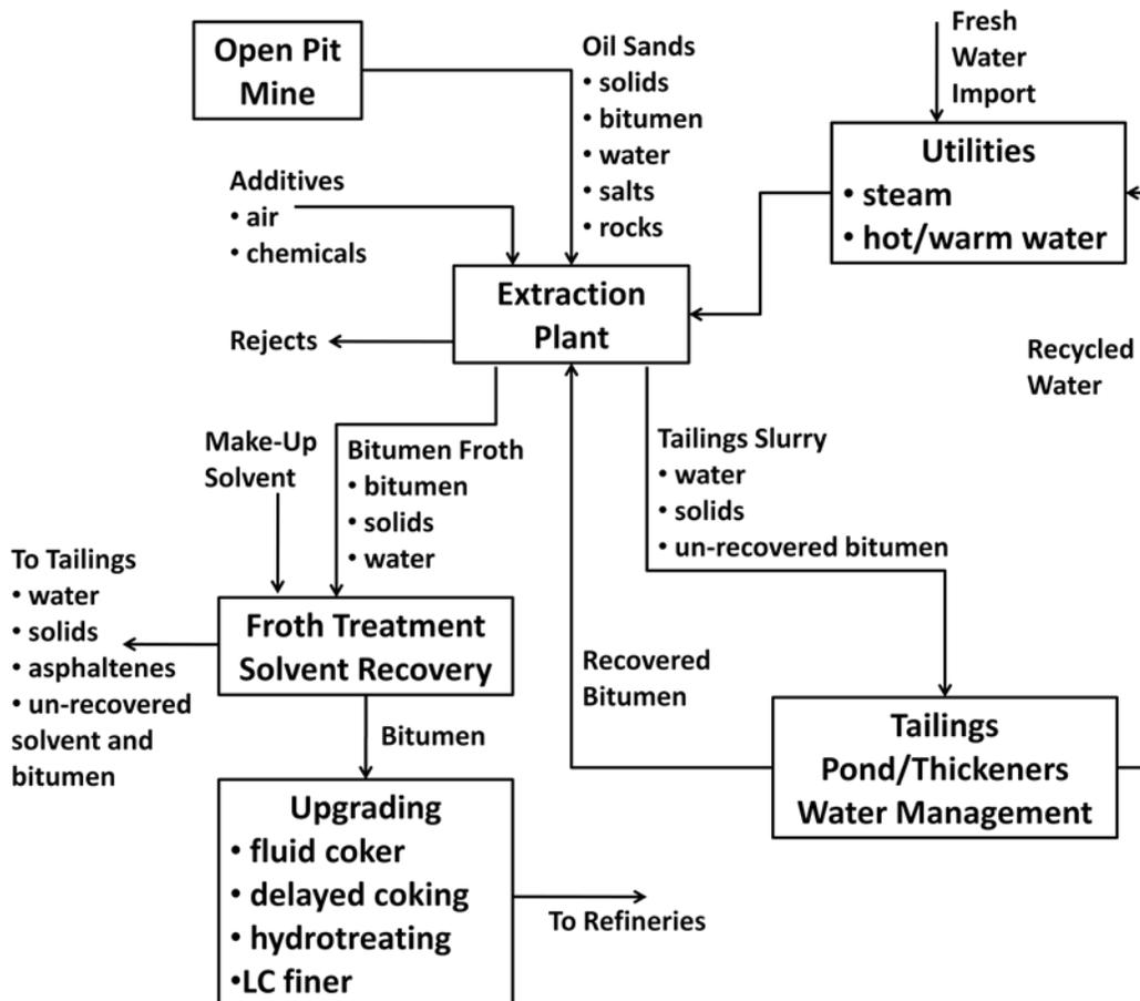
Figure 1-2-1 Generalized Flow Diagram for CHWE Process [3]
