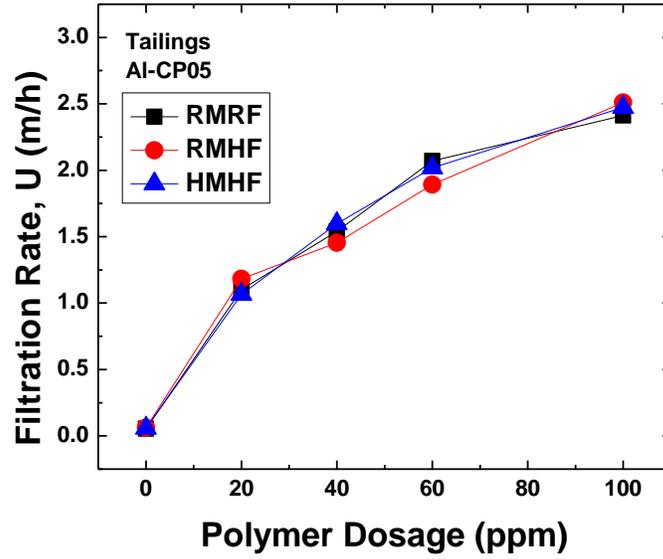
Figure 7-2-5 Filtration Performance of Al-CP05 on Tailings in Different Filtration Cases
