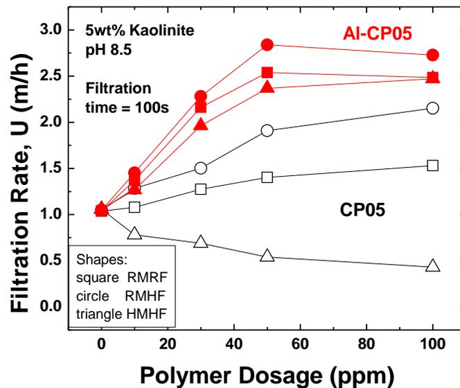
Figure 6-3-4 Comparison between Al-CP05 and CP05 on Filtration of Kaolinite Suspensions
