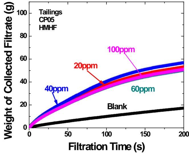
Figure B-1 Filtration Curves of Mixing CP05 with and Filtration of Laboratory Extraction Tailings both at Temperature above Corresponding LCST
