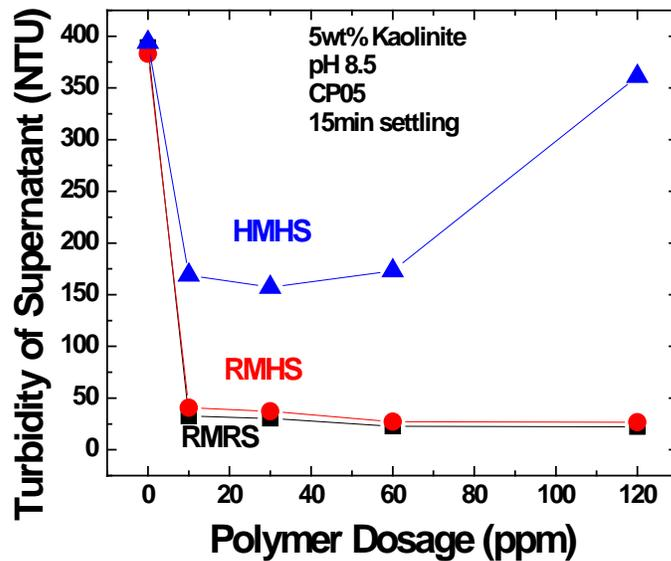
Figure 5-1-4 Supernatant Turbidity of Kaolinite Suspensions in Different Settling Cases with CP05 as Flocculant
