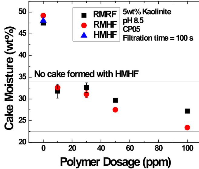
Figure 5-2-2 Moisture Content of Kaolinite Filter Cake in Different Filtration Cases with CP05 as Flocculant
