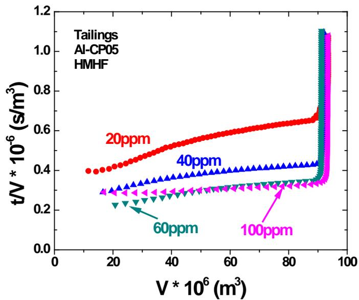
Figure C-7 Specific Resistance of Filtration of Tailings with Al-CP05 Addition both at Temperature above Corresponding LCST: (top) Comparison with Blank Sample (bottom) Magnification of Curves of Different Dosages
