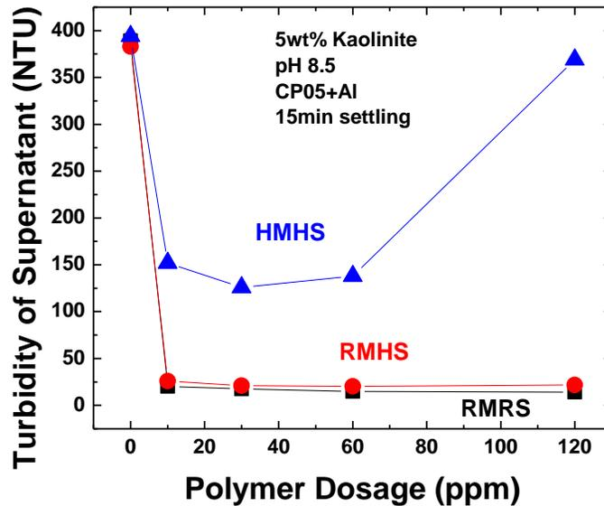
Figure 6-1-7 Turbidity of Supernatant of Kaolinite Suspensions in Different Settling Cases with {CP05+Al} as Flocculant
