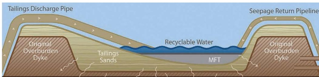
Figure 1-3-1 Schematic Diagram of a Tailings Pond [15]
