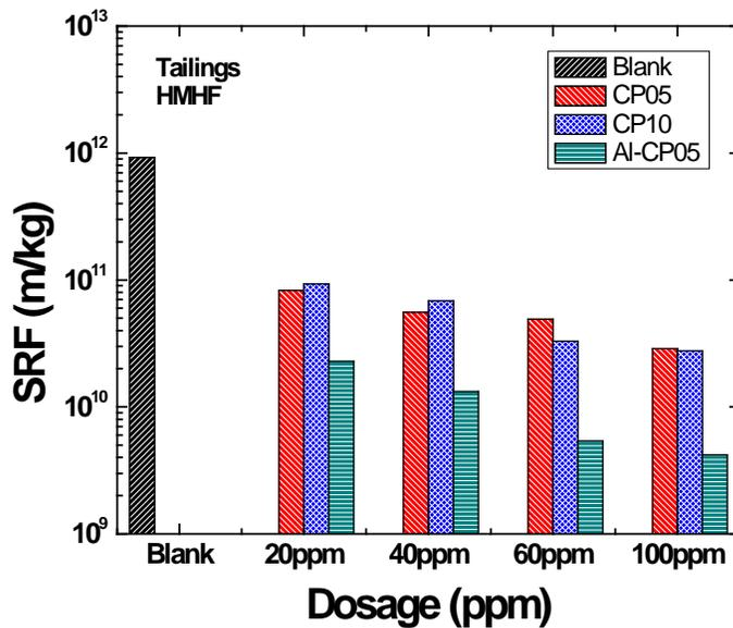
Figure C-10 Specific Resistances to Filtration of Tailings with Different Flocculants Added at Temperature above Corresponding LCST
