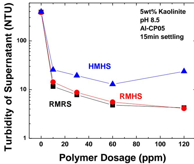
Figure 6-1-4 Turbidity of Supernatant of Kaolinite Suspensions in Different Settling Cases with Al-CP05 as Flocculant
