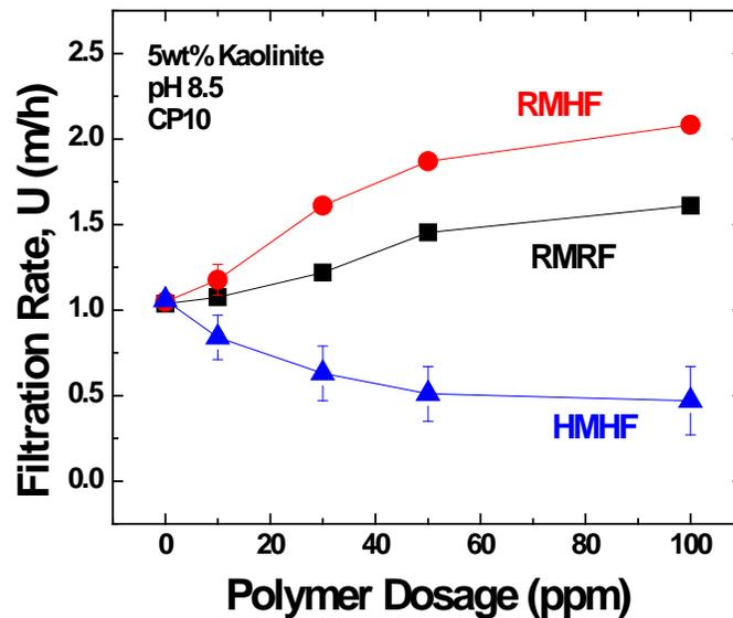
Figure 5-2-3 Filtration of Kaolinite Suspensions with CP10 Addition in Different Filtration Cases
