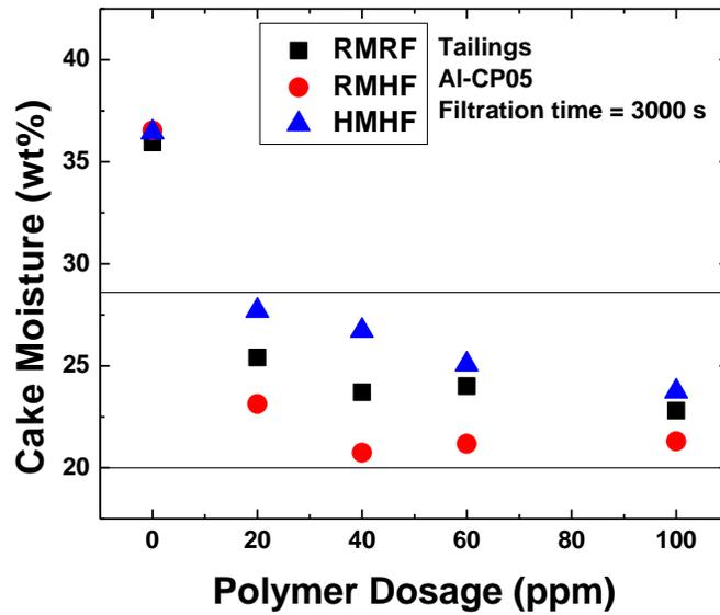
Figure 7-2-6 Moisture Content of Tailings Filter Cake in Different Filtration Cases with Al-CP05 as Flocculant
