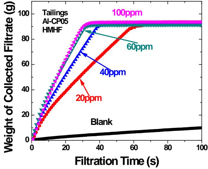
Figure B-7 Filtration Curves of Mixing Al-CP05 with and Filtration of Laboratory Extraction Tailings at Temperature above Corresponding LCST
