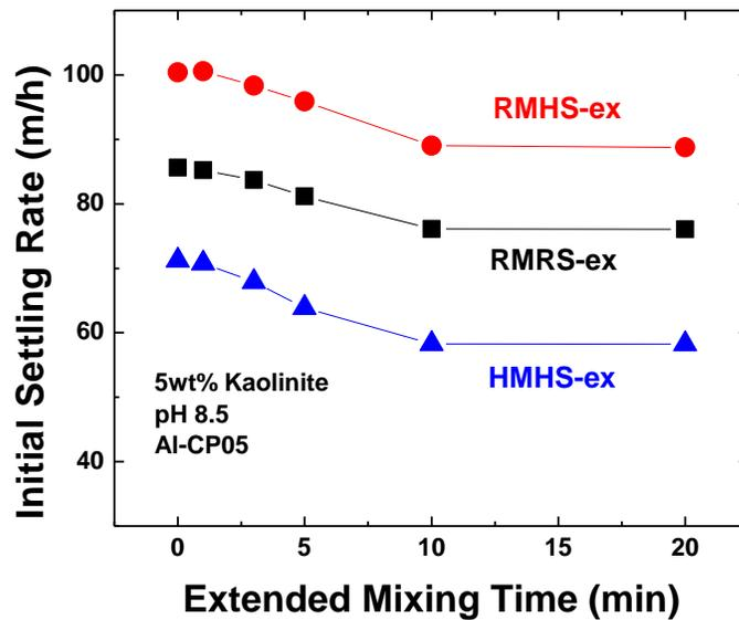
Figure 6-1-5 Effect of Mixing Time on Settling of Kaolinite Suspensions in Different Settling Cases with Al-CP05 as Flocculant
