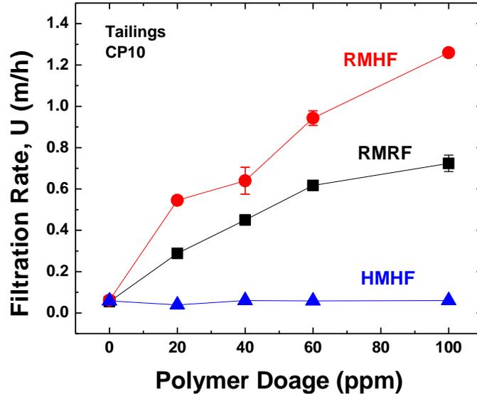
Figure 7-2-3 Filtration Performance of CP10 on Tailings in Different Filtration Cases
