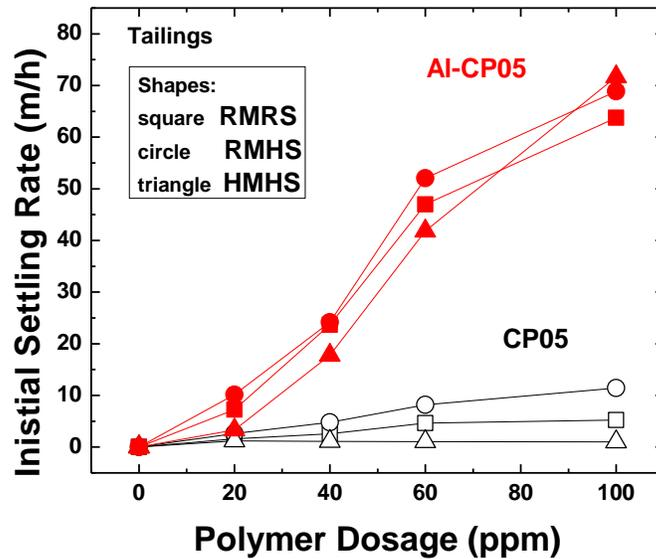
Figure 7-3-3 Comparison between Al-CP05 and CP05 on Settling Performance of Tailings
