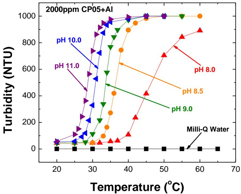
Figure 4-5-6 Lower Critical Solution Temperatures of {CP05+Al} at Different pH
