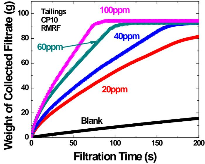
Figure B-5 Filtration Curves of Mixing CP10 with and Filtration of Laboratory Extraction Tailings both at Room Temperature
