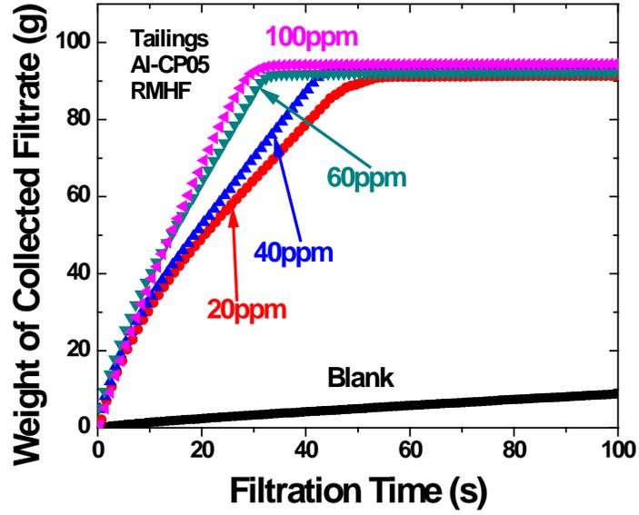
Figure B-9 Filtration Curves of Mixing Al-CP05 with Laboratory Extraction Tailings at Room Temperature and Filtration at Temperature above Corresponding LCST
