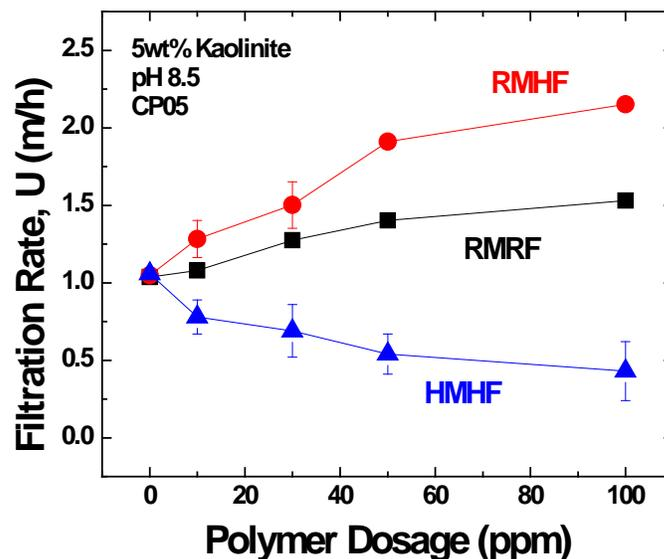
Figure 5-2-1 Filtration of Kaolinite Suspensions with CP05 Addition in Different Filtration Cases
