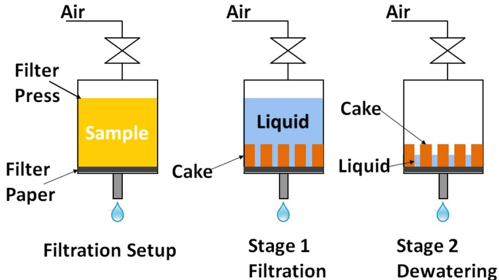
Figure 3-4-3 Schematic Diagram of Filtration Stages
