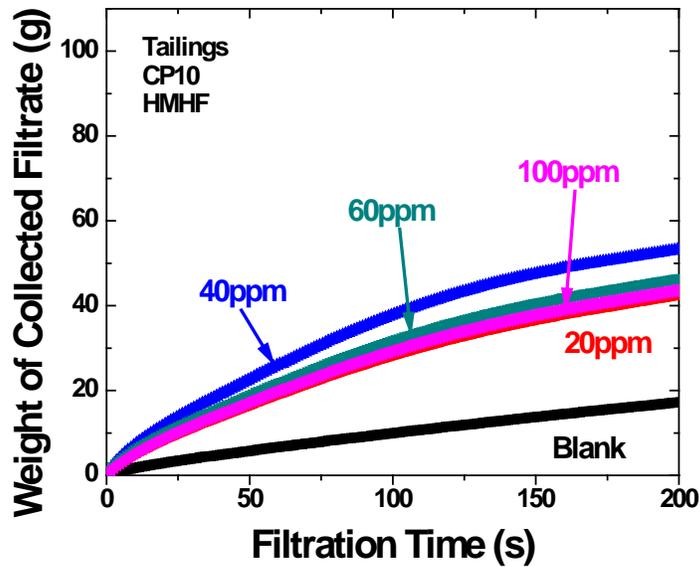
Figure B-4 Filtration Curves of Mixing CP10 with and Filtration of Laboratory Extraction Tailings both at Temperature above Corresponding LCST
