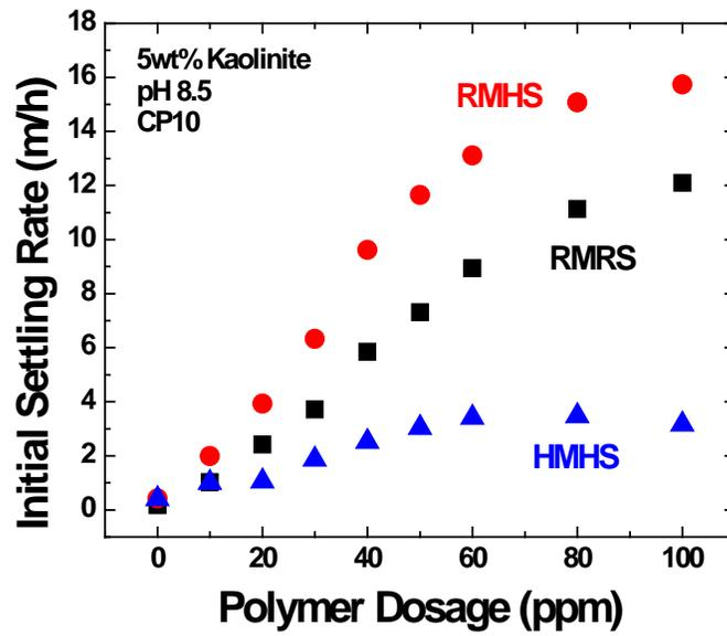
Figure 5-1-8 Settling of Kaolinite Suspensions with CP10 Addition in Different Settling Cases
