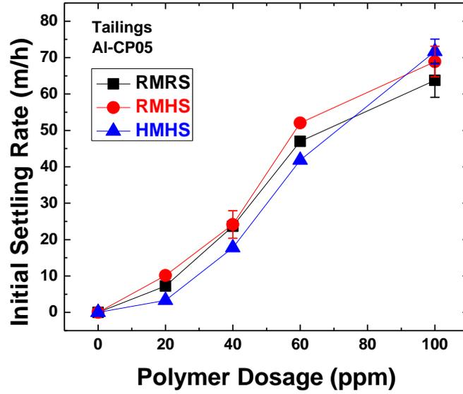
Figure 7-1-5 Settling Performance of AI-CP05 on Tailings in Different Settling Cases
