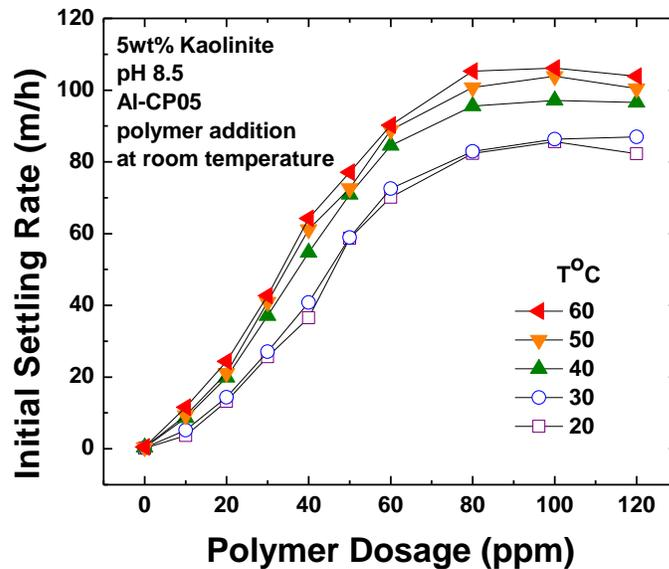
Figure 6-1-1 Initial Settling Rate of Kaolinite Suspensions with Al-CP05 Added at Room Temperature
