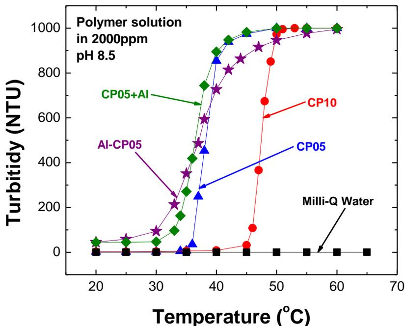
Figure 4-5-2 Lower Critical Solution Temperatures of All Flocculants at pH 8.5
