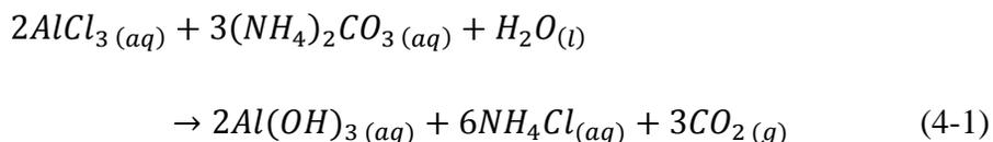
The  $Al(OH)_3$  colloids were prepared one day prior to the synthesis of polymer-colloid hybrid,  $Al(OH)_3$ -P[NIPAM-co-DMAPMA], (Al-CP).
