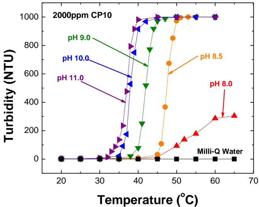
Figure 4-5-4 Lower Critical Solution Temperatures of CP10 at Different pH
