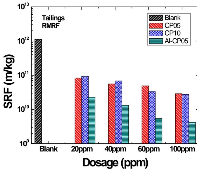
Figure C-11 Specific Resistances to Filtration of Tailings with Different Flocculants Added at Room Temperature
