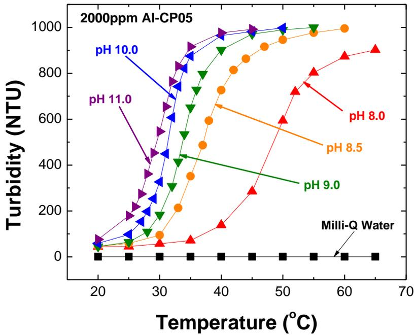
Figure 4-5-5 Lower Critical Solution Temperatures of Al-CP05 at Different pH
