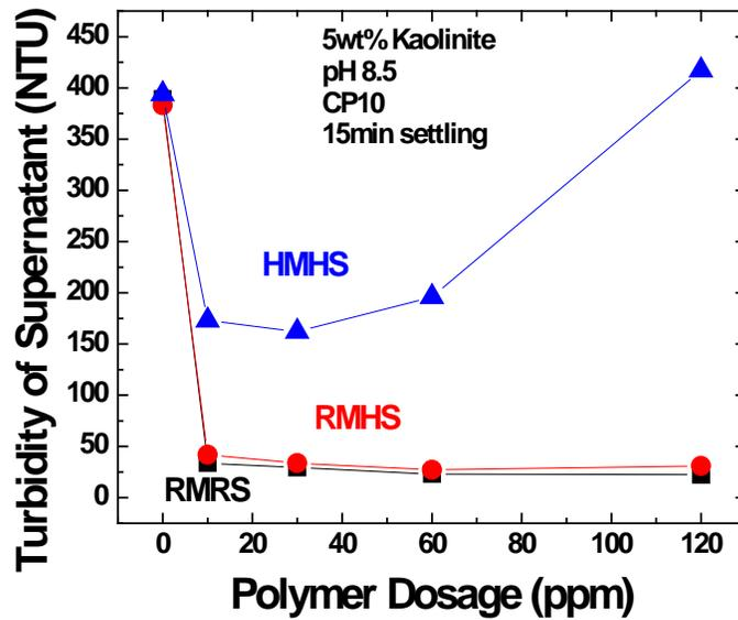
Figure 5-1-9 Supernatant Turbidity of Kaolinite Suspensions in Different Settling Cases with CP10 as Flocculant
