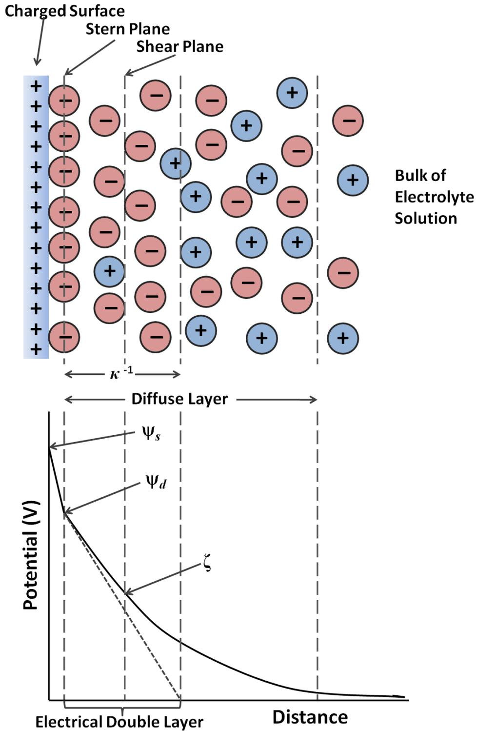
Figure 2-1-3 Schematic Illustration of the Electrical Double Layer according to Stern Model (top) and Corresponding Electrical Potential Profile Showing the Debye Length ( $\kappa^{-1}$ ) and the Diffuse Layer (bottom) [8]
