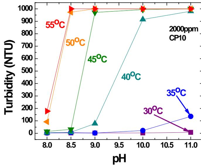
Figure D-2 The pH Induced Coil-Globule Transition of CP10
