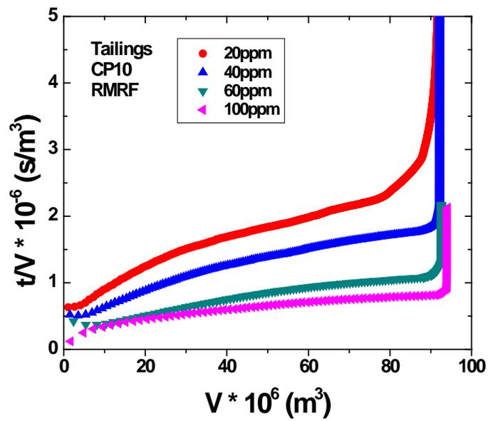
Figure C-5 Specific Resistance of Filtration of Tailings with CP10 Addition at Room Temperature: (top) Comparison with Blank Sample (bottom) Magnification of Curves of Different Dosages
