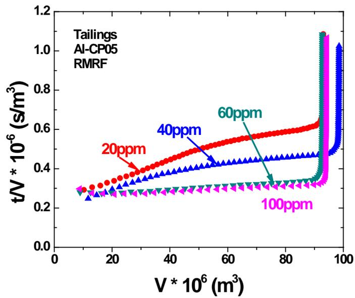
Figure C-8 Specific Resistance of Filtration of Tailings with Al-CP05 Addition at Room Temperature: (top) Comparison with Blank Sample (bottom) Magnification of Curves of Different Dosages
