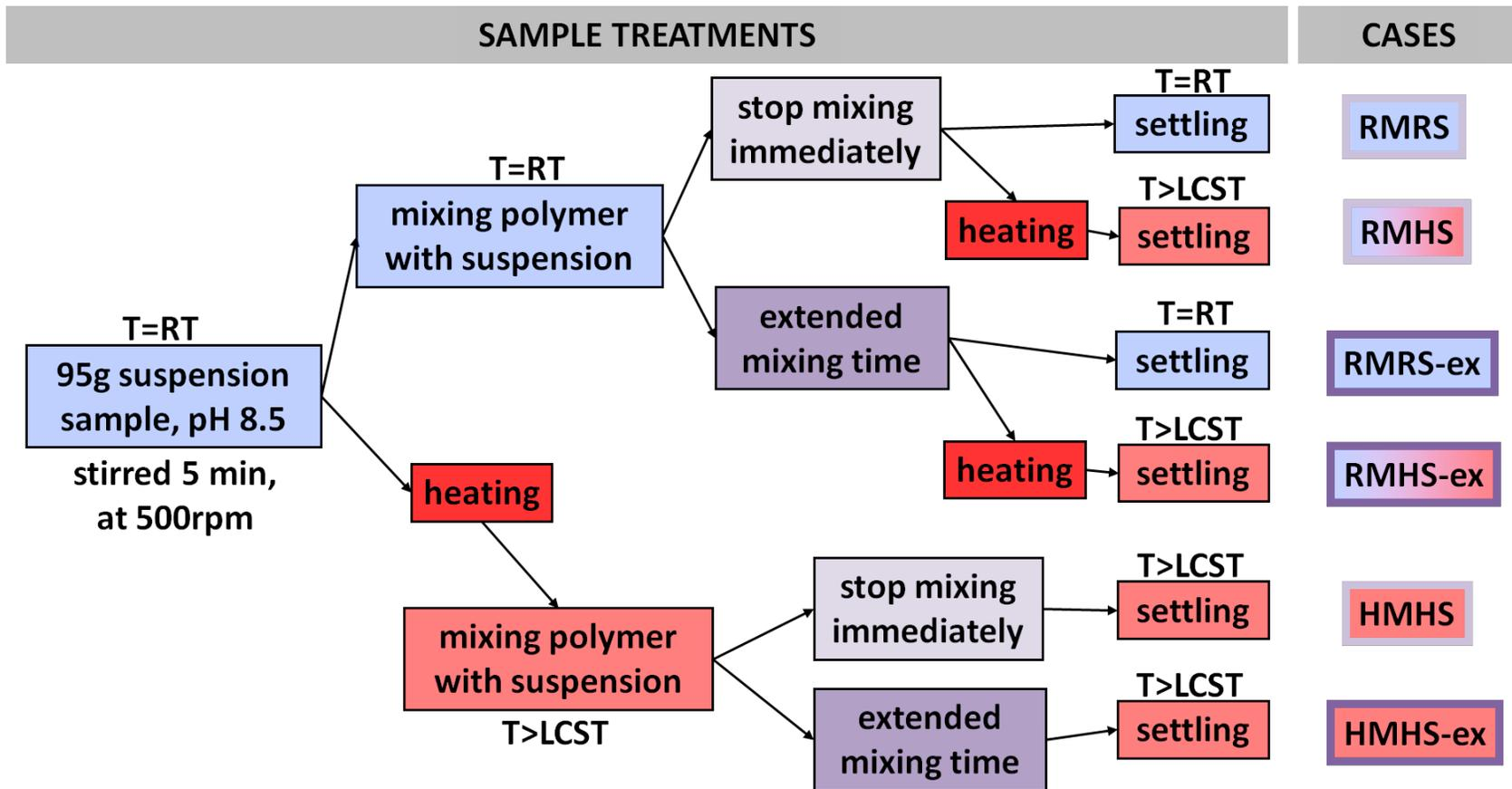
Figure 3-3-1 Proposed Cases Used in Settling Tests
