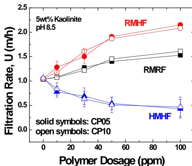
Figure 5-3-2 Comparison between CP05 and CP10 on Filtration Performance in Kaolinite Suspensions
