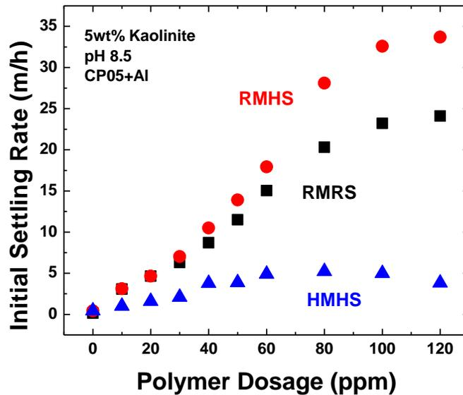
Figure 6-1-6 Settling of Kaolinite Suspensions with {CP05+Al} Addition in Different Settling Cases
