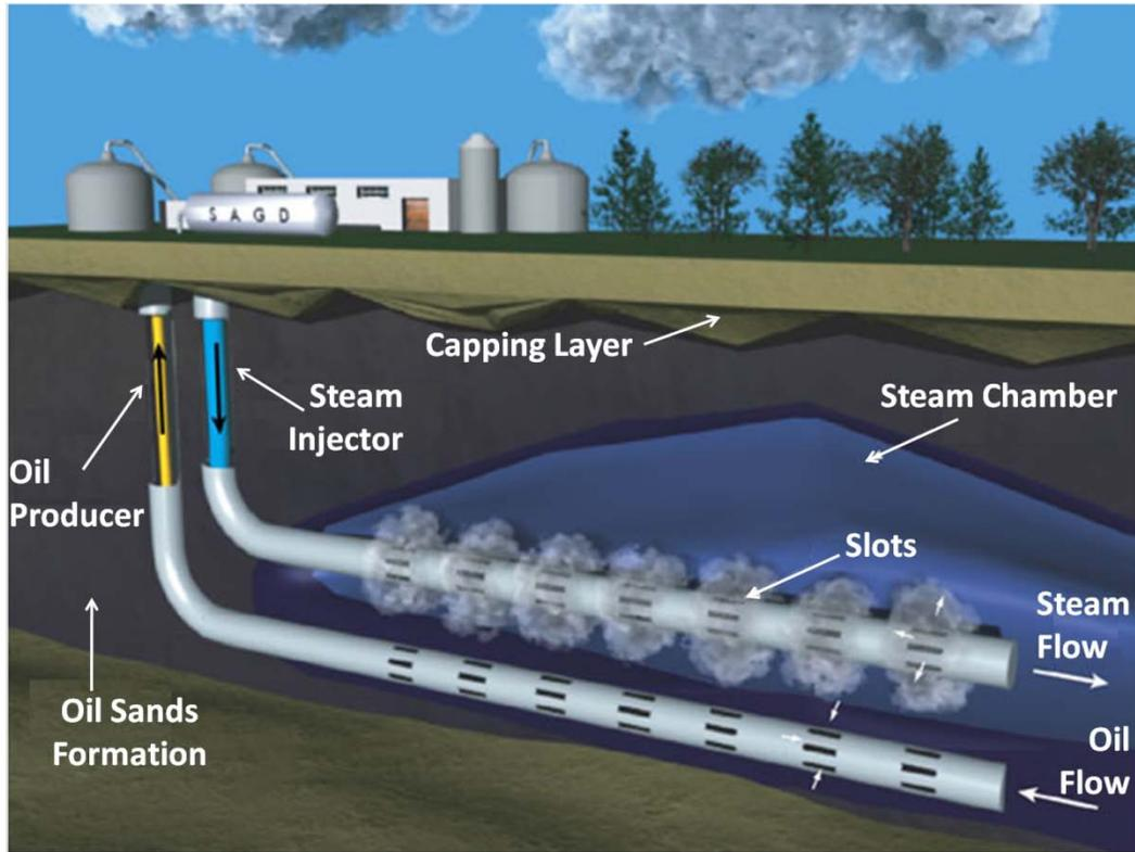
Figure 1-2-2 Schematic Diagram of SAGD Process [6]
