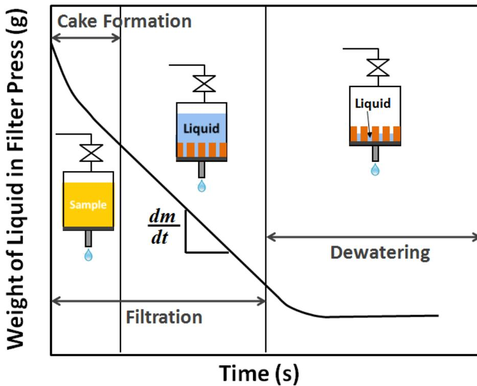
Figure 3-4-5 Filtration Stages in Filtration Curve
