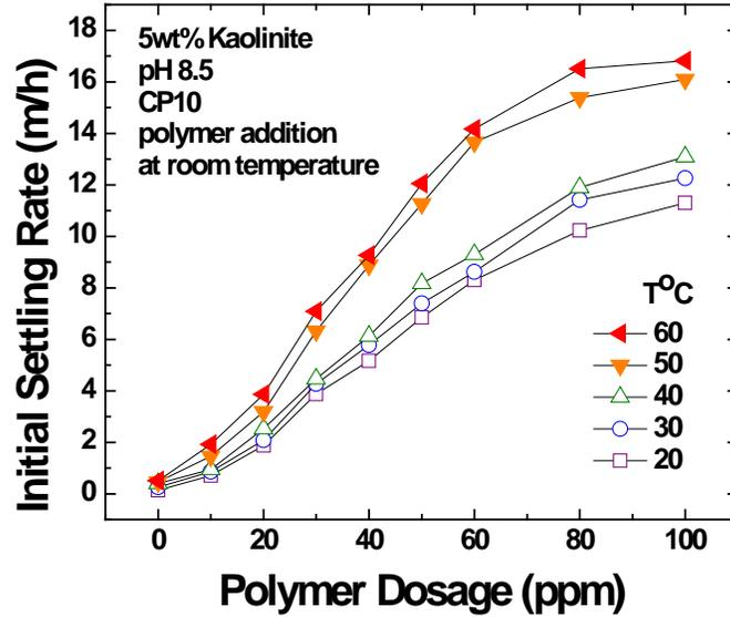
Figure 5-1-6 Initial Settling Rate of Kaolinite Suspensions with CP10 Added at Room Temperature
