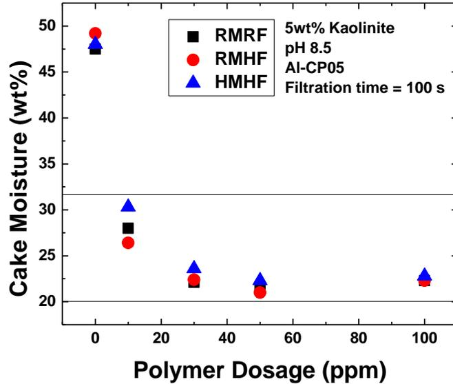
Figure 6-2-2 Moisture Content of Kaolinite Filter Cake in Different Filtration Cases with Al-CP05 as Flocculant
