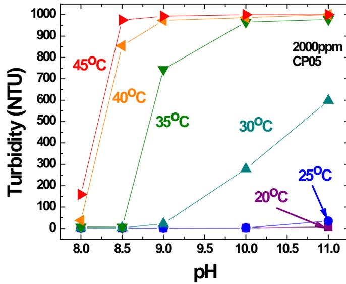
Figure D-1 The pH Induced Coil-Globule Transition of CP05
