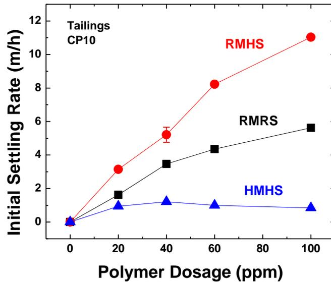
Figure 7-1-3 Settling Performance of CP10 on Tailings in Different Settling Cases
