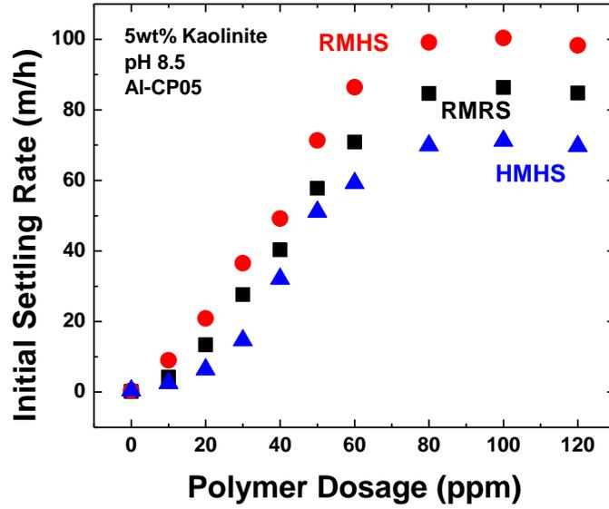
Figure 6-1-3 Settling of Kaolinite Suspensions with Al-CP05 Addition in Different Settling Cases
