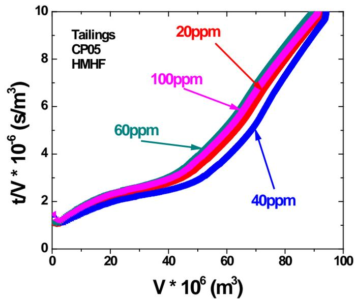
Figure C-1 Specific Resistance of Filtration of Tailings with CP05 Addition at Temperature above Corresponding LCST: (top) Comparison with Blank Sample (bottom) Magnification of Curves of Different Dosages
