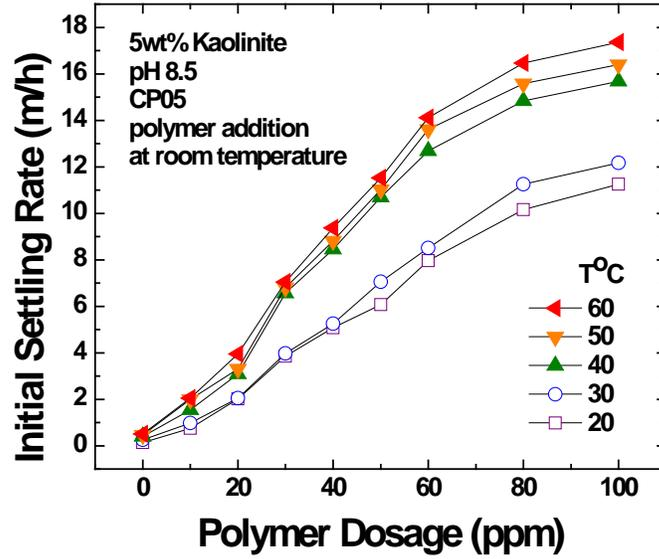
Figure 5-1-1 Initial Settling Rate of Kaolinite Suspensions with CP05 Added at Room Temperature
