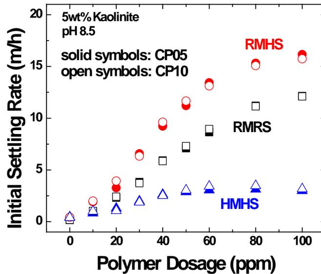
Figure 5-3-1 Comparison between CP05 and CP10 on Settling Performance in Kaolinite Suspensions
