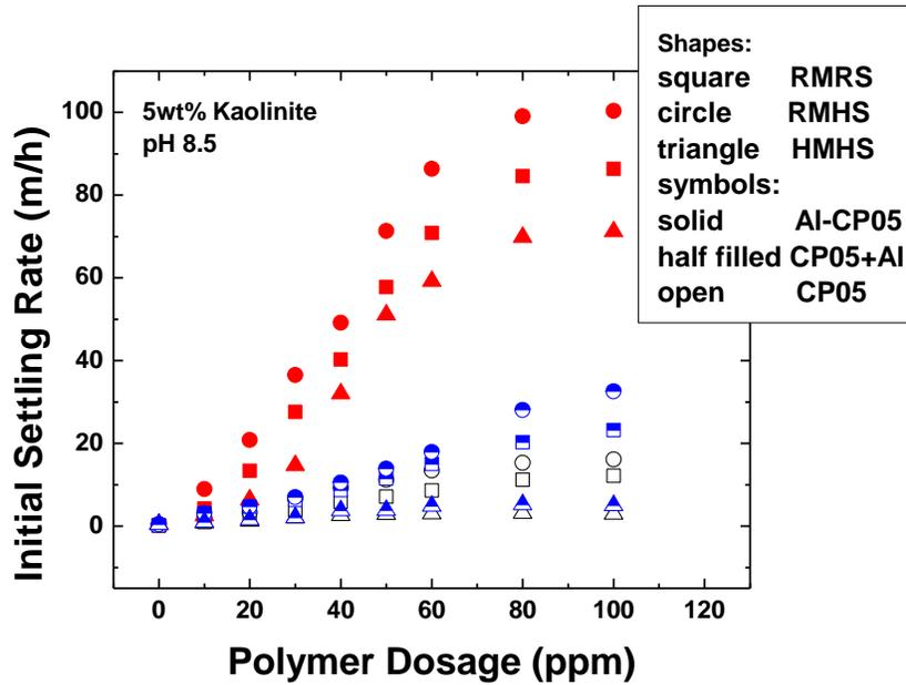
Figure 6-3-5 Comparison between Al-CP05, CP05, and {CP05+Al} on Settling of Kaolinite Suspensions
