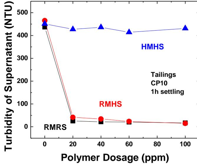
Figure 7-1-4 Supernatant Turbidity of Tailings in Different Settling Cases with CP10 as Flocculant
