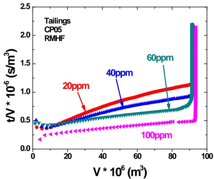
Figure C-3 Specific Resistance of Filtration of Tailings at Temperature above Corresponding LCST with CP05 Addition at Room Temperature: (top) Comparison with Blank Sample (bottom) Magnification of Curves of Different Dosages
