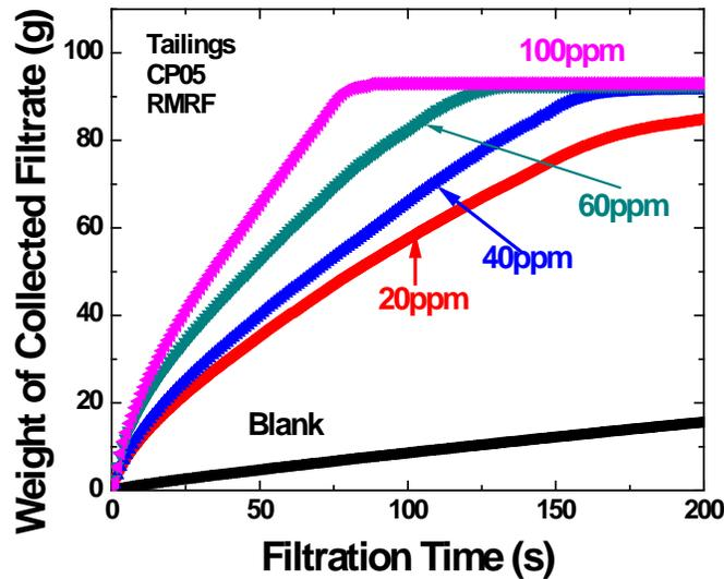
Figure B-2 Filtration Curves of Mixing CP05 with and Filtration of Laboratory Extraction Tailings both at Room Temperature
