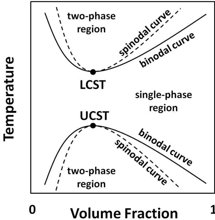
Figure 2-2-2 Schematic Phase Diagram for Polymer Solution Showing UCST and LCST Behaviours [31]
