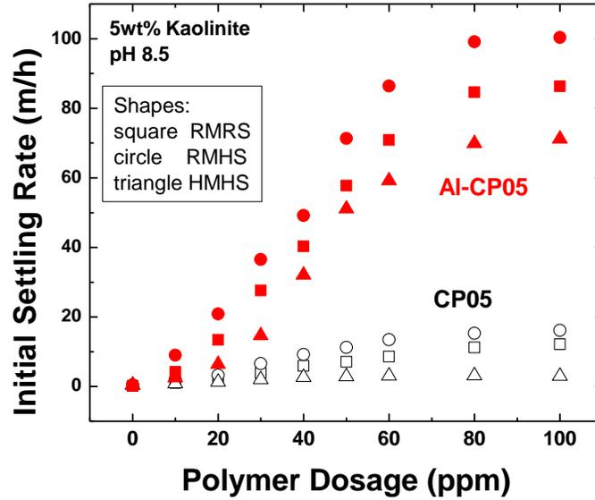
Figure 6-3-1 Comparison between Al-CP05 and CP05 on Settling of Kaolinite Suspensions
