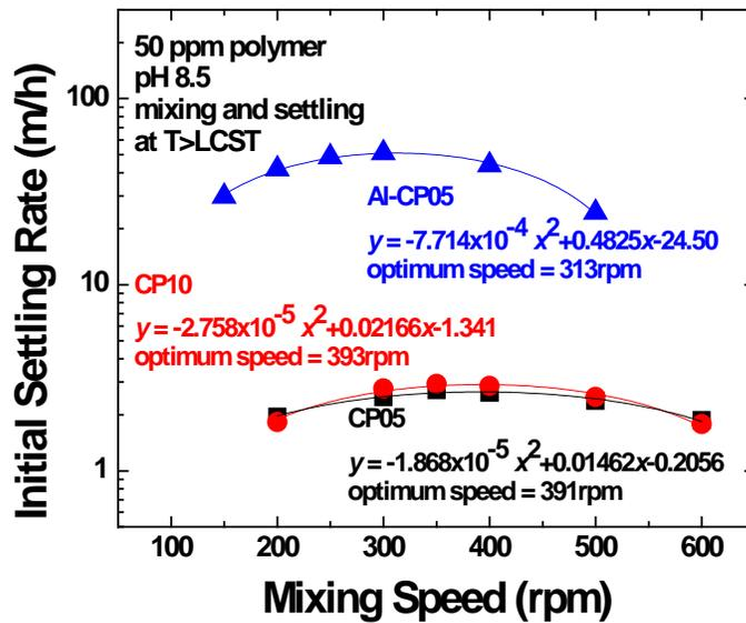
Figure 3-2-3 Mixing Condition of Each Flocculants in 5 wt% Kaolinite Suspensions at Temperatures above LCST
