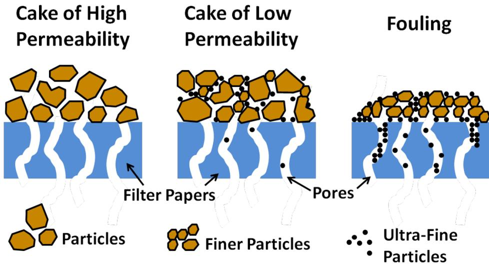
Figure 3-4-4 Schematic Diagram of Different Filter Cake Structures
