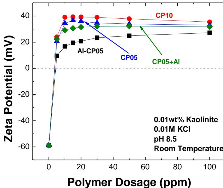
Figure 4-5-7 Effect of Flocculants on the Surface Charge of Kaolinite Particles
