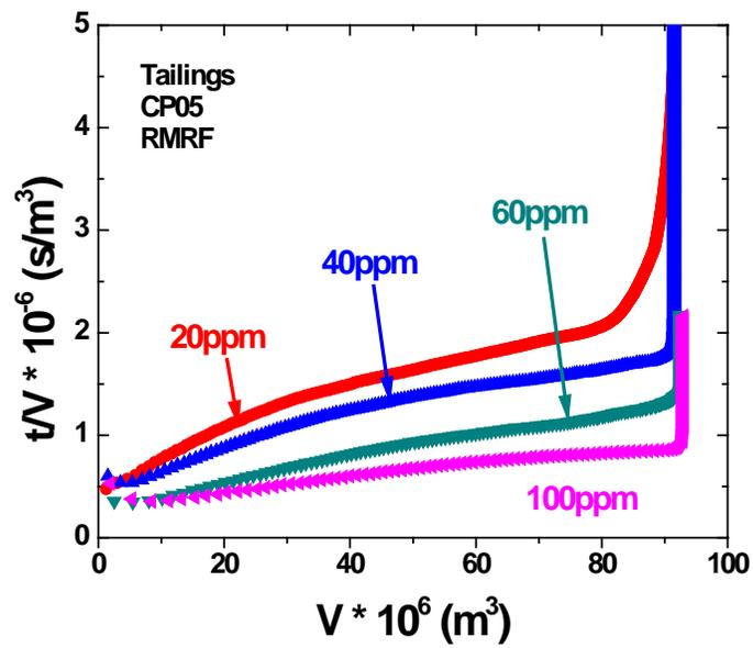
Figure C-2 Specific Resistance of Filtration of Tailings with CP05 Addition at Room Temperature: (top) Comparison with Blank Sample (bottom) Magnification of Curves of Different Dosages
