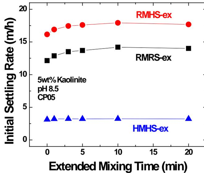
Figure 5-1-5 Effect of Mixing Time on Settling of Kaolinite Suspensions in Different Settling Cases with CP05 as Flocculant
