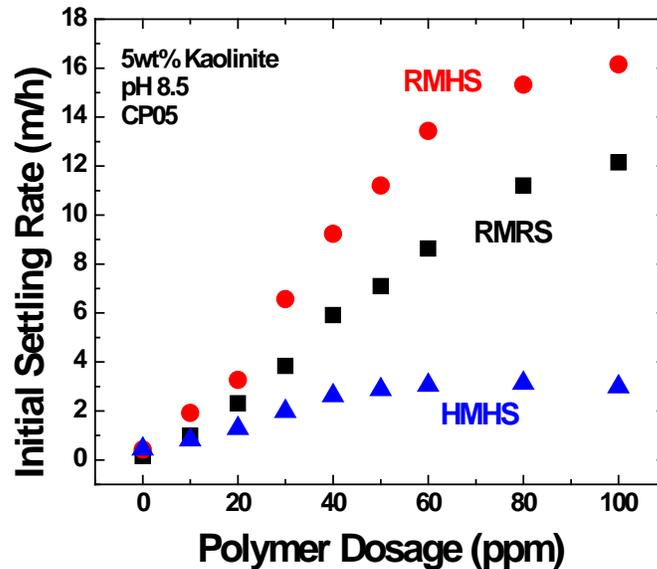
Figure 5-1-3 Settling of Kaolinite Suspensions with CP05 Addition in Different Settling Cases
