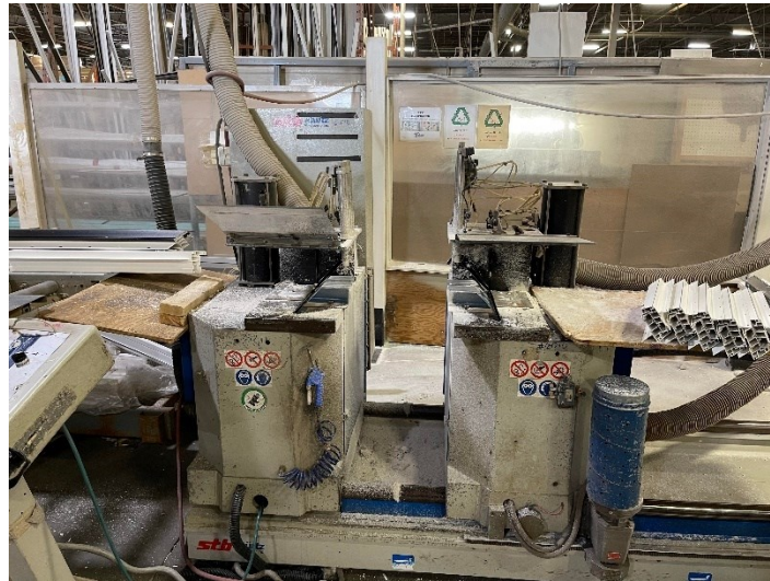
Figure 3.5: Cutting station for A/C windows
