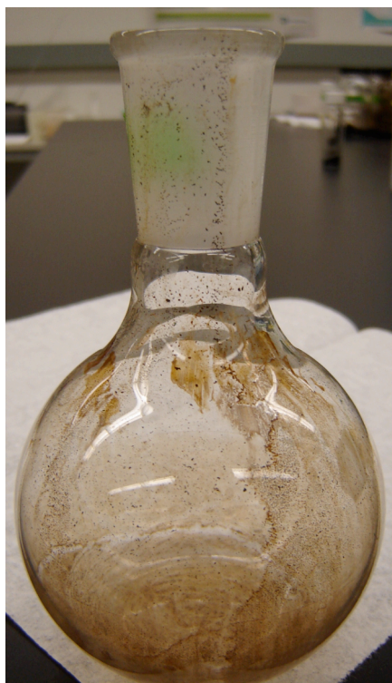
Figure 40. Residual asphaltene particles remaining on the glass wall after decanting with n-pentane.
